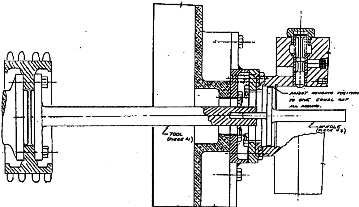
A straightforward method of assuring adequate length tang engagement is to lengthen the tang and slot design to accommodate the range of tolerances. This is the suggested fix.
