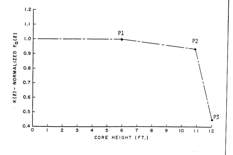
FIGURE TS 3.10-2 HOT CHANNEL FACTOR NORMALIZED OPERATING ENVELOPE
