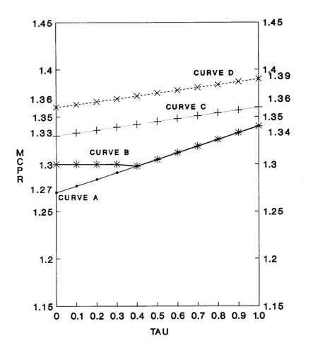
CURVE A - MCPR limit for CCC operational mode with both turbine bypass and moisture separator reheater in service.
