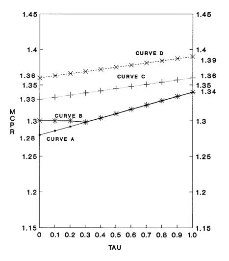
CURVE A - MCPR limit for CCC operational mode with both turbine bypass and moisture separator reheater in service. CURVE B - MCPR limit for non-CCC operational mode with both turbine bypass and moisture separator reheater in service. CURVE C - MCPR limit for both CCC and non-CCC operational modes without either turbine bypass or moisture separator reheater.
