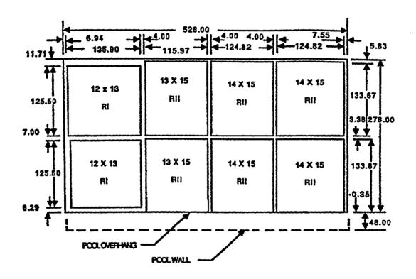
Figure 2-2 SAN ONOFRE UNITS 2 AND 3 REGION I SPENT FUEL STORAGE CELLS
