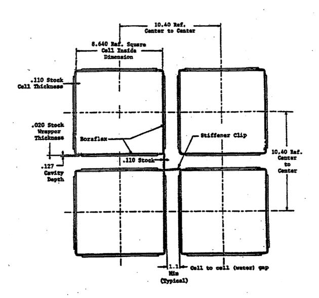
Figure 2-3 SAN ONOFRE UNITS 2 AND 3 REGION II SPENT FUEL STORAGE CELLS
