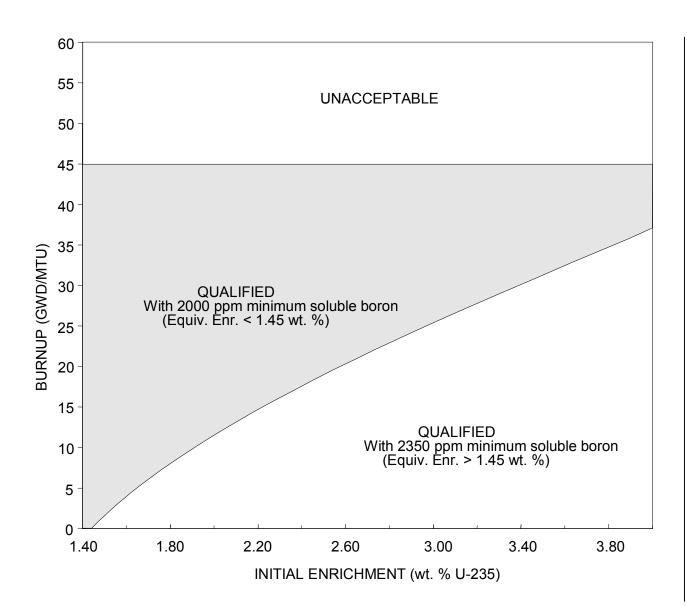
Figure 1-1 PWR Fuel Criticality Acceptance Curve
