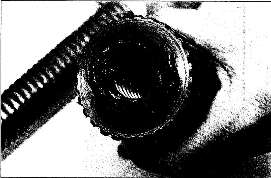
**Figure A-44.** After testing, the EP1 had hardened inside the stem nut.
