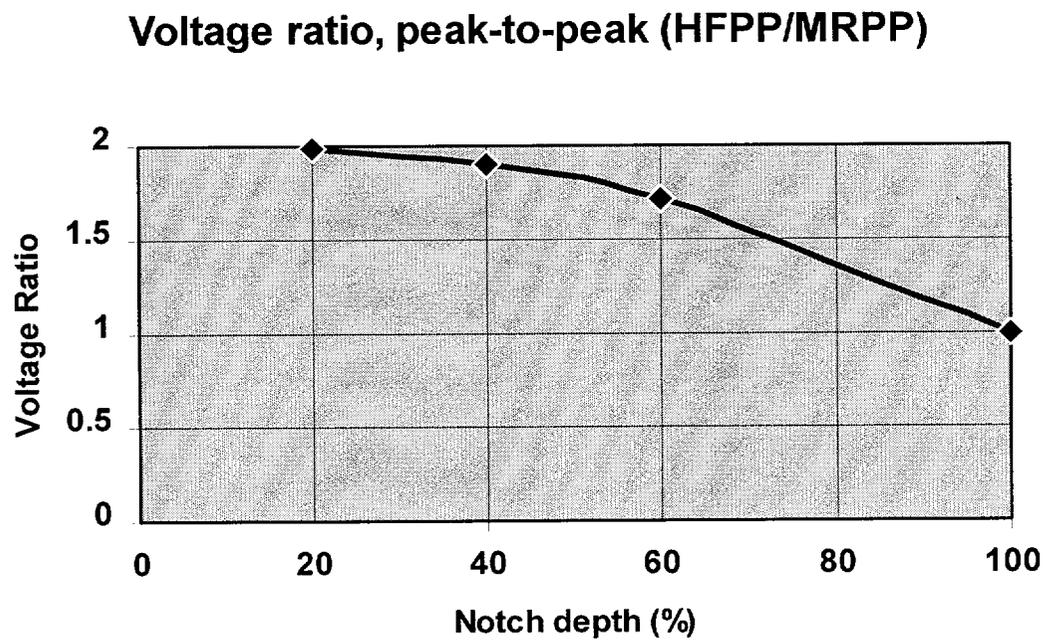
correspond to a defect about 70% deep. This curve is for the peak-to-peak voltage. The voltage measurement ratios for the vertical component of the high-frequency probe are slightly greater, since it has a larger phase angle.
