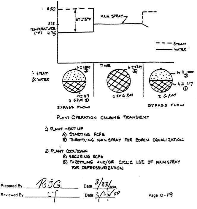
Newly Specified (ABB/CE) Transient <u>B-3</u> Stratified Flow  $\Delta T = 300^{\circ}$ F. Sources: Page E6 of Ref. O-3, and Figure 3.2-3 of Volume 1 of Ref. O-4
