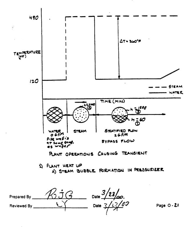
Newly Specified (ABB/CE) Transient <u>B-5</u> Stratified Flow  $\Delta T = 600^{\circ}$ F. Sources: Page E7 of Ref. O-3, and Figure 3.2-5 of Volume 1 of Ref. O-4
