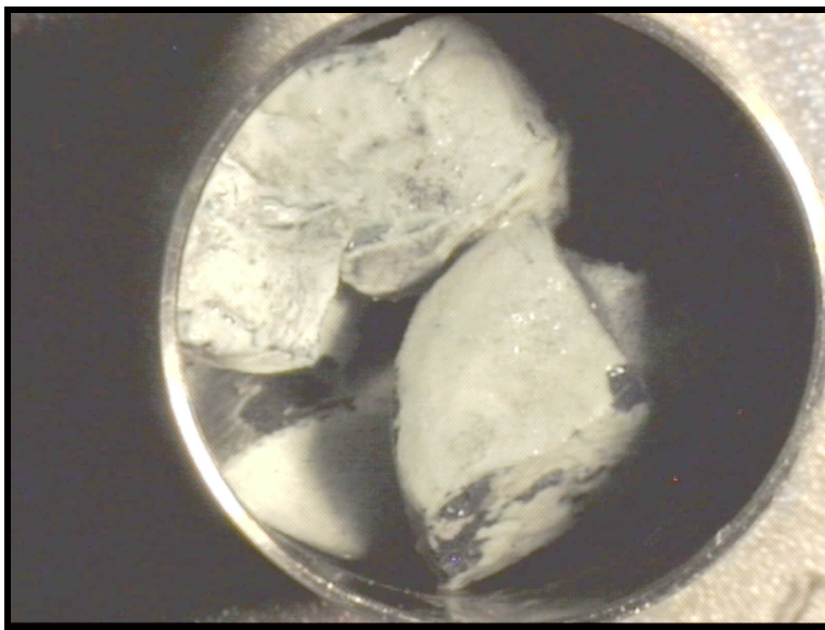
Figure 3. Visual Appearance of Fragments of the ATM-103 Fuel after 8.2 Years of Exposure to Humid Air and Dripping Groundwater
