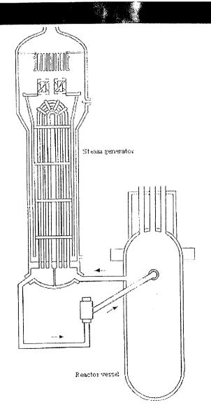
"Steam generators constitute more than 50% of the surface area of the primary pressure boundary in a pressurized water reactor."
