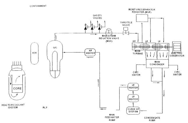
"Unlike other parts of the reactor pressure boundary, the barrier to fission product release provided by the steam generator tubes is not reinforced by the reactor containment as an additional barrier."
