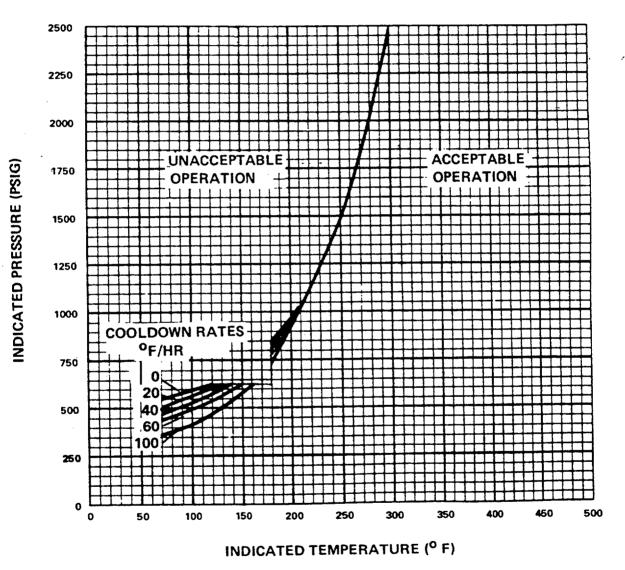
FIGURE 3.4-3 FARLEY UNIT 1 REACTOR COOLANT SYSTEM COOLDOWN LIMITATIONS APPLICABLE FOR THE FIRST 16 EFPY
