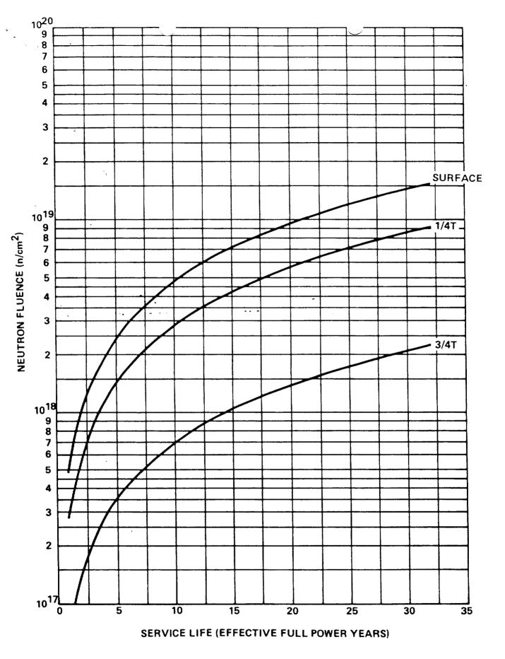
FIGURE B 3/4.4-2 FAST NEUTRON FLUENCE (E>1 MeV) AT 45° AS A FUNCTION OF FULL POWER SERVICE (EFPY)
