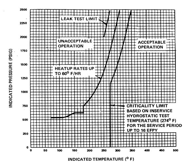
FIGURE 3.4-2 FARLEY UNIT 1 REACTOR COOLANT SYSTEM HEATUP LIMITATIONS APPLICABLE FOR THE FIRST 16 EFPY
