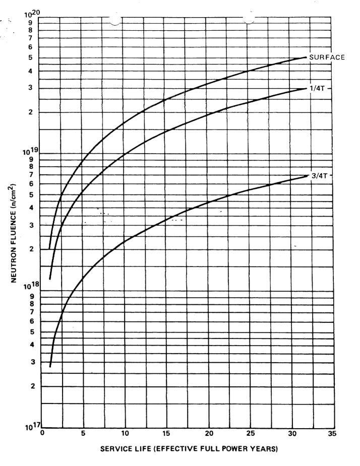
FIGURE B 3/4.4-1 FAST NEUTRON FLUENCE (E>1 MeV) AS A FUNCTION OF FULL POWER SERVICE LIFE (EFPY)
