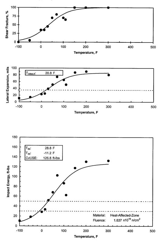
Figure 5-18. Charpy Impact Data for Irradiated Heat-Affected-Zone Material
