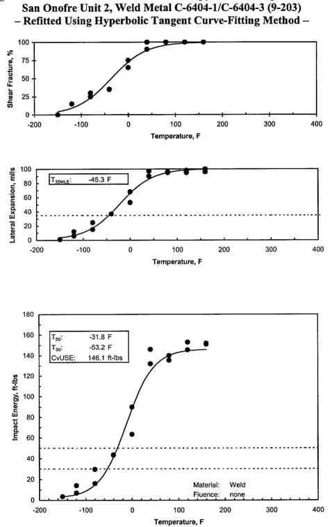
Figure B-5. Unirradiated Surveillance Charpy V-Notch Impact Data for
