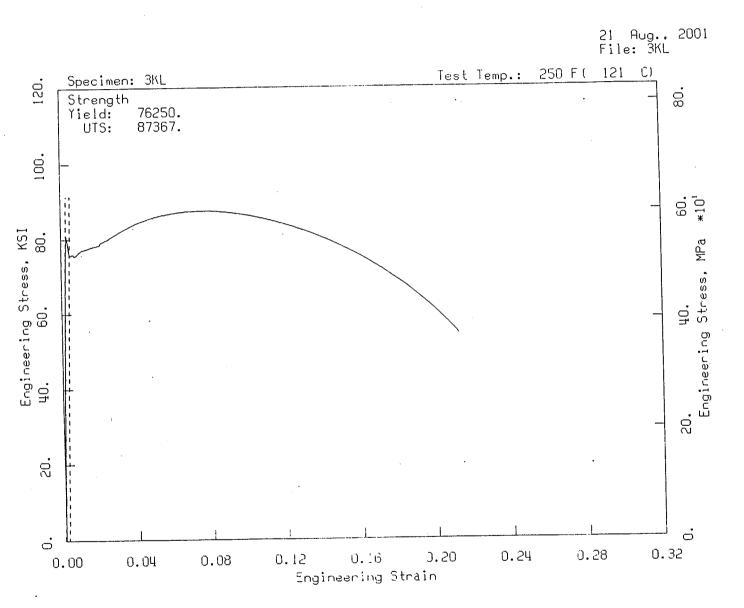
Figure 5-8. Tension Test Stress-Strain Curve for Weld Metal, C-6404-1/C-6404-3 (9-203), Specimen No. 3KL, Tested at 250°F
