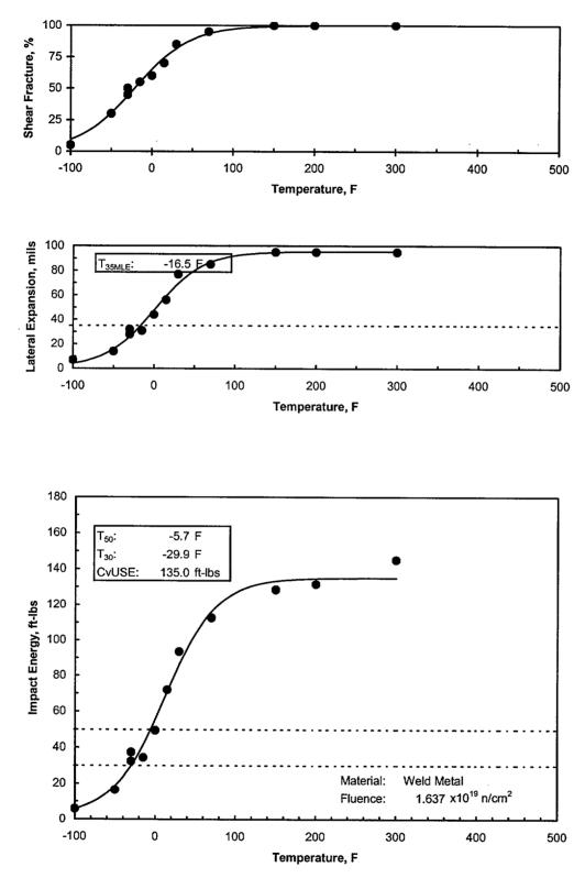
Figure 5-17. Charpy Impact Data for Irradiated Weld Metal, C-6404-1/C-6404-3 (9-203)
