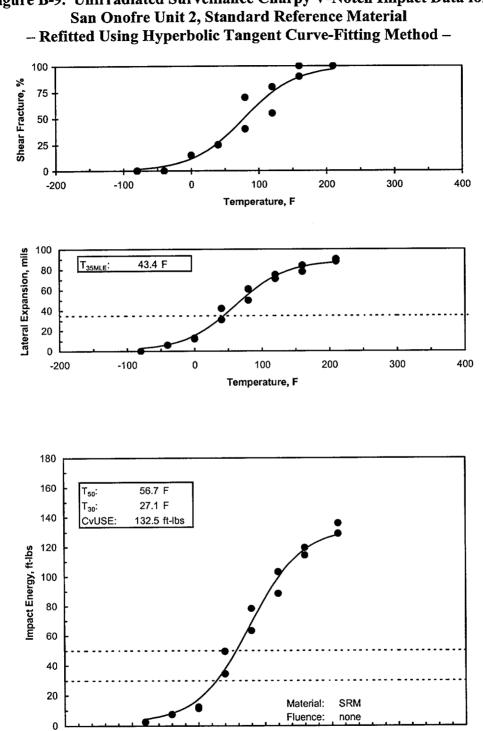
Figure B-9. Unirradiated Surveillance Charpy V-Notch Impact Data for
