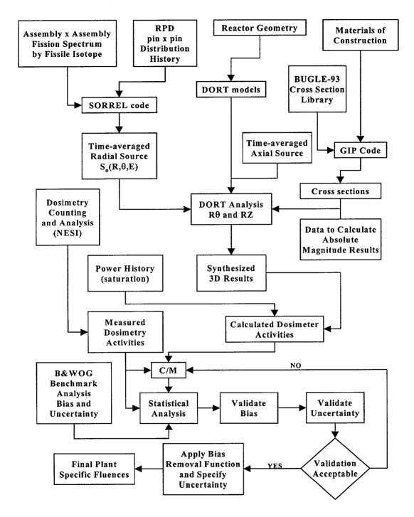
Figure D-1. Fluence Analysis Methodology for San Onofre Unit 2 Surveillance Capsule
