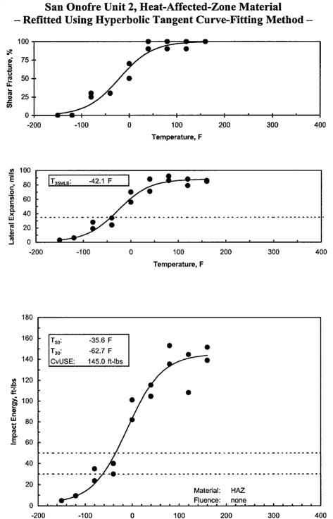
Figure B-7. Unirradiated Surveillance Charpy V-Notch Impact Data for San Onofre Unit 2, Heat-Affected-Zone Material
