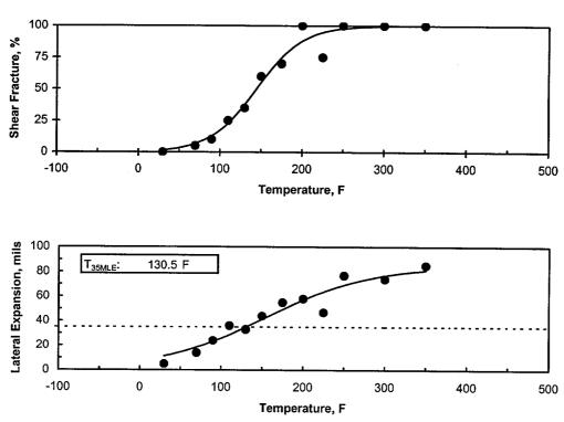
Figure 5-16. Charpy Impact Data for Irradiated Base Metal Plate C-6404-2, Transverse Orientation
