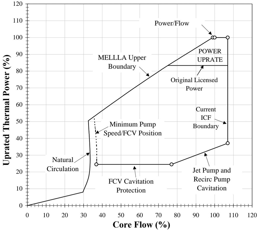
Figure 1-1. Typical CPPU-Based Power Uprate Power/Flow Map
