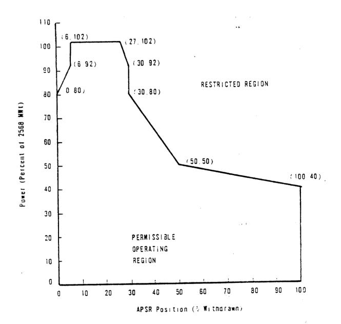
APSR POSITION LIMITS FOR OPERATION FROM 150 ± 10 EFPD TO 390 + 10 EFPD Unit 2 - 30 OCONEE NUCLEAR STATION Figure 3.5.2-482
