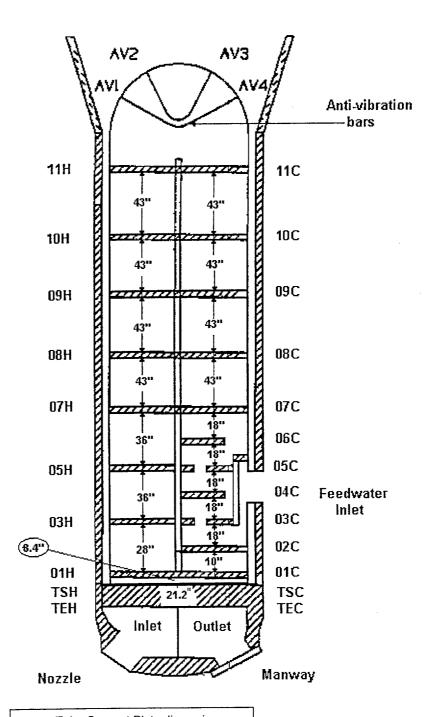
**Note:** Tube Support Plate dimensions are from centerline to centerline.
