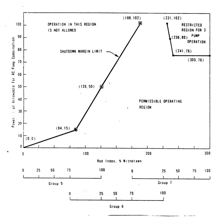
ROD POSITION LIMITS FOR TWO-AND THREE-PUMP OPERATION FROM 100  $(\pm 10)$  TO 235  $(\pm 10)$ , EFPD UNIT 1
