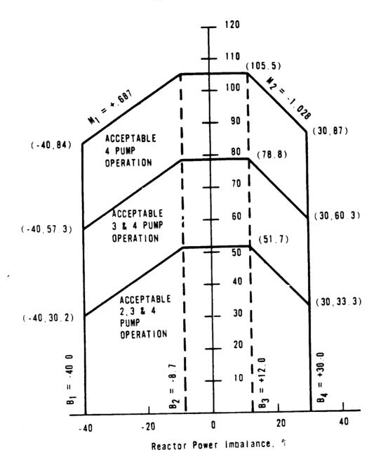
PROTECTIVE SYSTEM MAXIMUM ALLOWABLE SETPOINTS UNIT 1 OCONEE NUCLEAR STATION Figure 2.3-2A
