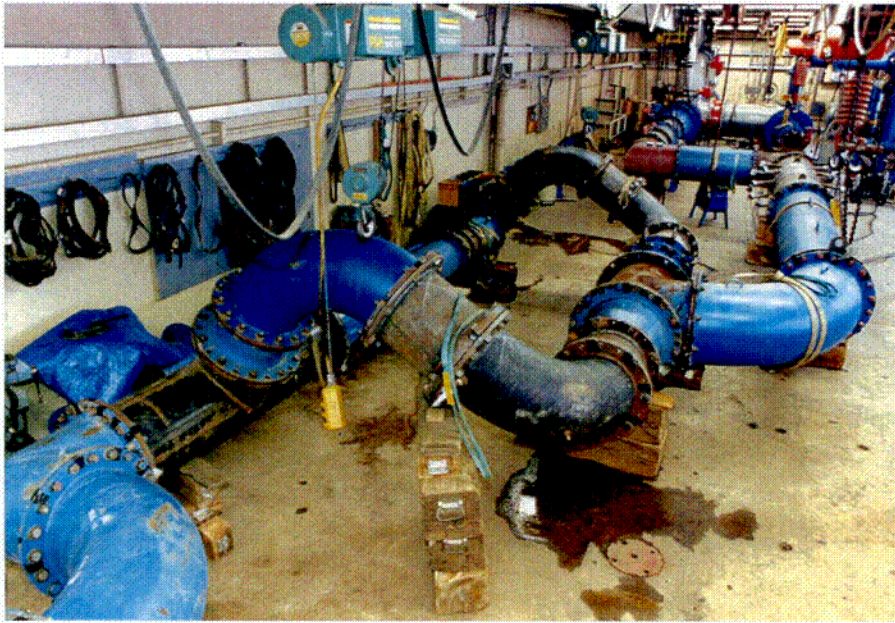
Figure 5: Calibration Test of an LEFM CheckPlus Spool (Looking Downstream)
