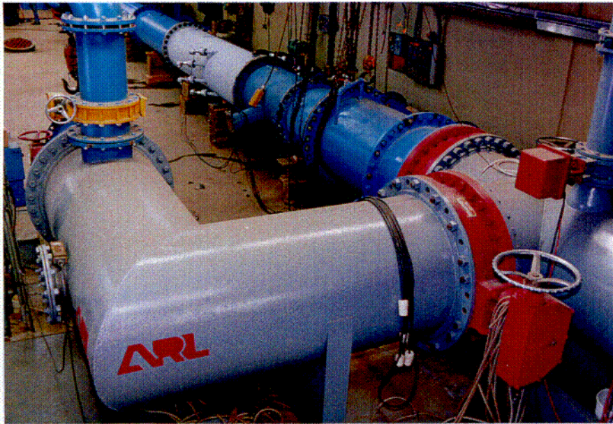
Figure 4: Calibration Test of an LEFM Check Spool (Looking Upstream)
