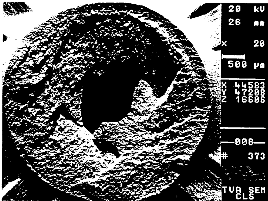
SEM photographs of typical fracture surfaces taken from fractures screws (set "A"). Note that all fractured screws received in set "A" failed in a brittle manner (except for the small final fracture area near the center which failed in a ductile manner). 20X.
