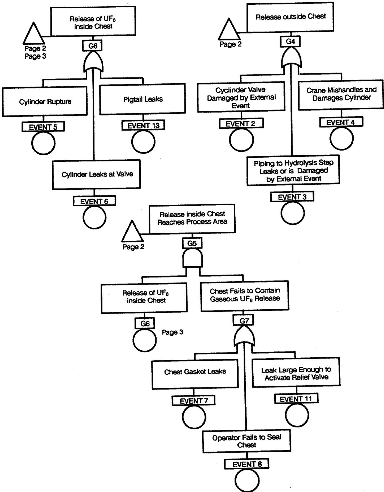
Fault Tree for Release of UF<sub>6</sub> During Vaporization (Cont.)
