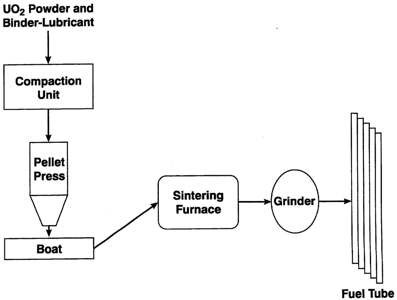
**Figure B.1. Uranium Fuel Fabrication**
