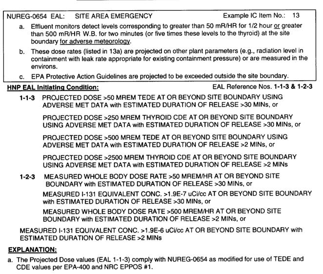
b. The measured values (EAL 1-2-3) are consistent with the recommendations stated in the NUREG.
