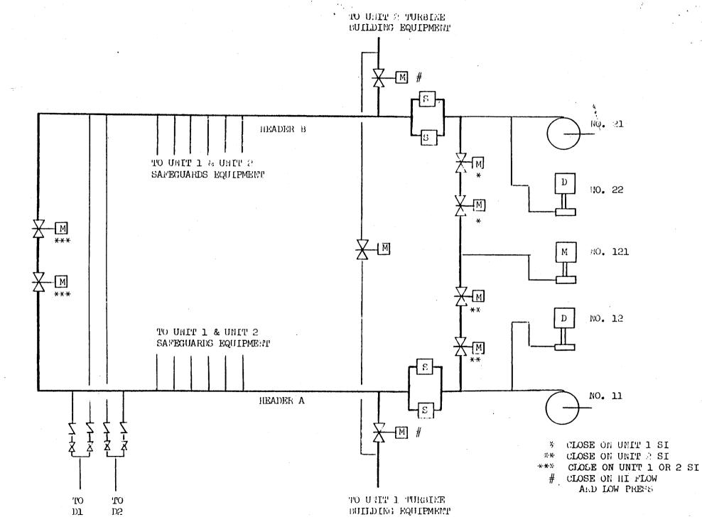
Figure 1. Simplified flow diagram of Cooling Water Supply Hender.
