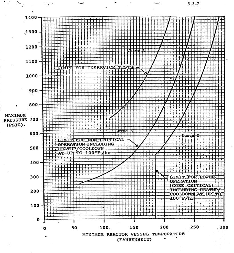
OYSTER CREEK NUCLEAR GENERATING STATION REACTOR VESSEL PRESSURE/TEMPERATURE LIMITS
