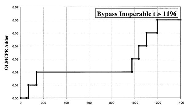
Bypass Valve Delay Time Relative to Time of TSV Full Closure (msec)
