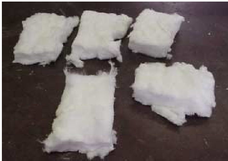
Photo A-11. Kaowool insulation cut into 4-in. x 6-in. pieces.
