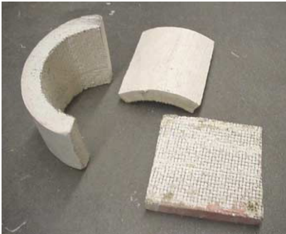
Photo A-4. Marinite fire-barrier material (dry and soaked block).
