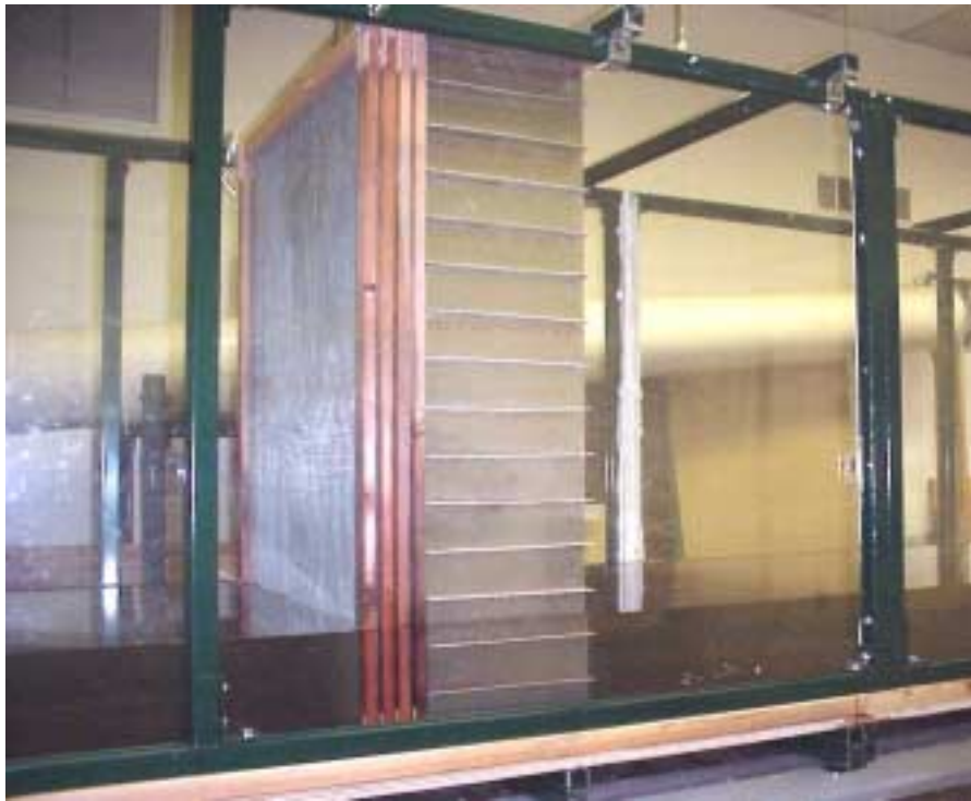
Photo 2. Diffuse flow entry flow conditioning section.
