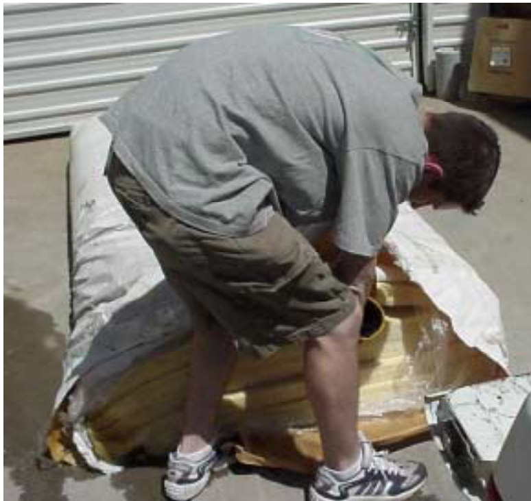
Photo A-9. Thermal-wrap fiberglass insulation in bulk form.
