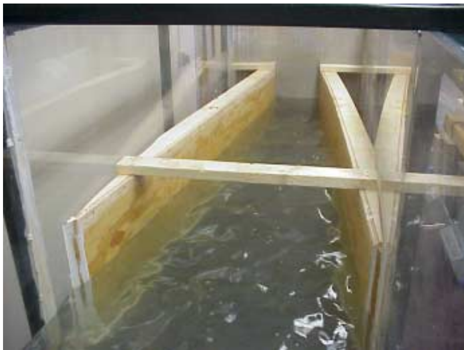
Photo 4. Converging test section.
