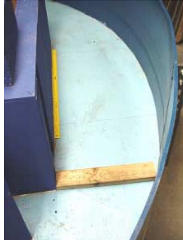
2x4 Barrier to Redirect Debris
