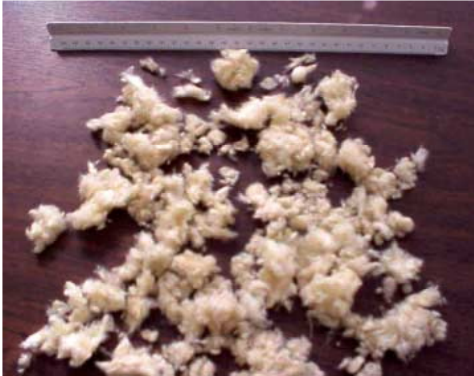
Photo A-8. Typical NUKON fiberglass insulation.
