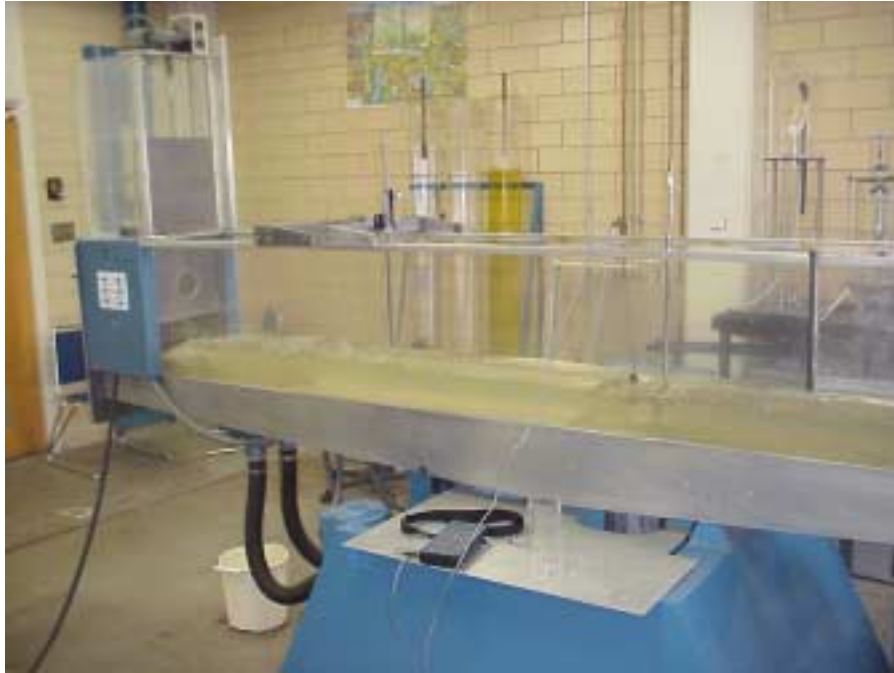
Photo 5. Small flume test apparatus.
