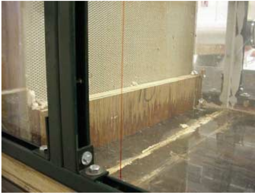
Photo 3. Test obstruction curb (6-in.) and debris catch screen.
