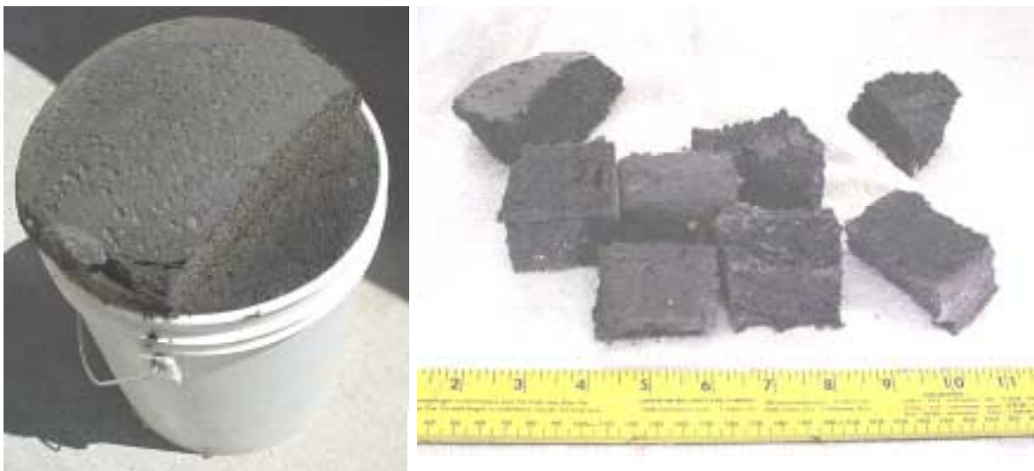
Photo A-6. Silicone foam insulation material (as foamed and pieces tested).
