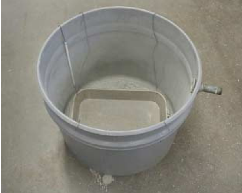
Photo 7. Plastic cylinder used in dissolution tests.
