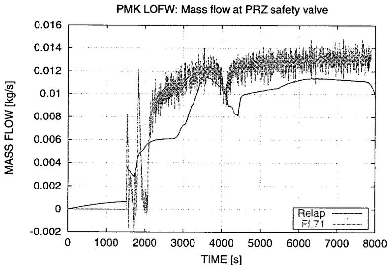
Figure 13: Mass flow rate at PRZ safety valve
