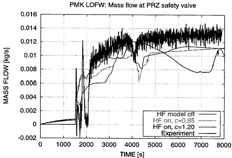
Figure 20: Mass flow rate in PRZ safety valve
