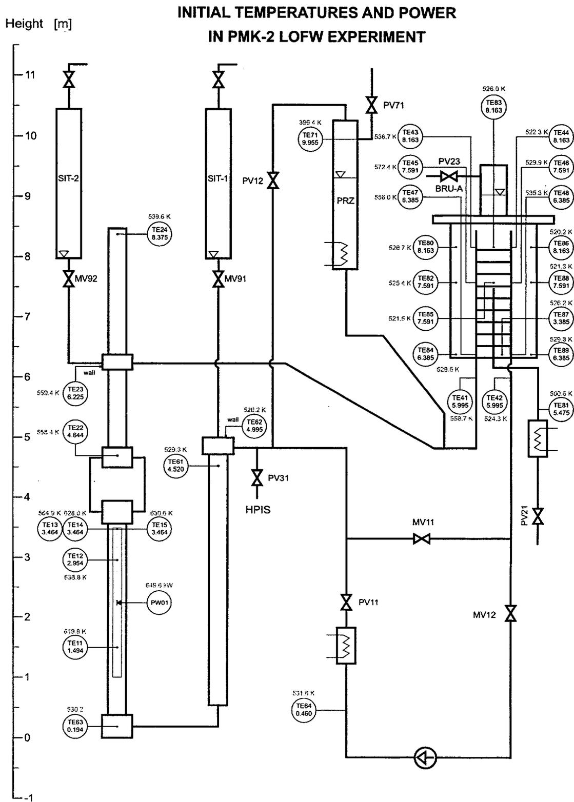
Figure 4: Initial temperatures and the heating power
