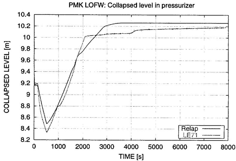
Figure 12: Collapsed level in the PRZ
