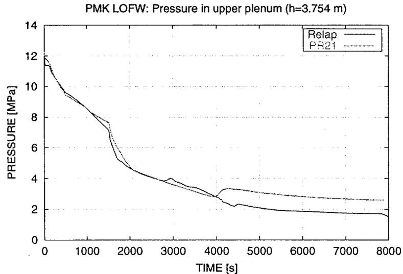
Figure 11: Pressures in the upper plenum
