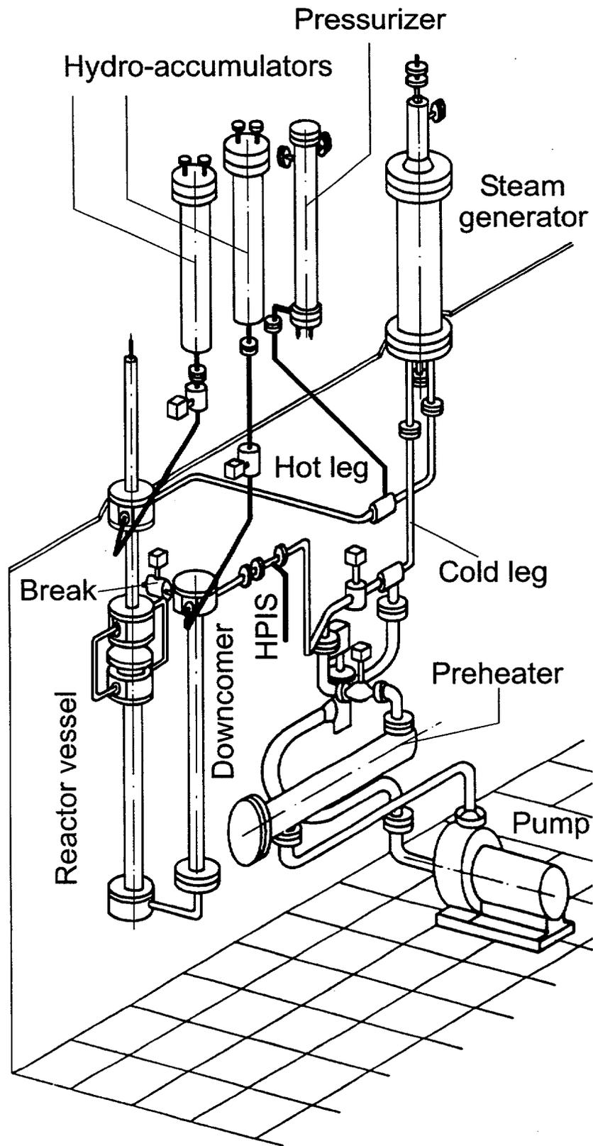
Figure 1: Axonometric view of the PMK-2 facility
