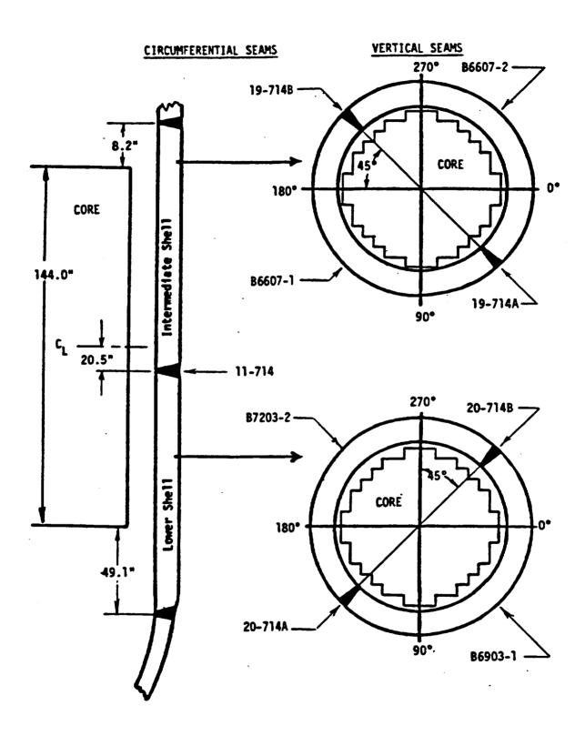
Figure 1: Identification and Location of Beltline Region Materials for the Beaver Valley Unit 1 Reactor Vessel
