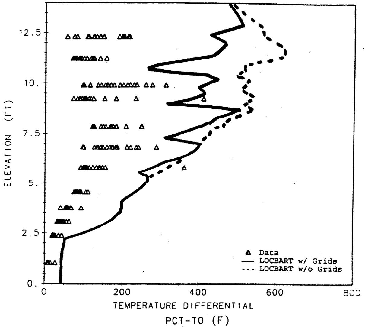
Figure 102. Maximum Clad Temperature Rise (PCT-T0) Versus Elevation for G2 562.
