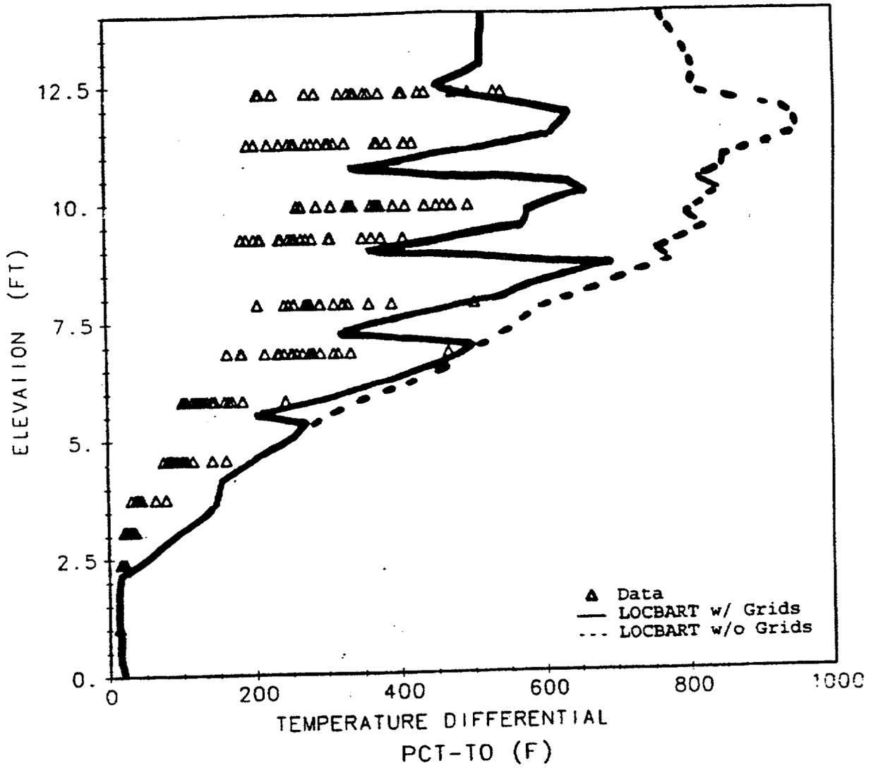
Figure 111. Maximum Clad Temperature Rise (PCT-T0) Versus Elevation for G2 564.
