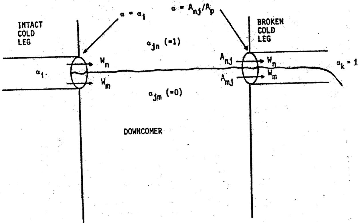
Figure 3-15. Flow Links Connecting Volume Pairs
