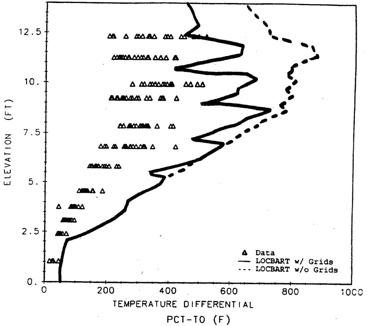
Figure 120. Maximum Clad Temperature Rise (PCT-T0) Versus Elevation for G2 568.
