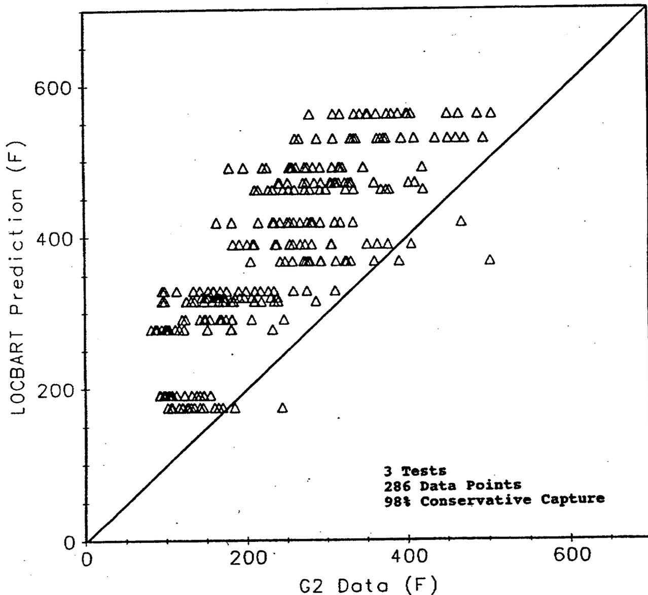
Figure 129. G2 Experiments Data Versus LOCBArt Model Clad Temperature Rise Adjusted for [ ]<sub>a,c</sub>
