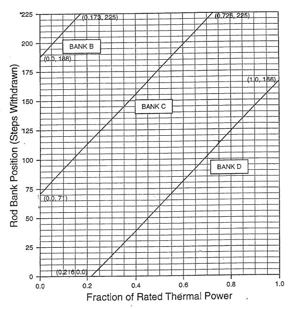
Bank A must be fully withdrawn prior to power operation.
