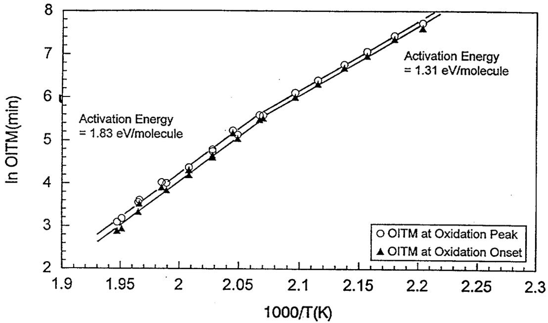
Figure 3.44 Arrhenius plot for white XLPE insulation
