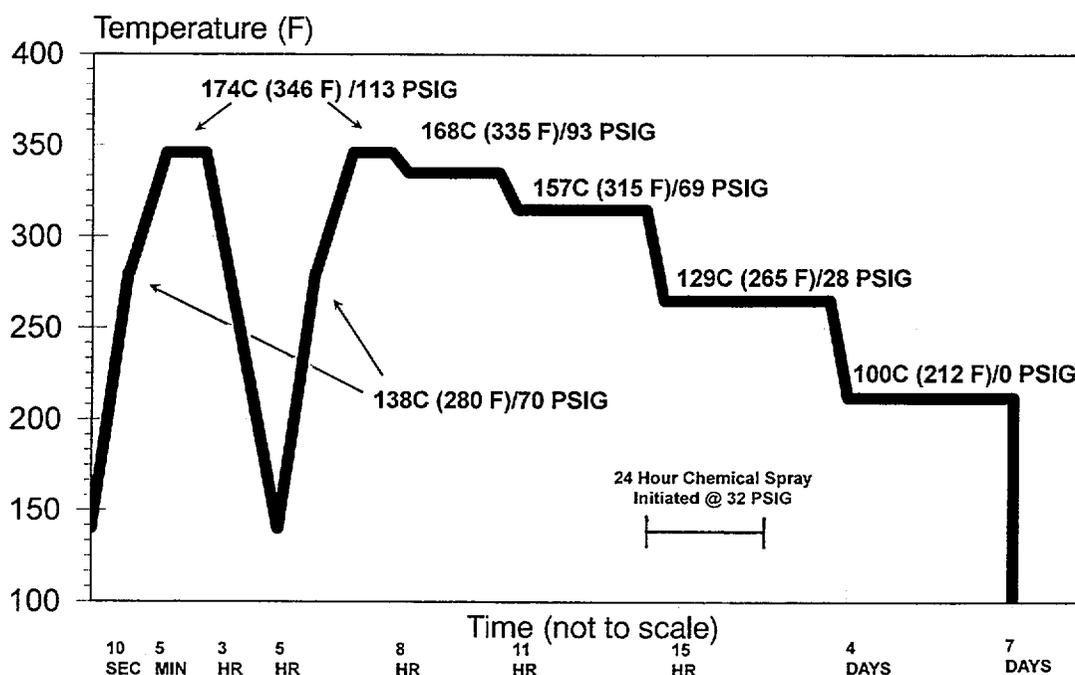
**Figure 3.3 Test chamber temperature/pressure profile used in LOCA Tests 1, 3, 4, 5 and 6**
