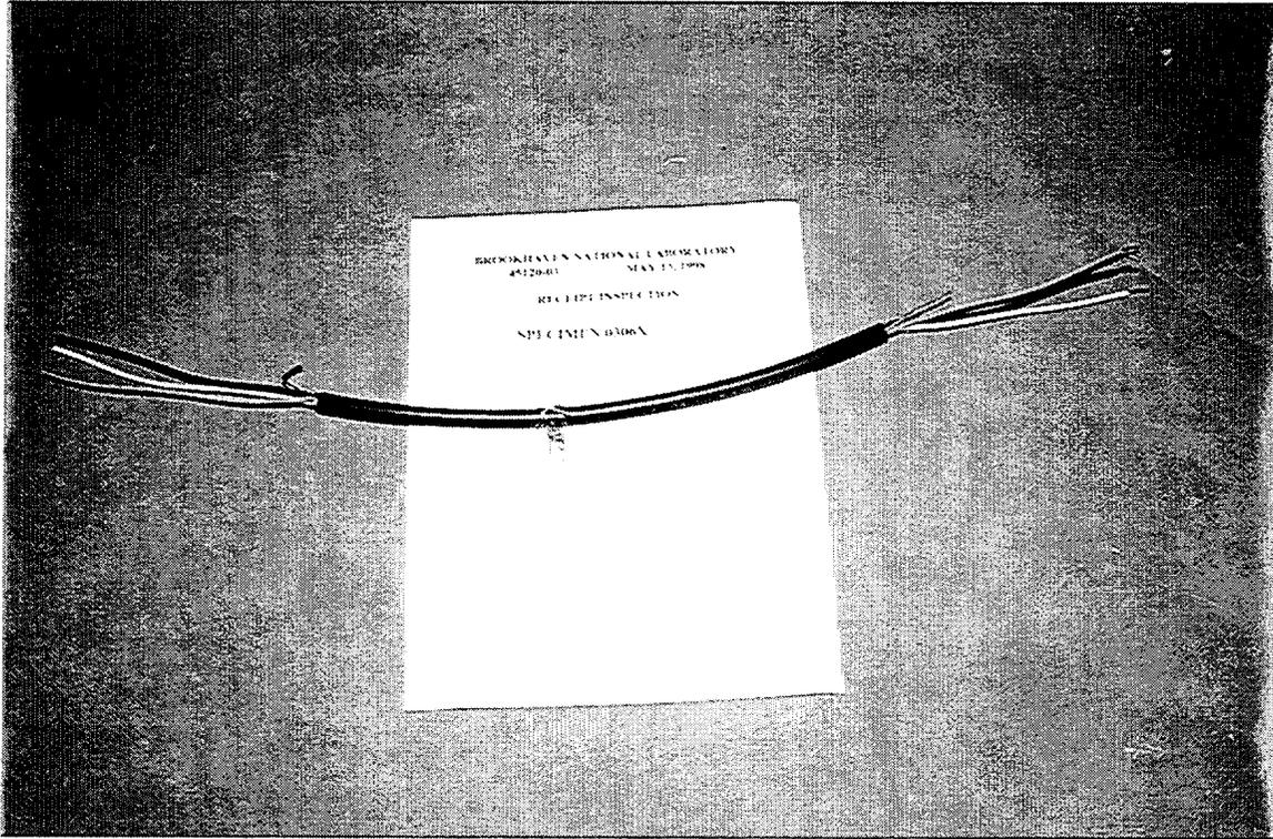
Figure 2.6 Typical 2-foot specimen for indenter testing
