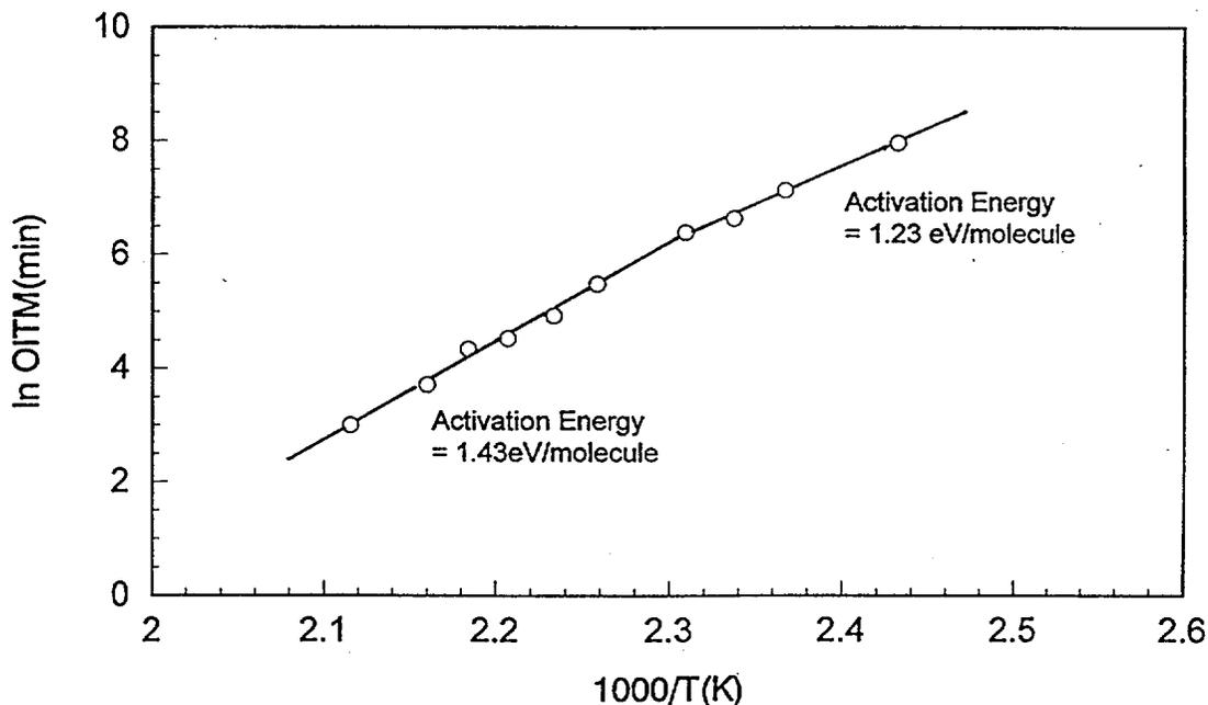
Figure 3.45 Arrhenius plot for EPR insulation
