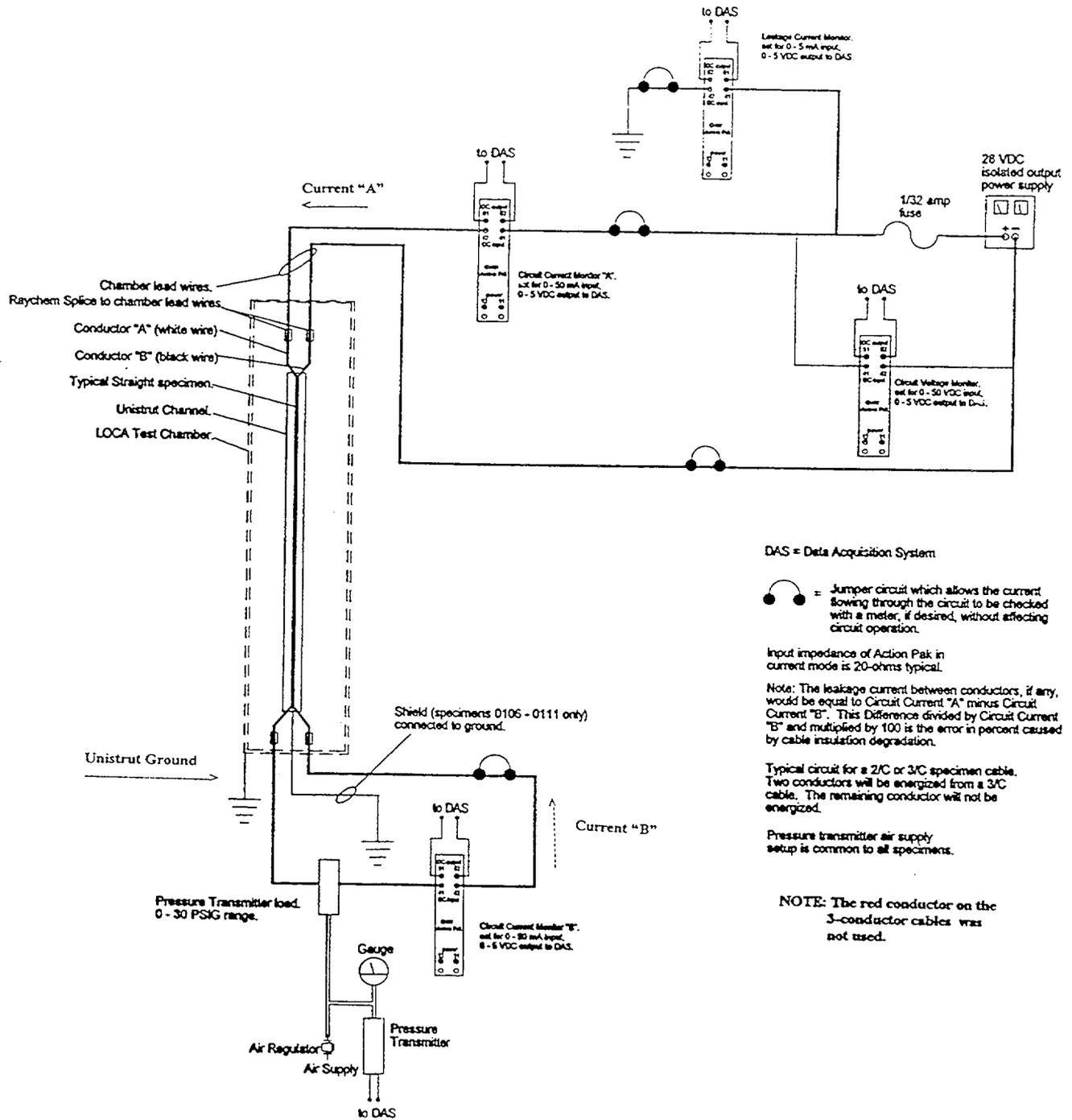
Figure 2.13 Monitoring circuit diagram for straight Unistrut<sup>®</sup> mounted specimens
