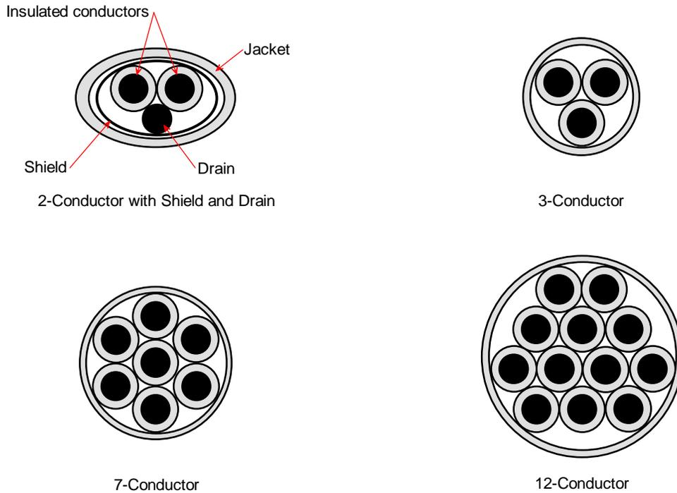
Figure 2-1. Illustration of common multi-conductor cable arrangements.
