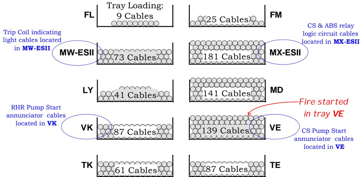
Figure C-9. Cable tray locations and contents. (Ref: Exhibit C1, pp. 30-32 of 69, *Physical Damage to Electric Cables and Raceways Involved in the Browns Ferry Nuclear Plant Fire on March 22, 1975*, contained in Regulatory Investigation Report Office of Inspection and Enforcement Region II.)
