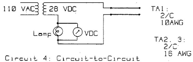
Circuit 4: Circuit-to-Circuit
