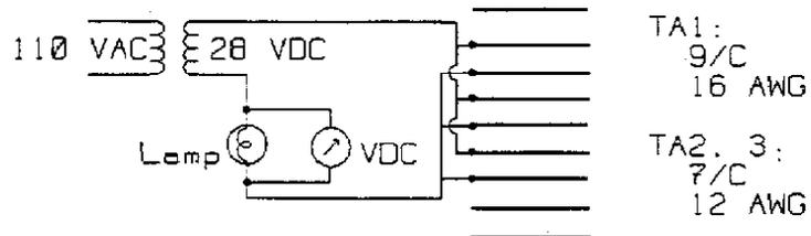
Circuit 3: Circuit-to-Circuit
