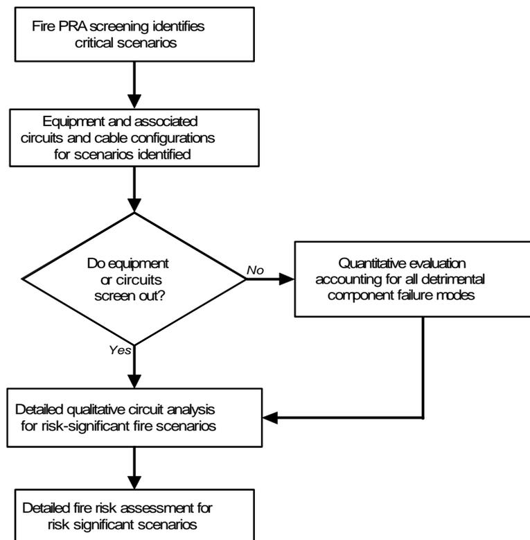
Figure 4-1. Circuit analysis process for fire risk assessment.
