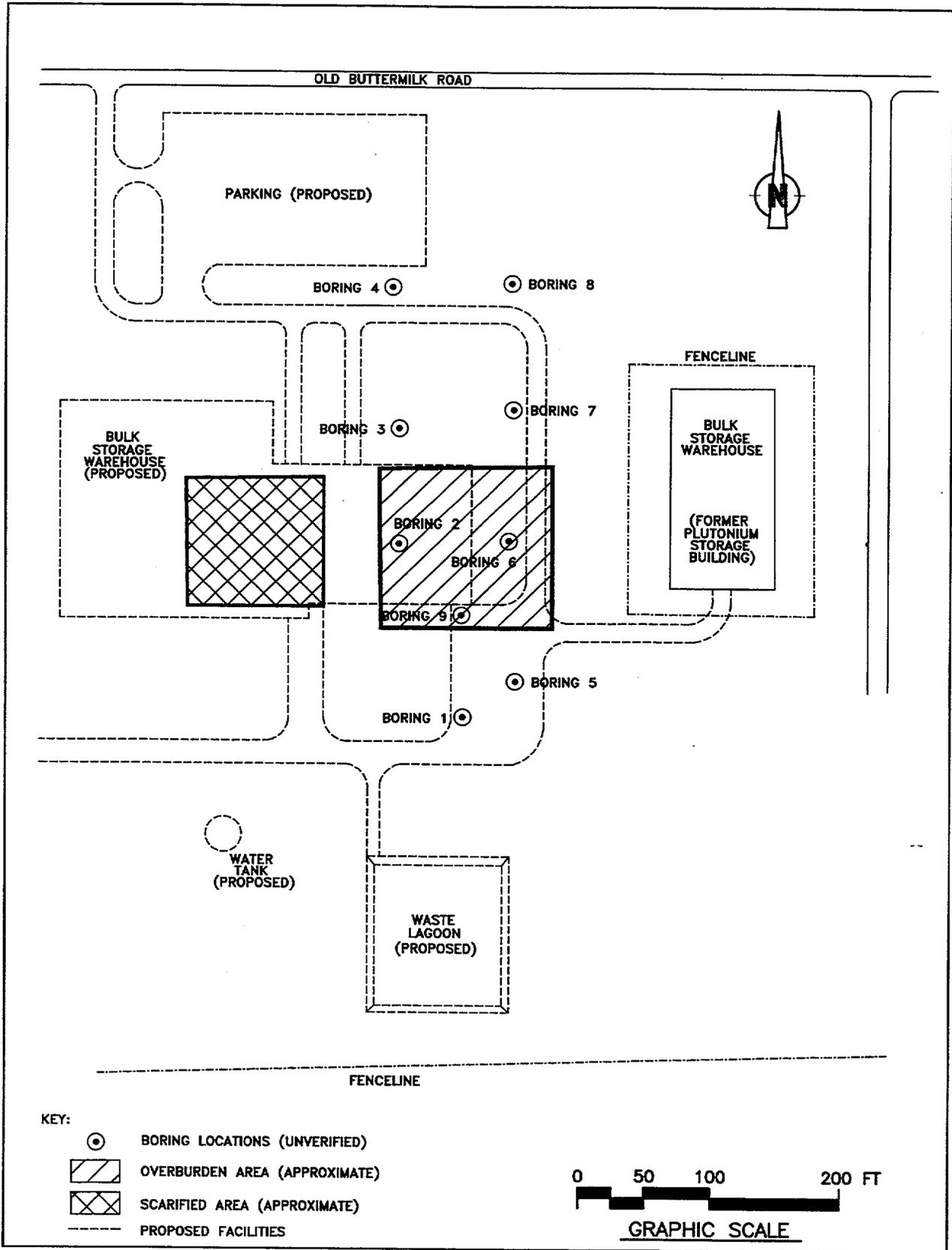
Figure A.3.6-16b Locations of Boreholes Indicated in FIGURE A.3.6-16a
