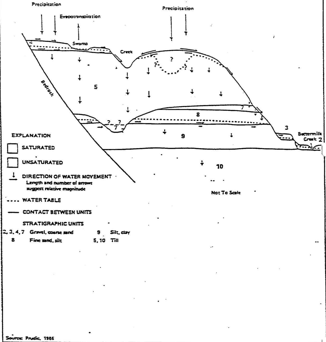
FIGURE A.3.5-11 Inferred Distribution of Saturated and Unsaturated Conditions in the South Plateau Subsurface (Idealized Cross Section)
