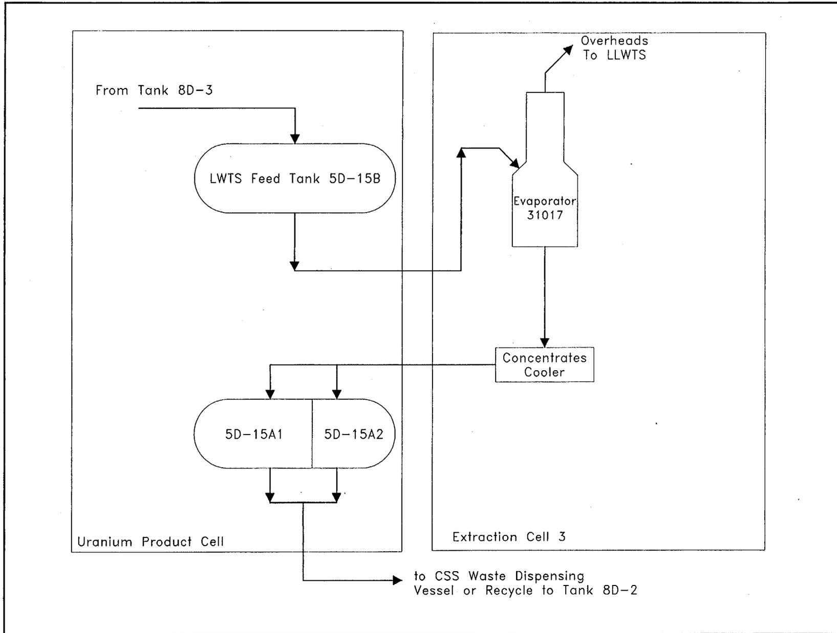
Figure A.1.3-3 Liquid Waste Treatment System Process Flow Diagram.
