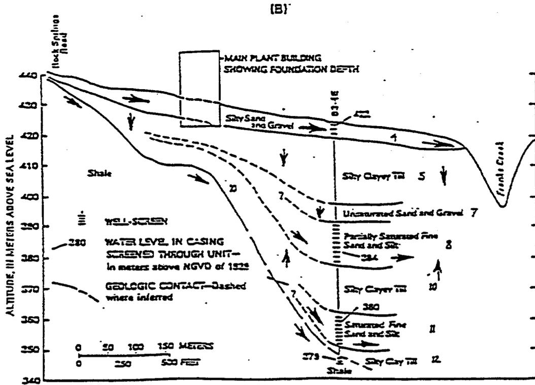
SCHMATIZED GROUNDWATER FLOW PATTERNS BENEATH THE SOUTHERN (A) AND NORTHERN (B) SECTORS OF THE WVDP
