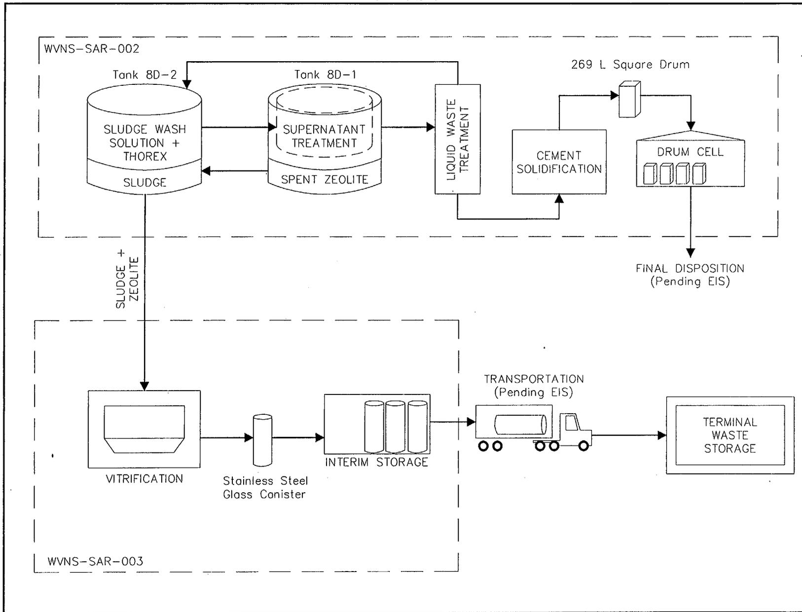
Figure A.1.3-1 Waste Processing Flow Diagram
