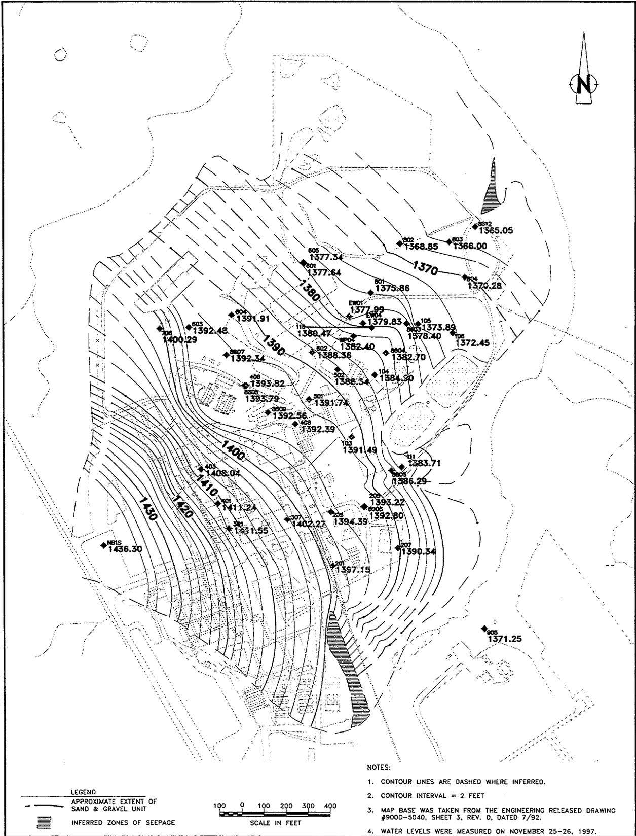
Figure A.3.5-4 Unconfined Groundwater Flow Within the Surficial Sand and Gravel Layer – North Plateau
