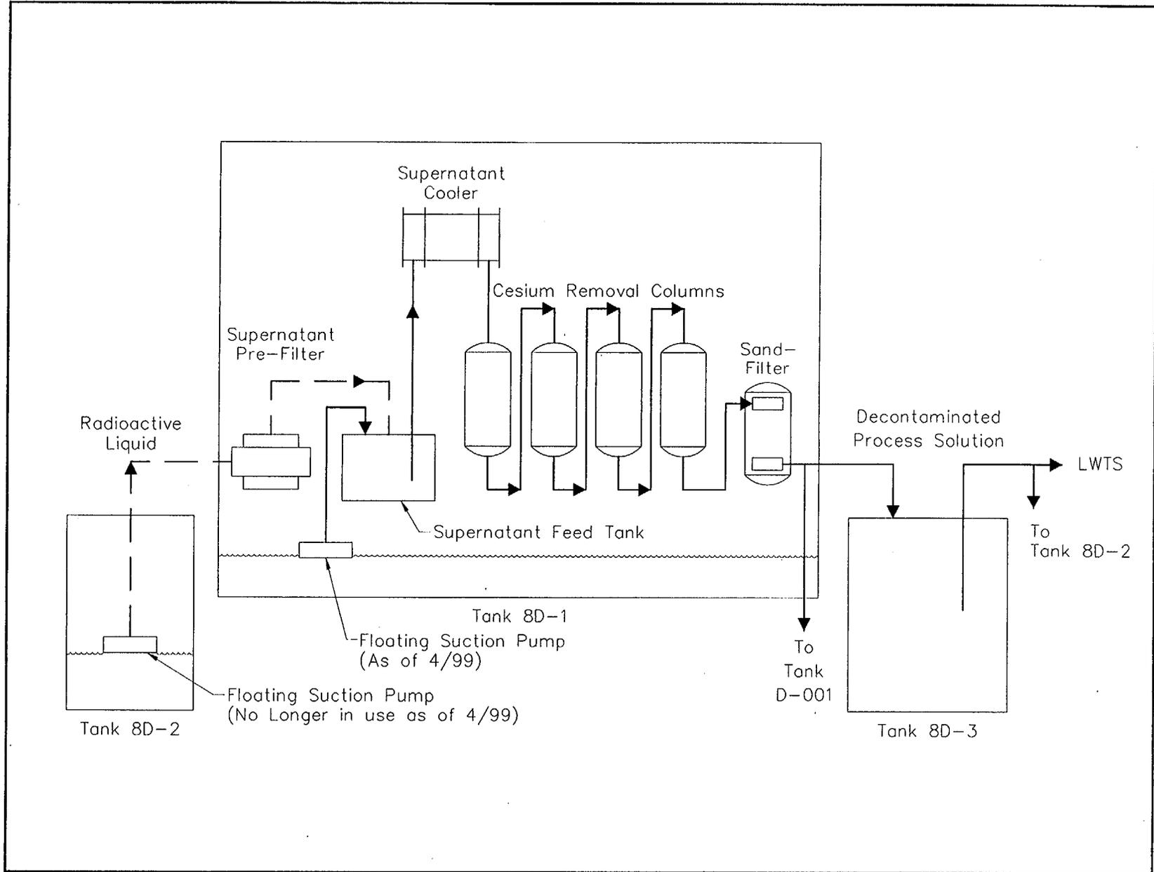
Figure A.1.3-2 Supernatant Treatment System Process Flow Diagram.
