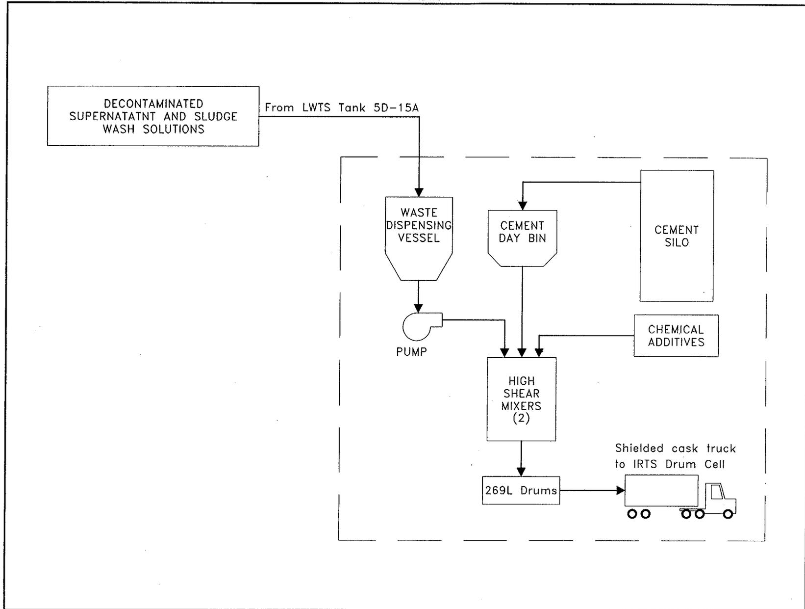
Figure A.1.3-4 Cement Solidification System Process Flow Diagram.
