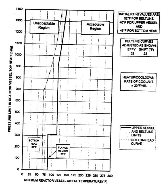
P-T Curve for Hydrostatic or Leak Testing
