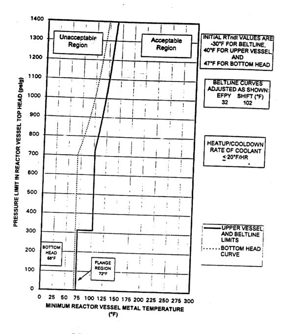
P-T Curve for Hydrostatic or Leak Testing
