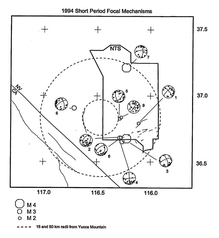
Figure 12. Lower hemisphere projections of reliably determined short period p-wave first motion focal mechanisms in the SGB druing 1994. See Table 3 for event desciptions and location information.
