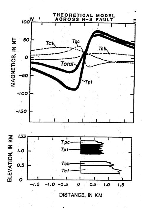
Figure 5. Theoretical magnetic anomaly from vertical offset of north-south trending fault (from Bath and Jahren, 1984). Geologic units and their modeled properties are described in tables 1 and 2, respectively.
