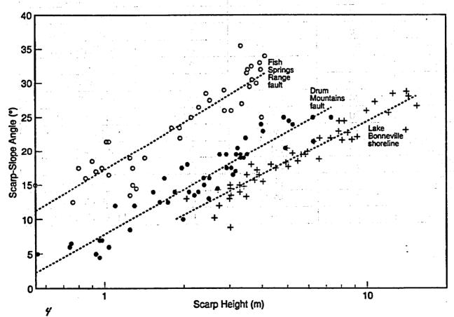
FIGURE 8. Scarp-slope angle versus log scarp-height data for single-event scarps in western Utah. The figure illustrates the resolution and variability of scarp-morphology data. Dotted lines are linear regressions to each of the sets of data. Open circles, fault scarp of Fish Springs Range (about 2 ka; Bucknam and others, 1989); solid circles, fault scarp of Drum Mountains (about 10 ka; Crone, 1983); crosses, shoreline scarp of Lake Bonneville (about 15 ka; Machette, 1989).
