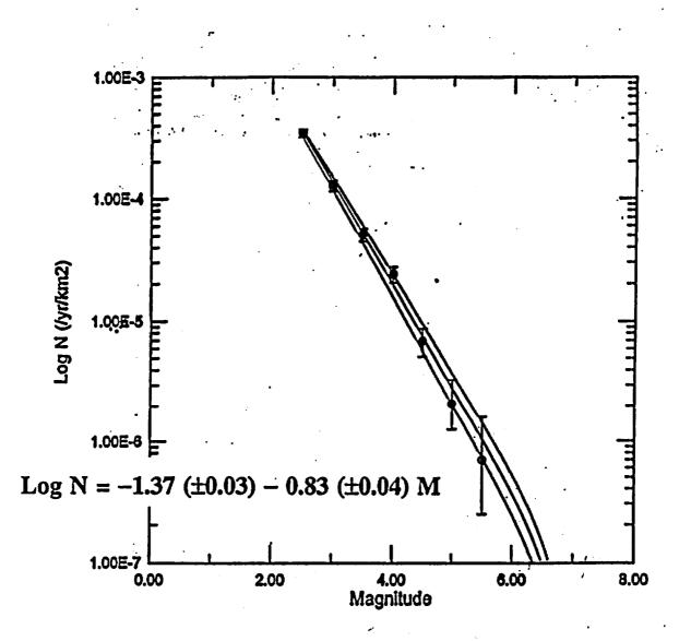
Example of recurrence modeling of seismicity within an areal source zone using the Gutenberg-Richter truncated exponential model and methodology described by Weichert (1980) [from 1994 report for Exploratory Studies Facility at Yucca Mountain].
