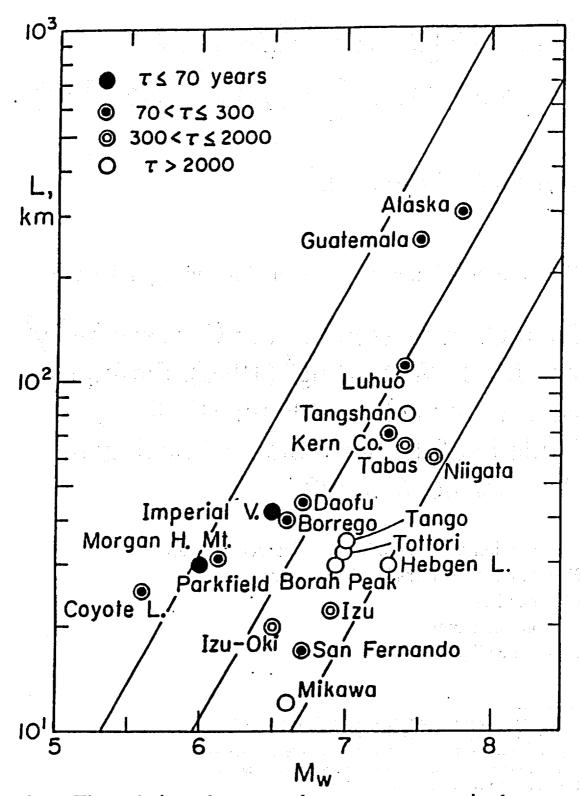
Fig. 2. The relations between the moment magnitude,  $M_W$ , and the fault length, L. The solid lines indicate the trend for a constant stress drop.
