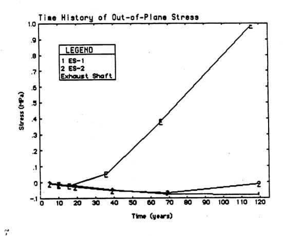
Figure 6. Time History of Induced Out-of-Plane Horizontal Stresses at the Shaft Locations, Computed Using the Boundary Element Models
