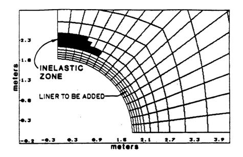
a) Extent of inelastic behavior after relaxation of 85% of in situ stress ( $\sigma_{\rm H}$  horizontal,  $\sigma_{\rm h}$  vertical on diagram)
