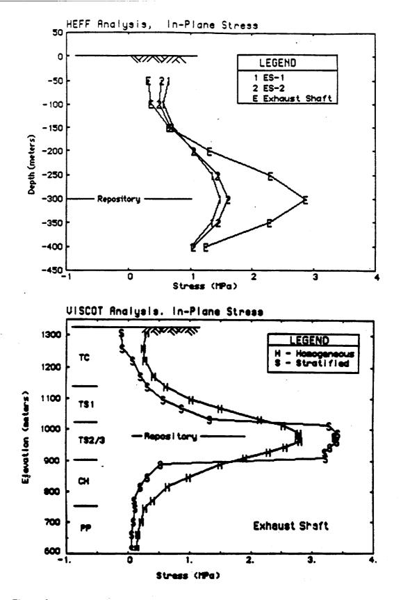
Figure 3. Profile of Induced In-Plane Horizontal Stresses at Selected Shaft Locations, 100 Years After Waste Emplacement
