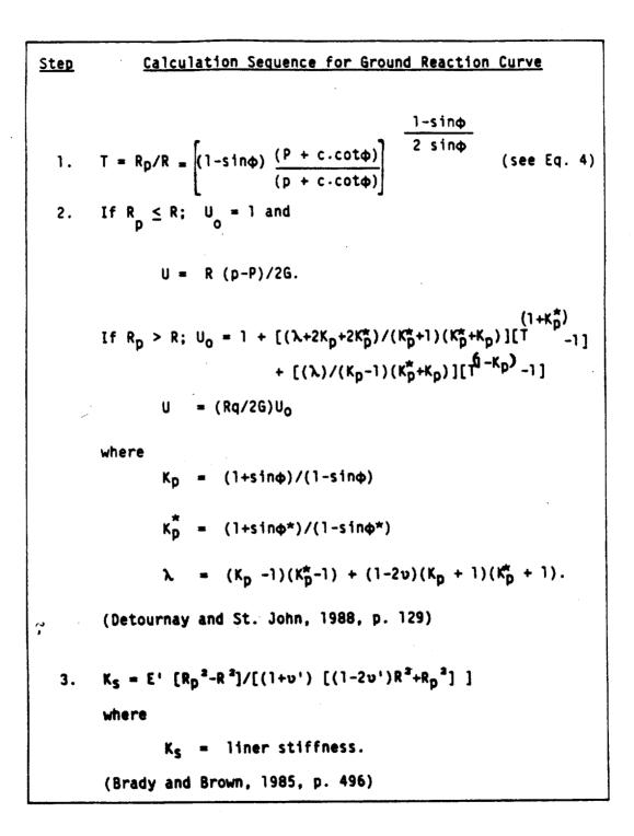
Figure 4-2. Calculation Sequence for Preparing Ground Reaction Curves Using a Dilational Mohr-Coulomb Model
