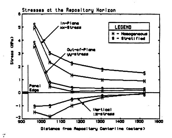
Figure 9. Induced Stress as a Function of Distance, 100 Years After Waste Emplacement, as Computed by the Finite-Element Model
