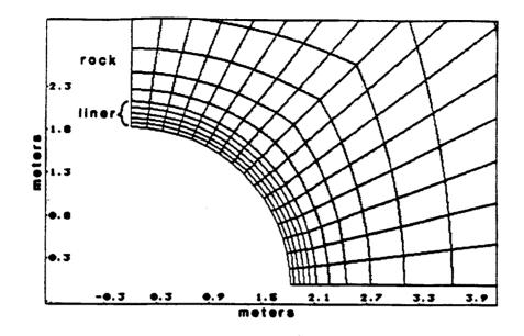
a) Details of the Finite-Element Mesh for the Lined Shaft Model
