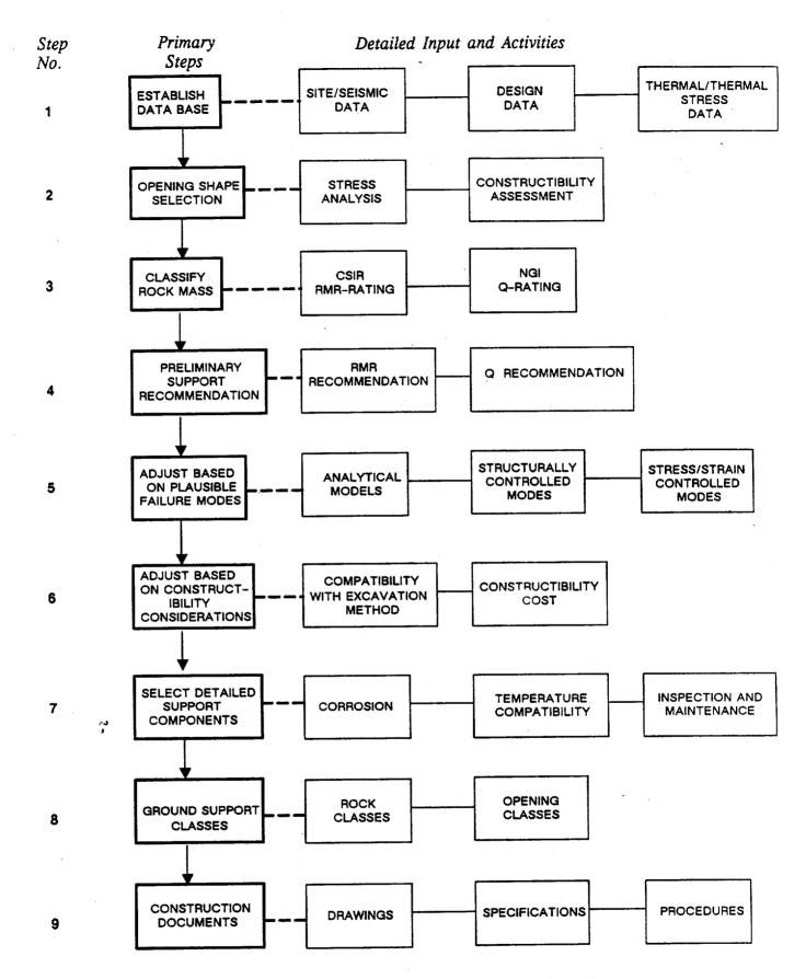
Figure 1. Design Steps for Underground Openings
