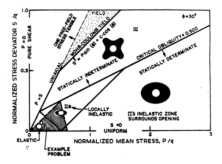
Figure 3-2. Relationship Between the Initial Horizontal Stress State and Failure Modes for an Unlined Shaft in a Mohr-Coulomb Elastic-Plastic Medium, for  $\Phi = 30^{\circ}$  (after St. John et al., 1984). (Shaded area represents the approximate zone of interest for example problem: note very limited inelastic behavior.)
