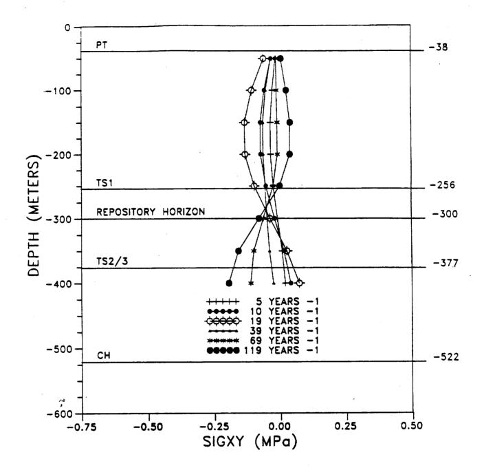
Figure 11. Induced Shear Stress Versus Depth at the ES1 Shaft Location, Computed Using the Boundary Element Model
