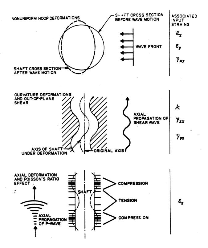
Figure 4-5. Schematic Diagram of Possible Deformation Modes Resulting from Seismic Wave Action (After Owen and Scholl, 1981)
