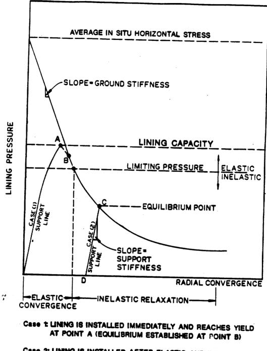
Case 2: LINING IS INSTALLED AFTER ELASTIC AND INELASTIC CONVERGENCE (D) OCCURS (EQUILIBRIUM ESTABLISHED AT POINT C)
