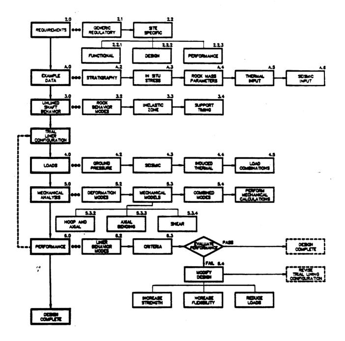
Figure 1-3. Flow Chart of Liner Design Methodology (numbered boxes refer to report sections)
