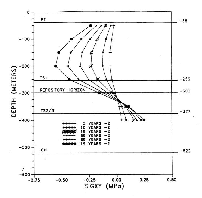
Figure 12. Induced Shear Stress Versus Depth at the ES2 Shaft Location, Computed Using the Boundary Element Model
