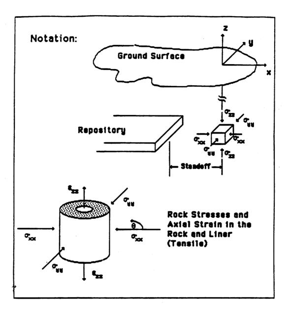
Figure 2. Notation for Repository and Shaft Analysis
