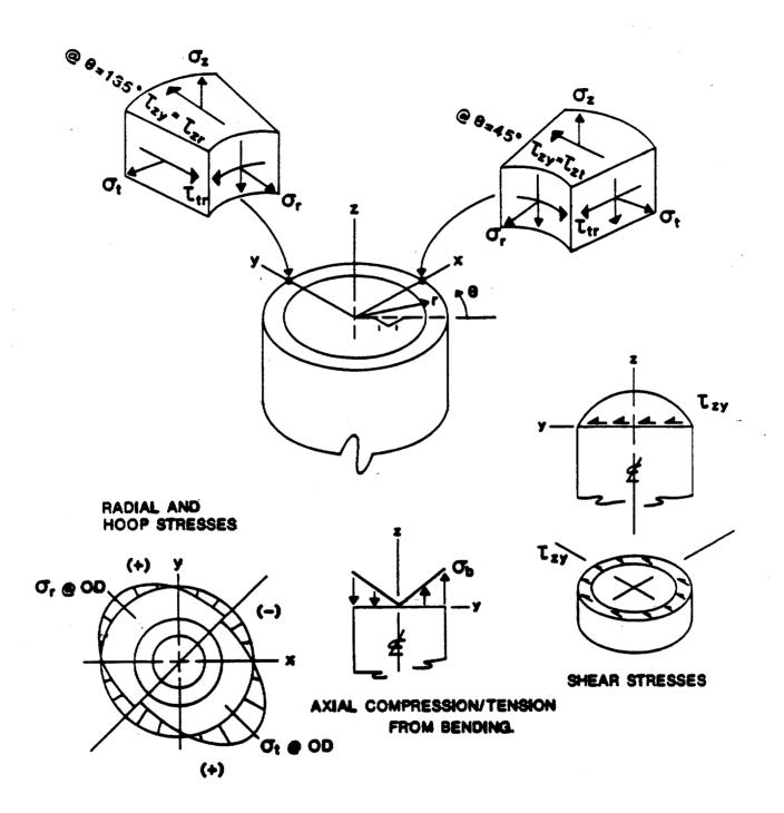
Figure 5-5. Typical Stresses due to Inclined S<sub>H</sub> Wave (After Fluor/PB-KBB, 1987)
