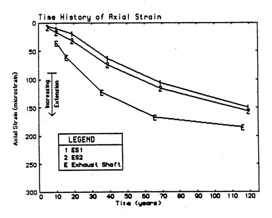
Figure 8. Time History of Induced Axial Strain at the Shaft Locations, Computed Using the Boundary Element Models
