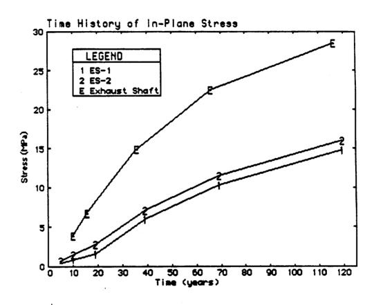
Figure 7. Time History of Induced In-Plane Horizontal Stresses at the Shaft Locations, Computed Using the Boundary Element Models
