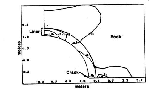
b) Fully Cracked Liner
