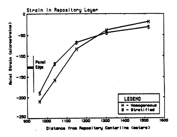
Figure 10. Induced Axial Strain as a Function of Distance, 100 Years After Waste Emplacement, as Computed by the Finite-Element Model
