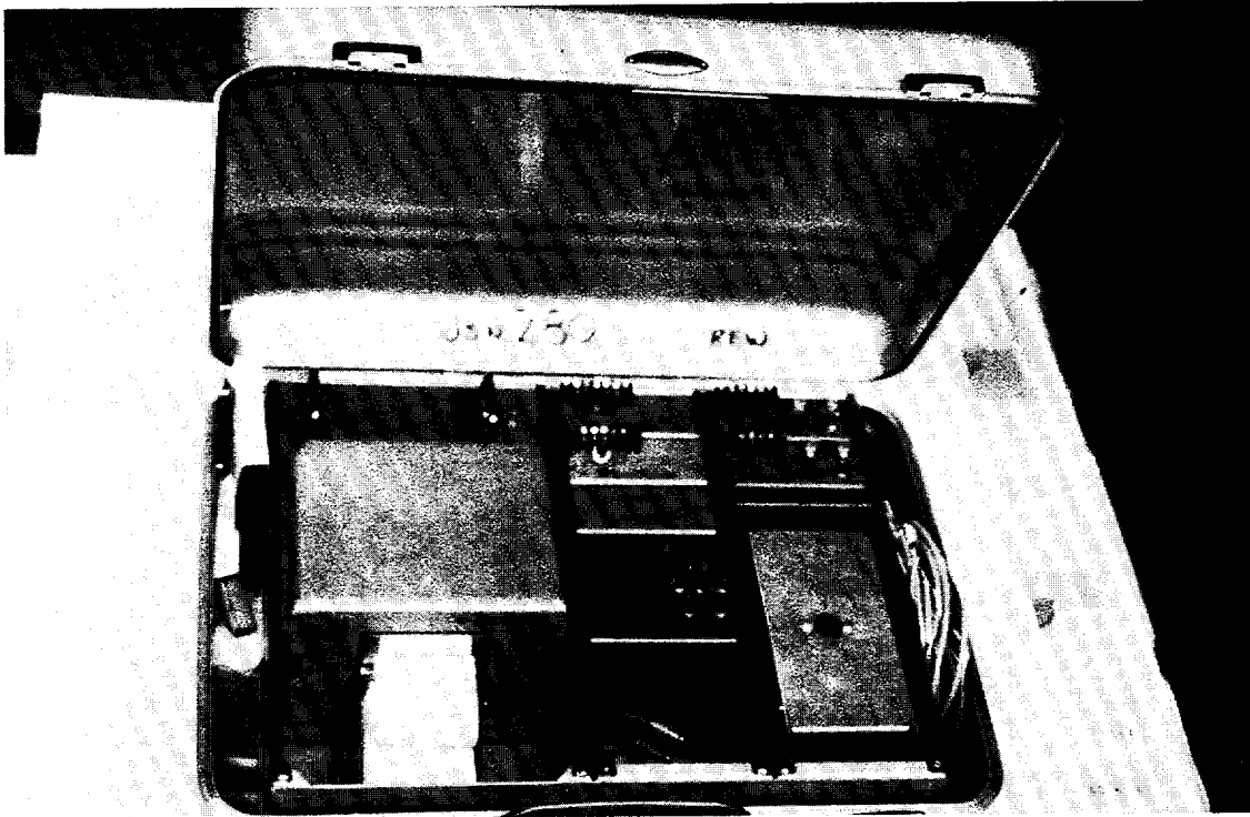
Figure 21.--Example of a solid-state datalogger.
