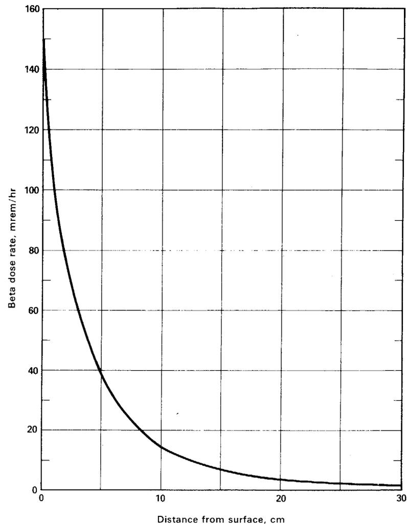
**FIGURE 2. BETA DOSE RATE FROM YELLOWCAKE SEPARATED FROM ORE FOR MORE THAN 100 DAYS (from Reference 13)**
