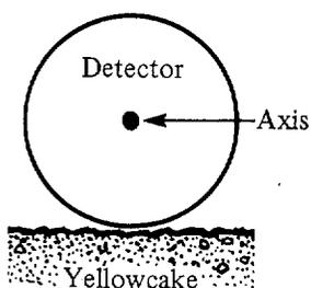
At 2 cm: Place the axis of the detector at 2 cm from the surface of the yellowcake. The closed-window reading is 3 mR/hr. The open-window reading is 23 mR/hr. The difference is 20 mR/hr. Since the beta dose rate at 2 cm is 75 mrem/hr, the calibration factor  $CF_{2\text{cm}}$  can be calculated:
