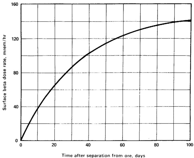
**FIGURE 1. BETA DOSE RATE ON THE SURFACE OF YELLOWCAKE**
