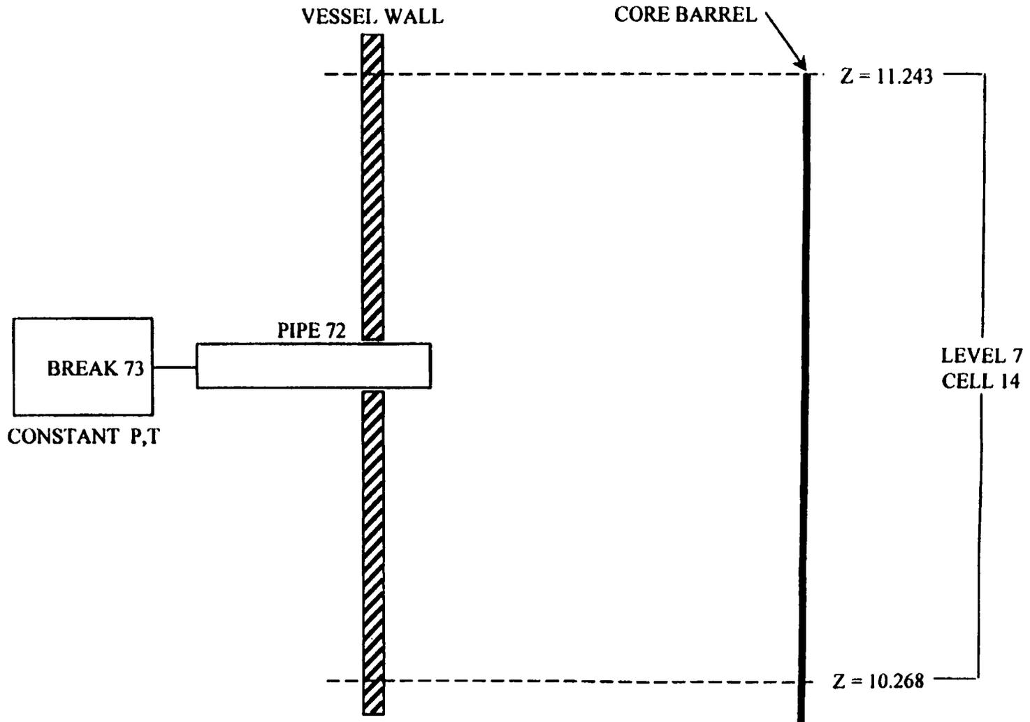
Figure 3: Break Nodalization
