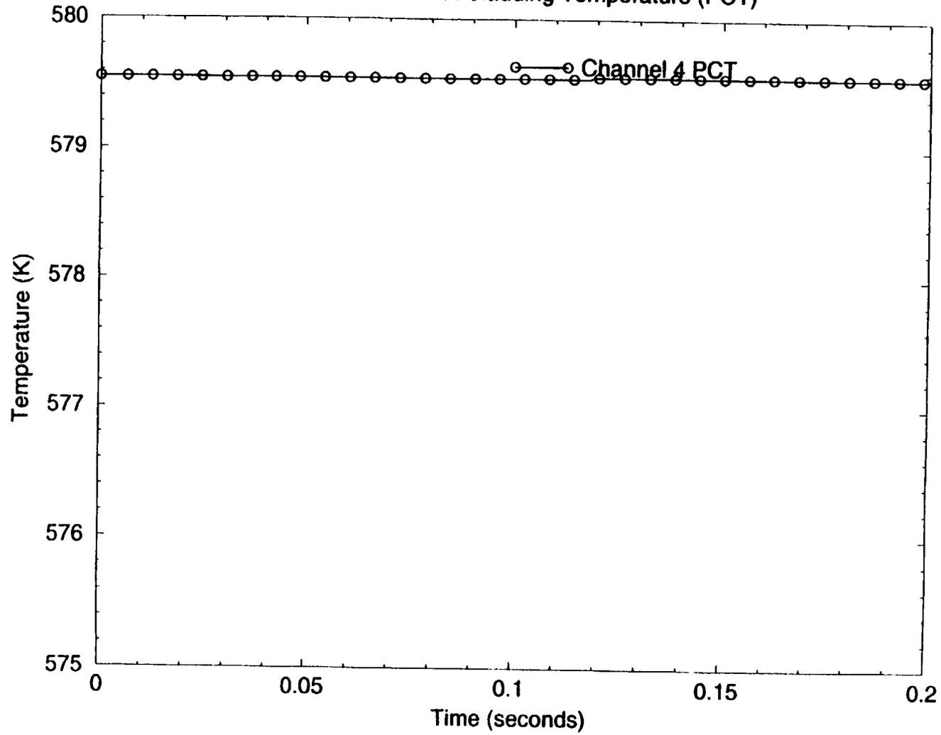
Figure 35: Peak Cladding Temperature for Hot Channel Component 4 (0-0.2 sec)
