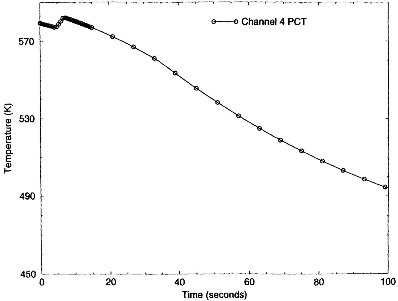
Figure 30: Peak Cladding Temperature for Hot Channel Component 4 (0-100 sec)
