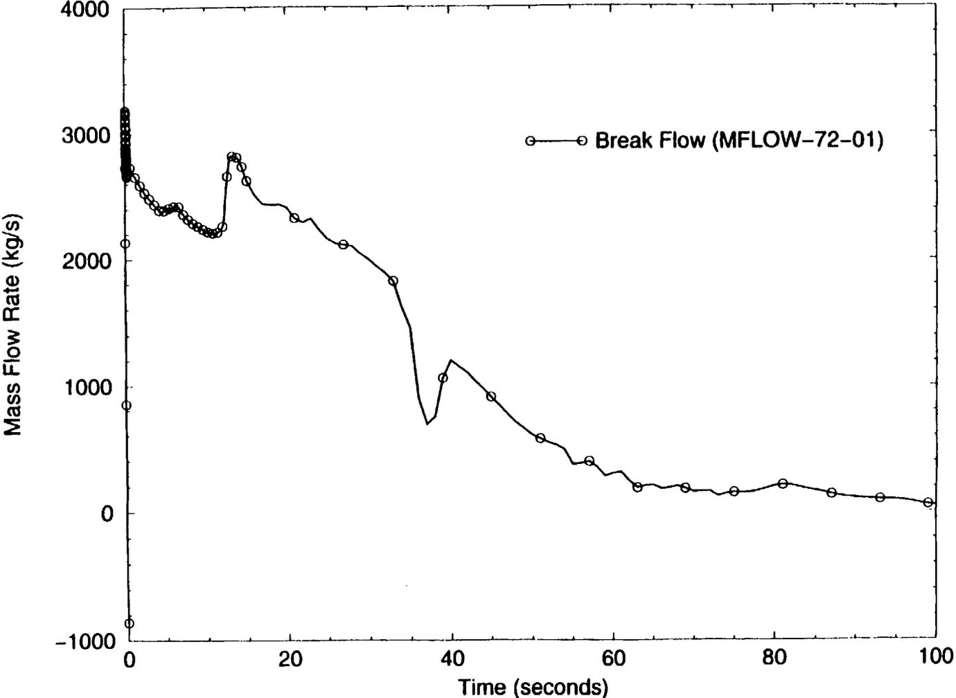
Figure 5: Mass Flow Rate in the Broken Feedwater Line (0-100 sec)
