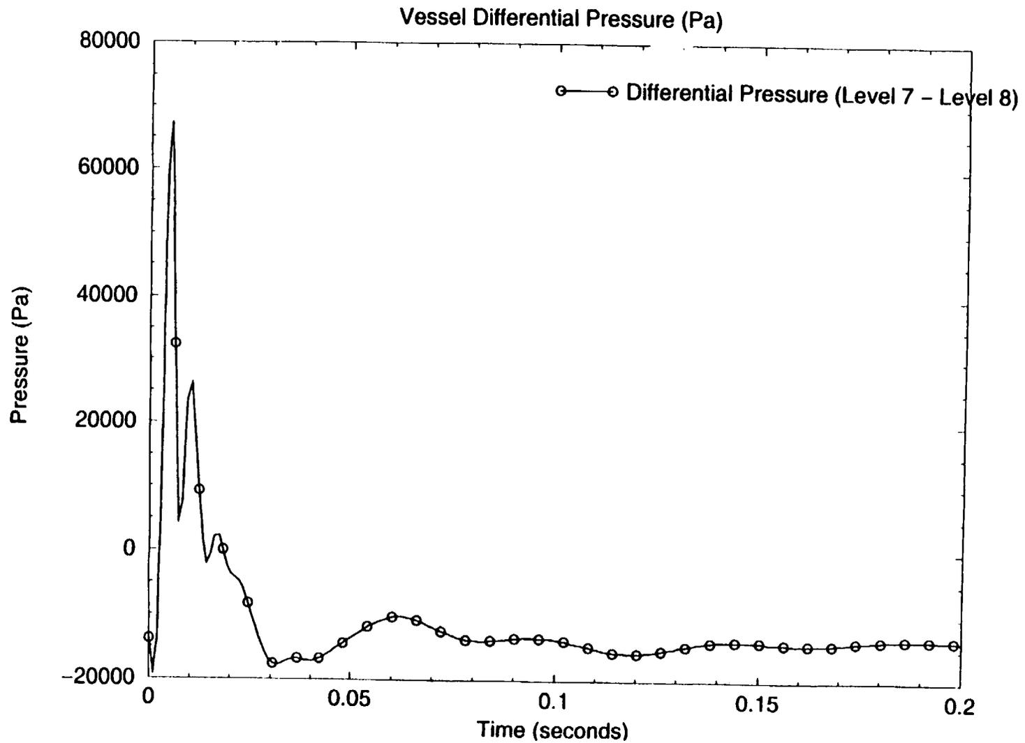
Figure 32: Differential Pressure Between Level 7 and 8 in Cell 14 (0-0.2 sec)
