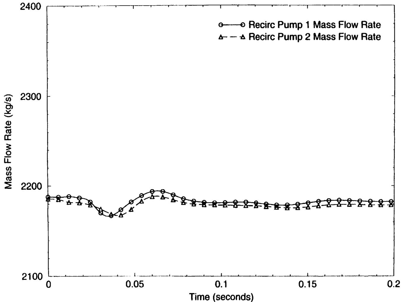
Figure 23: Recirculation Pump 1 and 2 Mass Flow Rates (0-0.2 sec)
