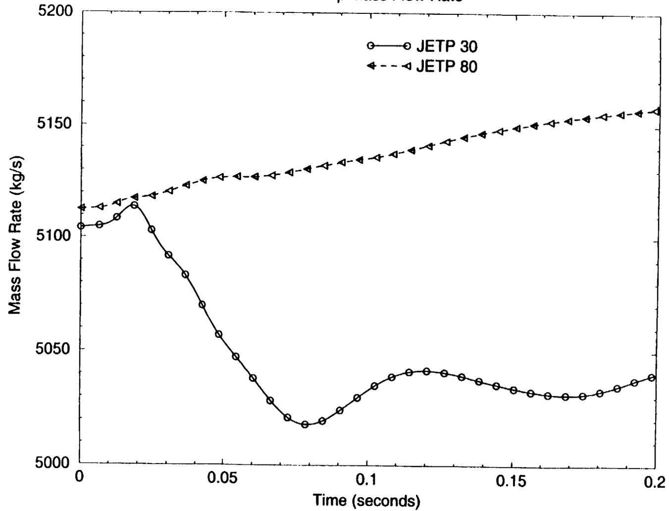
Figure 17: Mass Flow Rate in Jet Pump Components 30 and 80 (0-0.2 sec)
