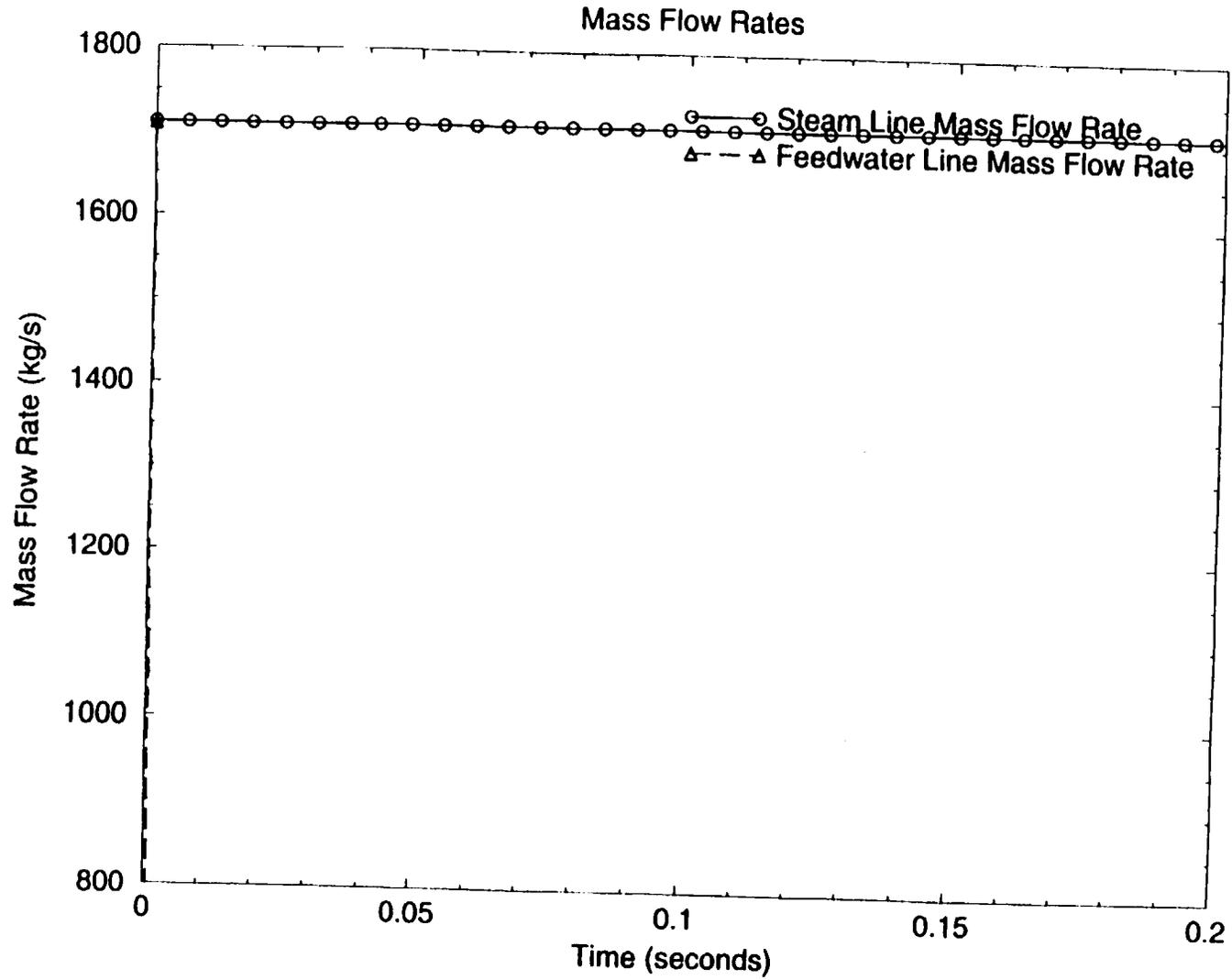
Figure 20: Steam Line and Feedwater Mass Flow Rates (0-0.2 sec)
