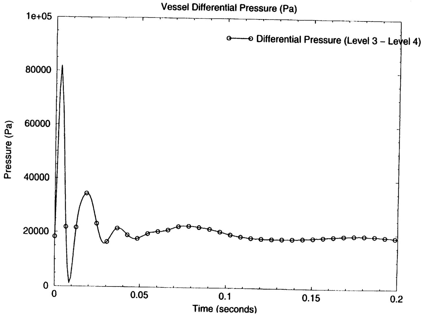
Figure 21: Differential Pressure Between Level 4 and 3 in Cell 13 (0-0.2 sec)
