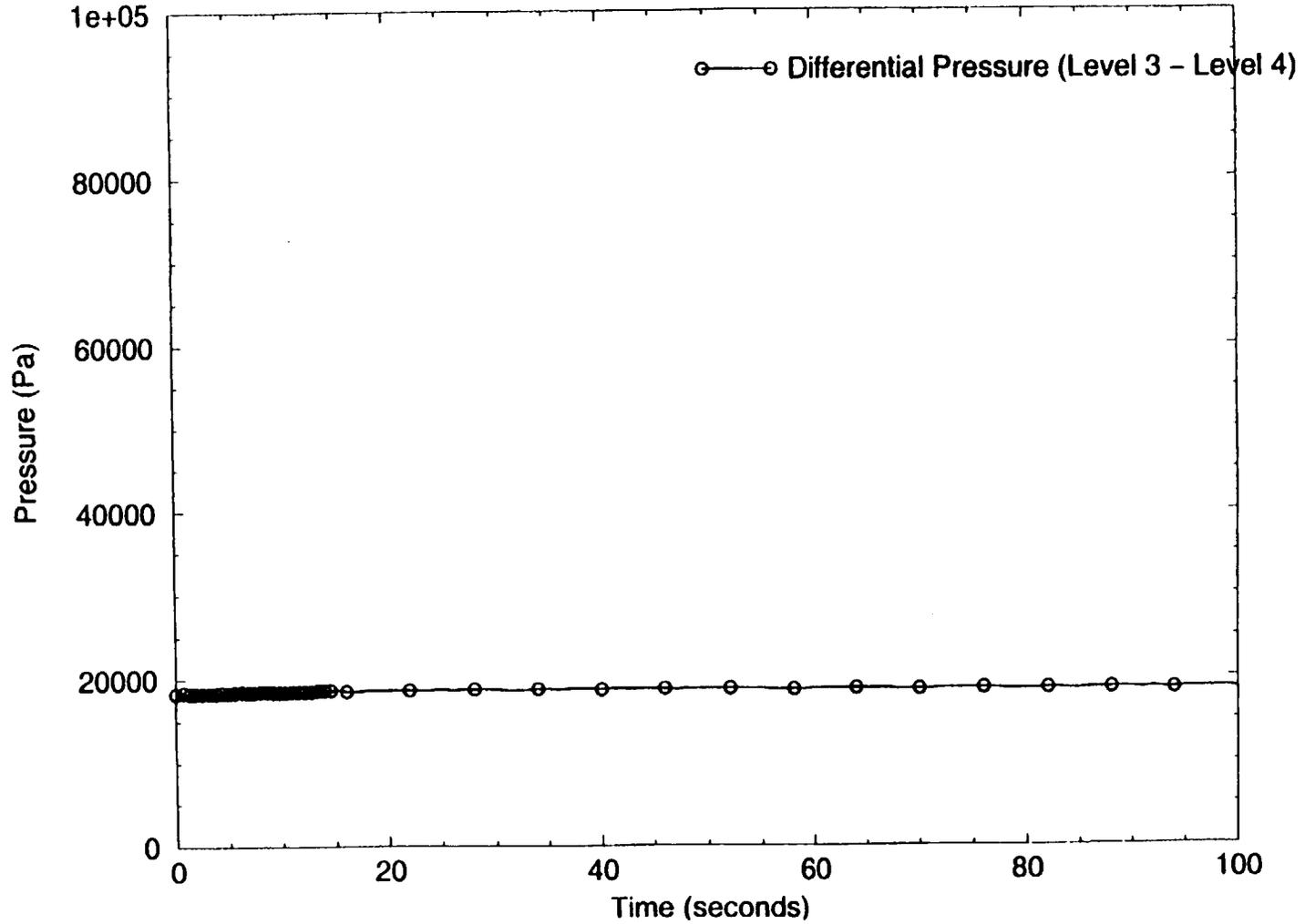
Figure 22: Differential Pressure Between Level 4 and 3 in Cell 13 (0-100 sec)
