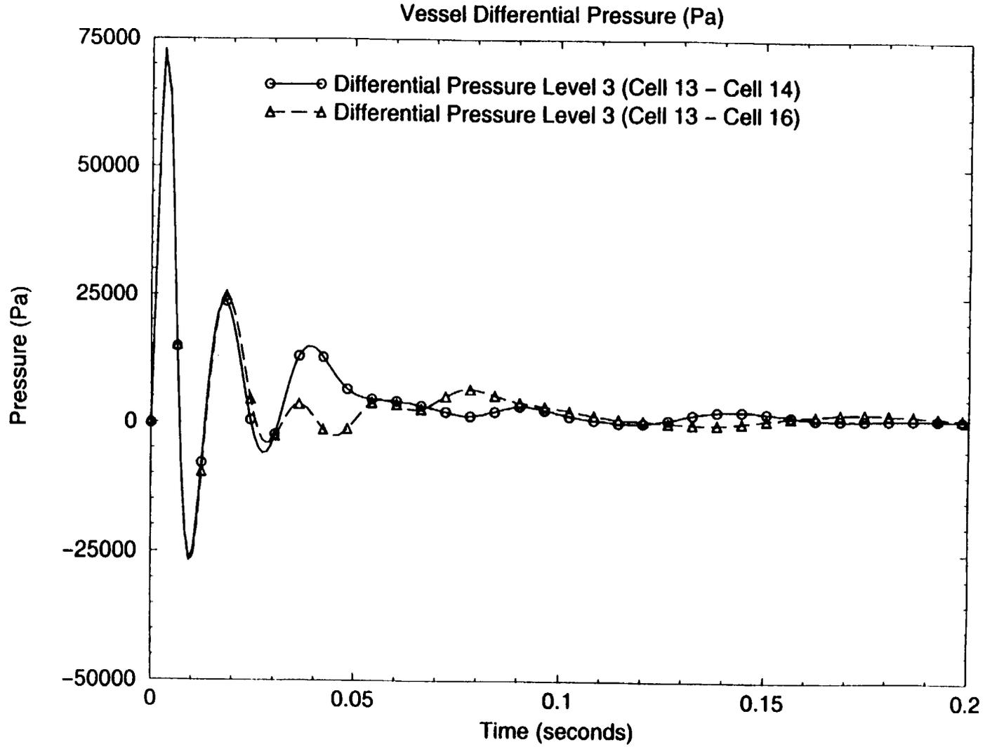
Figure 23: Differential Pressure Between Cell 13, 14 and 16 in Level 3 (0-0.2 sec)
