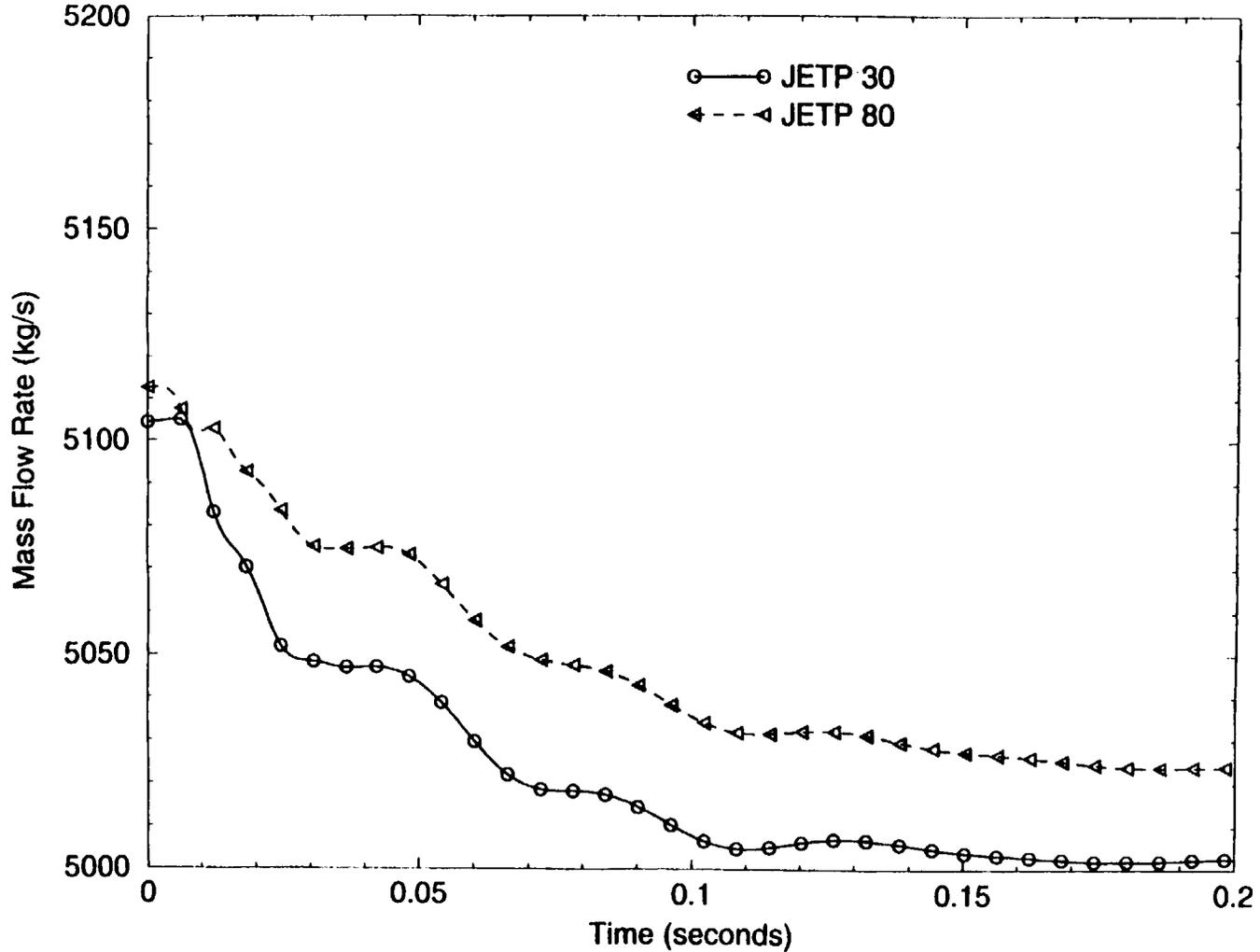
Figure 27: Mass Flow Rate in Jet Pump Components 30 and 80 (0-0.2 sec)
