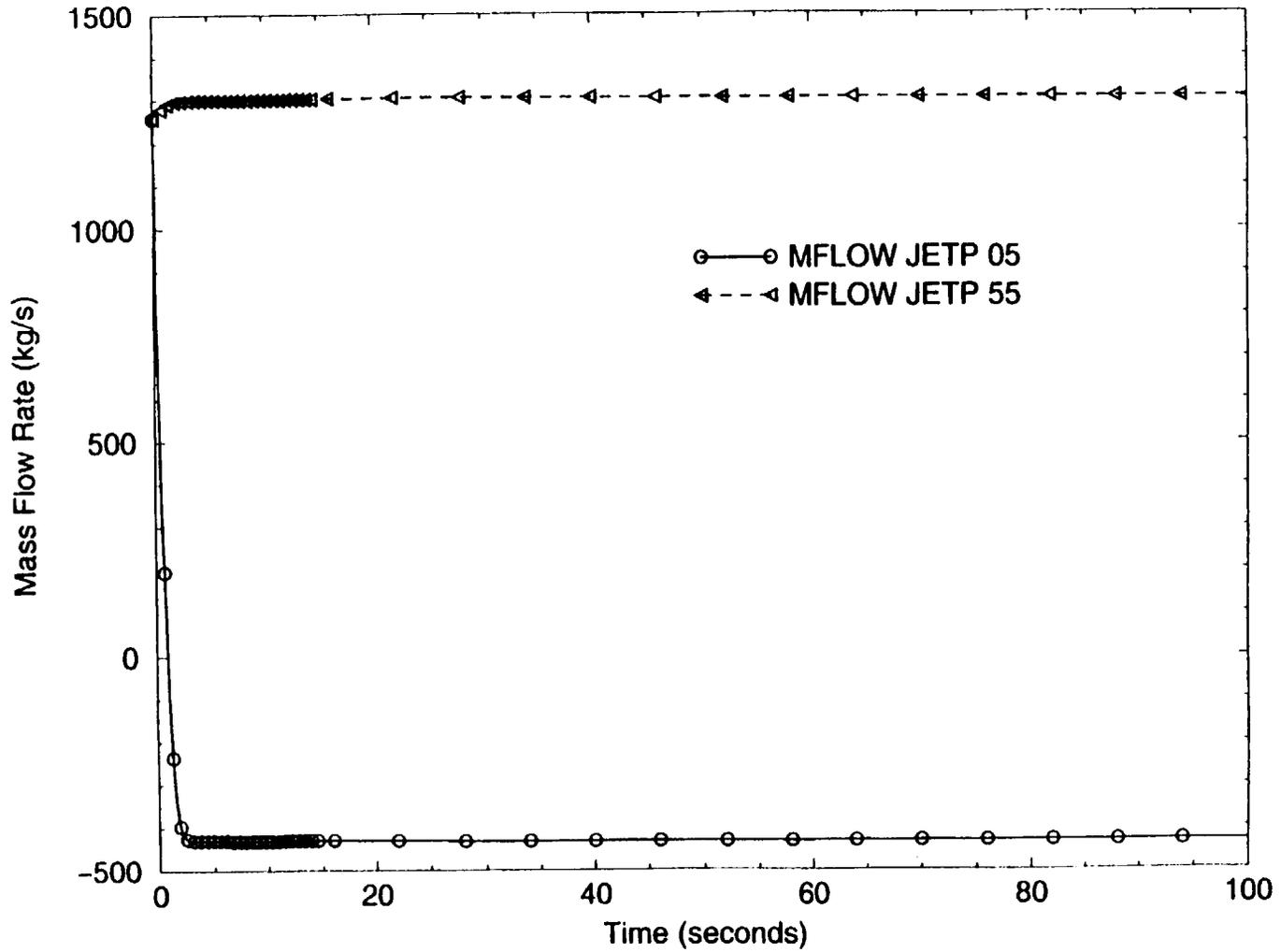
Figure 16: Mass Flow Rate in Jet Pump Components 5 and 55 (0-100 sec)
