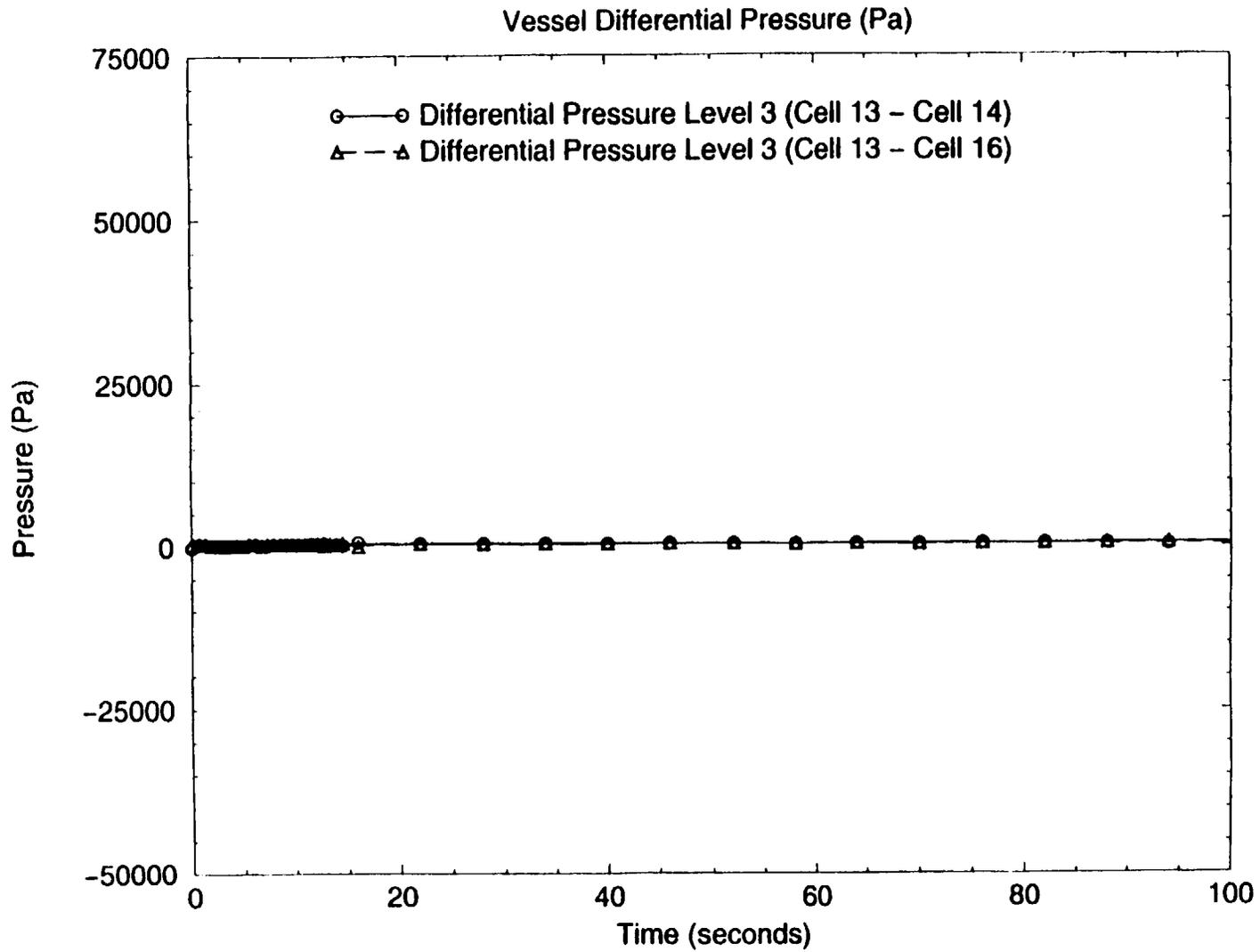
Figure 24: Differential Pressure Between Cell 13, 14 and 16 in Level 3 (0-100 sec)
