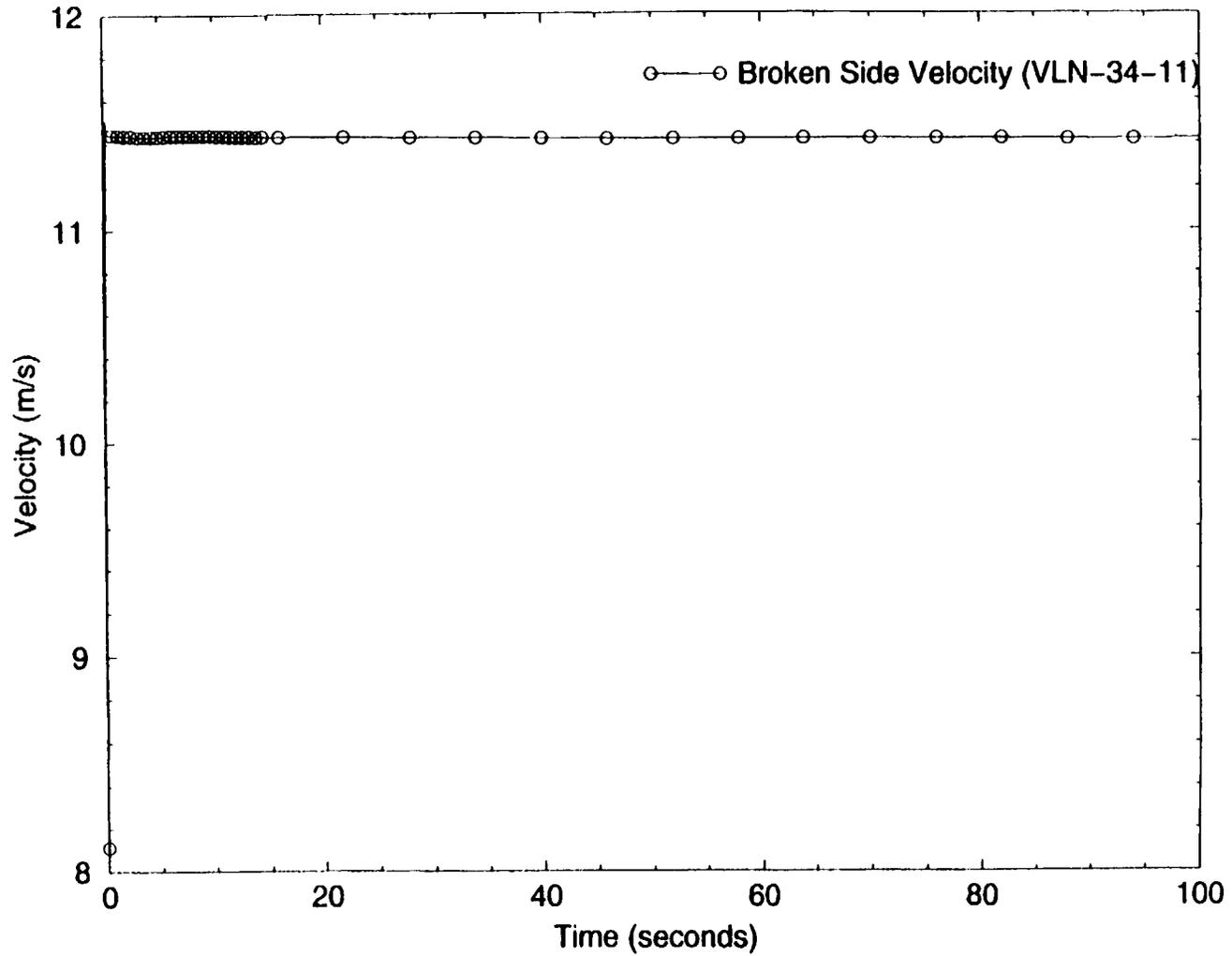
Figure 8: Liquid Velocity in the Broken Side of the Recirculation line (0-100 sec)
