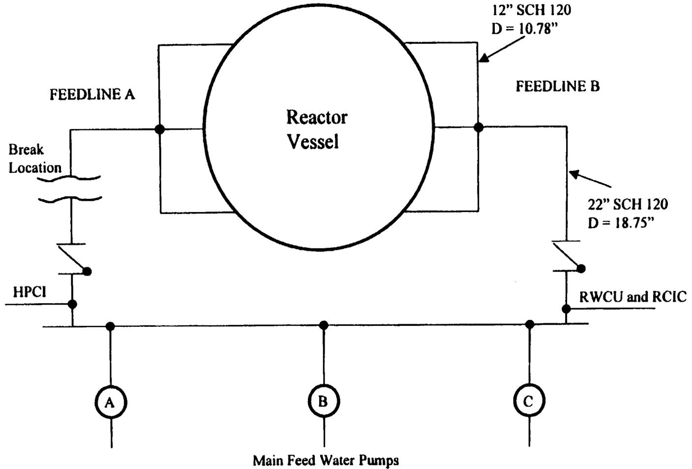
**Figure 1: Feedwater Piping Diagram, Showing Break Location**
