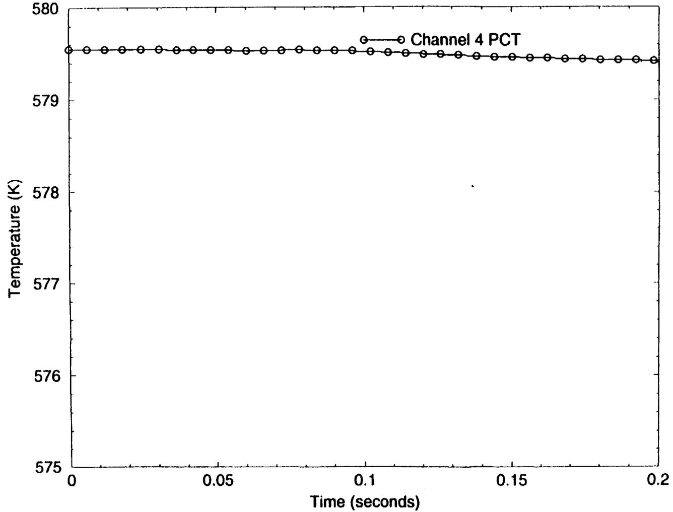
Figure 29: Peak Cladding Temperature for Hot Channel Component 4 (0-0.2 sec)
