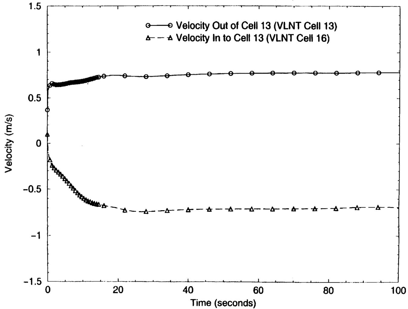
Figure 26: Azimuthal Liquid Velocities in And Out of Cell 13, Level 3 (0-100 sec)
