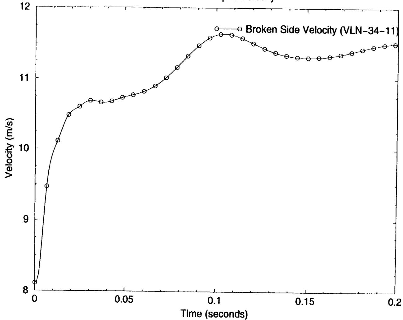
Figure 7: Liquid Velocity in the Broken Side of the Recirculation line (0-0.2 sec)
