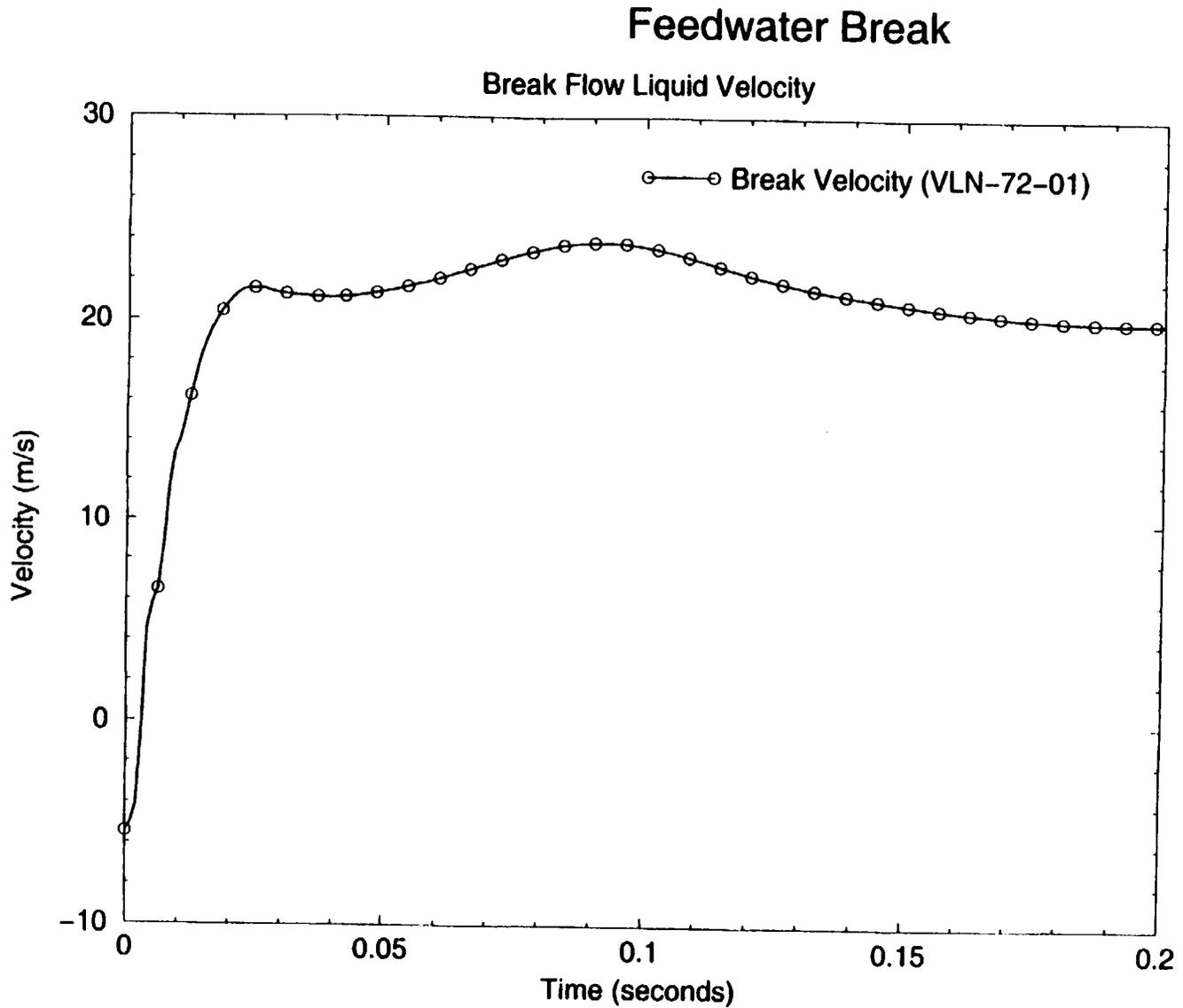
**Figure 6: Liquid Velocity in the Broken Feedwater Line (0-0.2 sec)**
