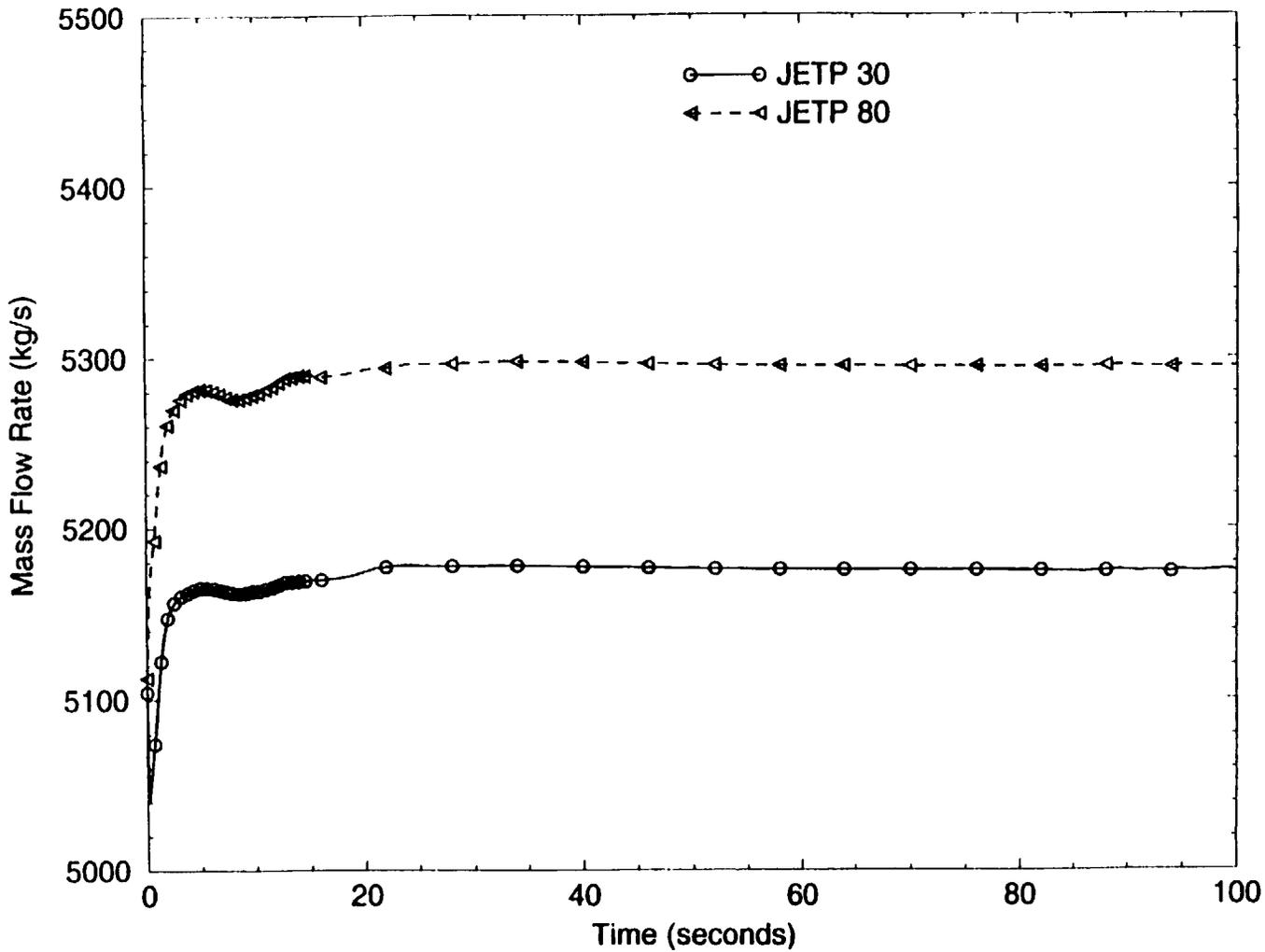
Figure 18: Mass Flow Rate in Jet Pump Components 30 and 80 (0-100 sec)
