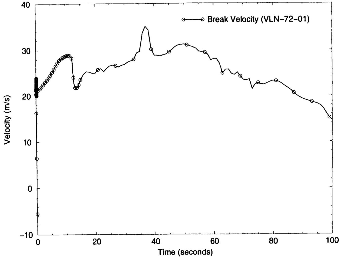
Figure 7: Liquid Velocity in the Broken Feedwater Line (0-100 sec)
