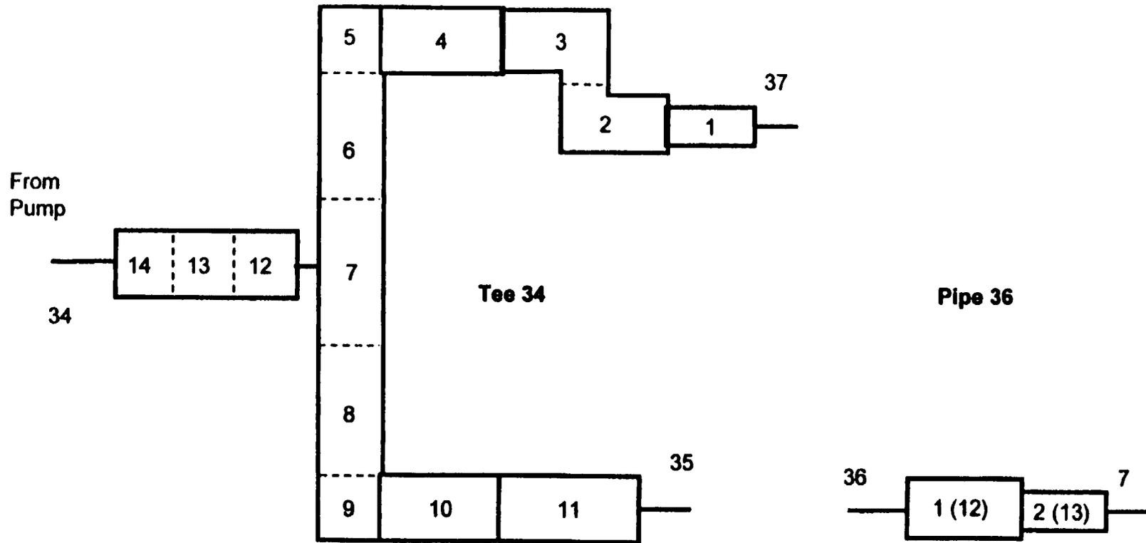
Figure 3: Renodalization of Tee Component 34
