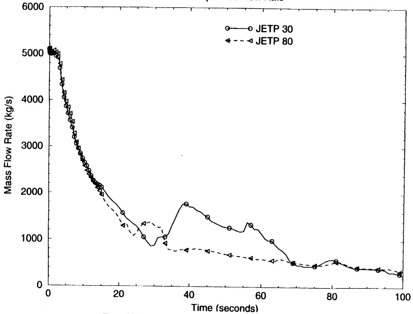
Figure 28: Mass Flow Rate in Jet Pump Components 30 and 80 (0-100 sec)
