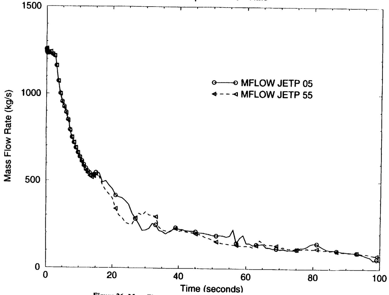
Figure 26: Mass Flow Rate in Jet Pump Components 5 and 55 (0-100 sec)
