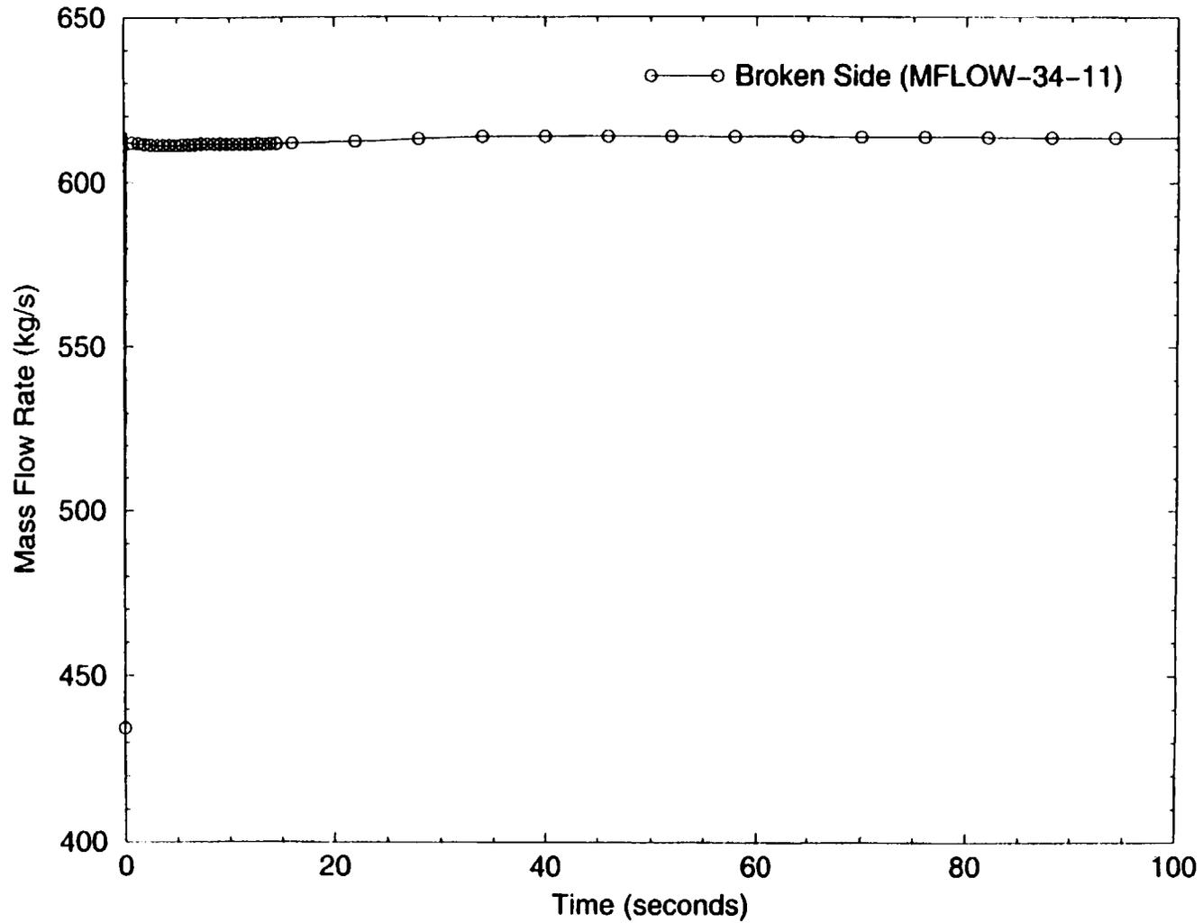
**Figure 6: Mass Flow Rate in the Broken Side of the Recirculation Line (0-100 sec)**
