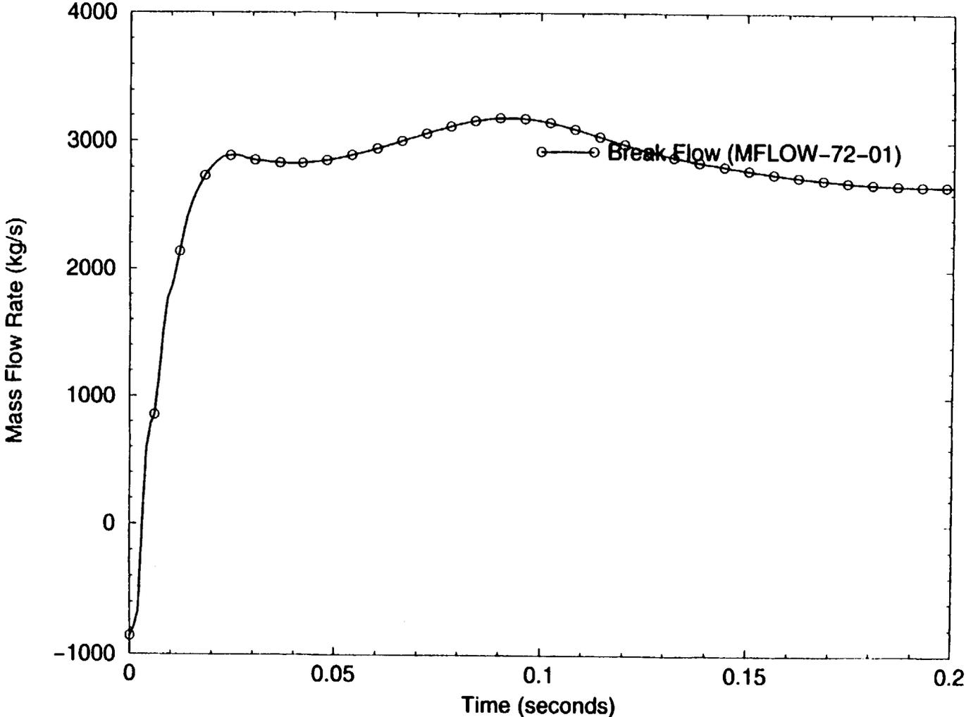
Figure 4: Mass Flow Rate in the Broken Feedwater Line (0-0.2 sec)
