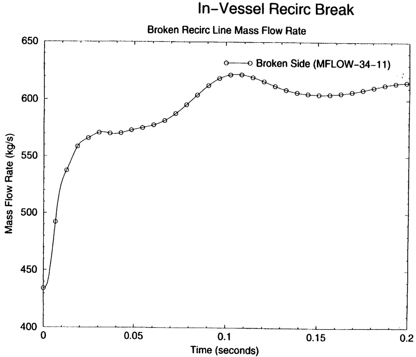
**Figure 5: Mass Flow Rate in the Broken Side of the Recirculation Line (0-0.2 sec)**
