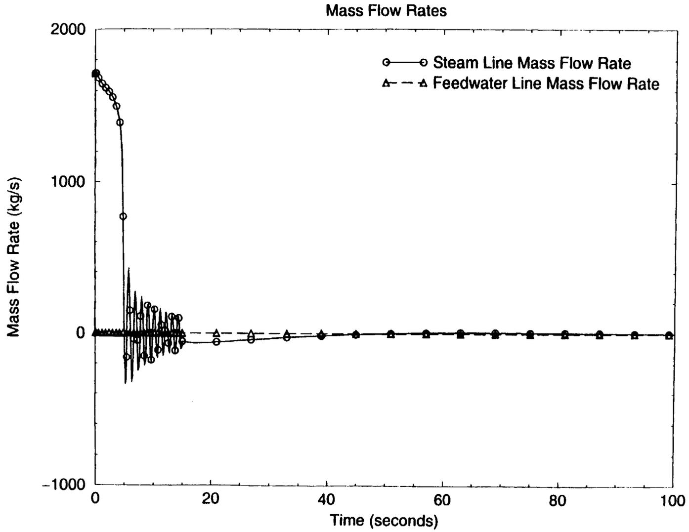
Figure 21: Steam Line and Feedwater Mass Flow Rates (0-100 sec)
