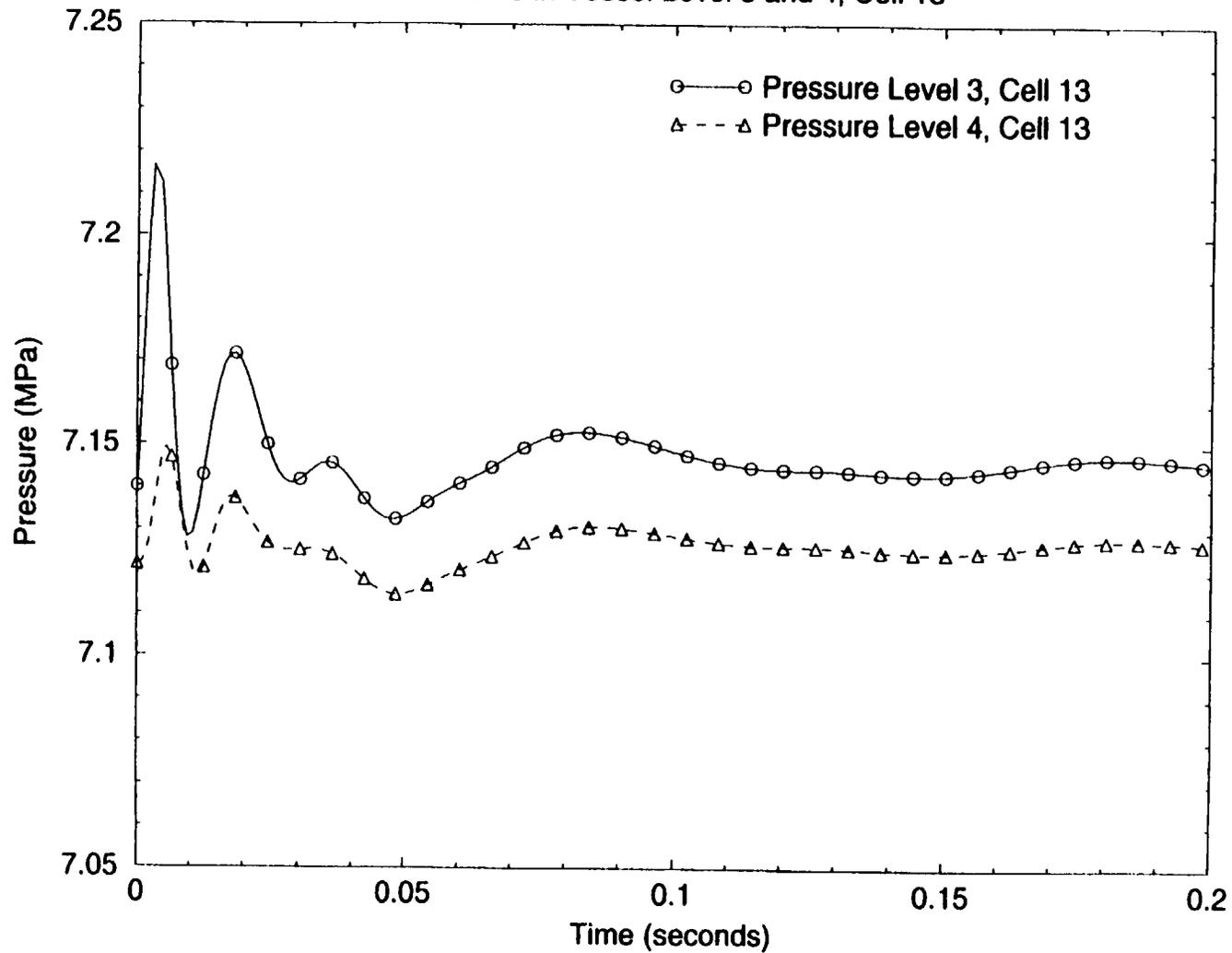
Figure 19: Pressure in Vessel Level 3, Cell 13, and Level 4 and Cell 13 (0-0.2 sec)
