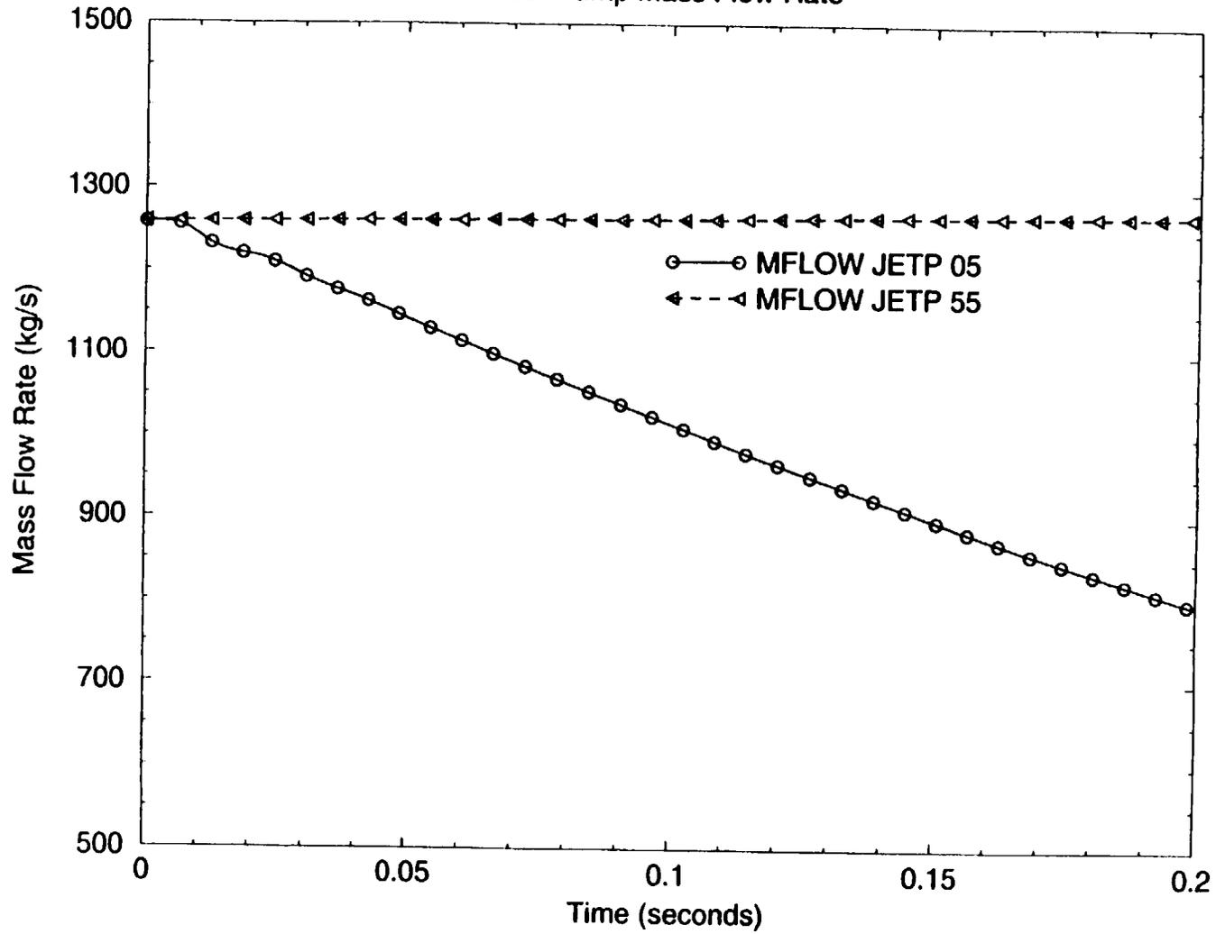
Figure 15: Mass Flow Rate in Jet Pump Components 5 and 55 (0-0.2 sec)
