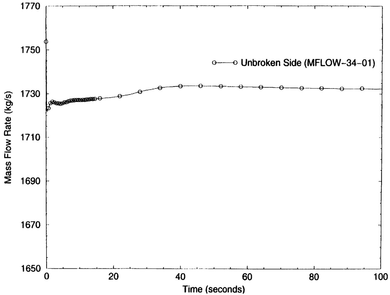
Figure 14: Mass Flow Rate in the Intact Side of the Recirculation Line (0-100 sec)
