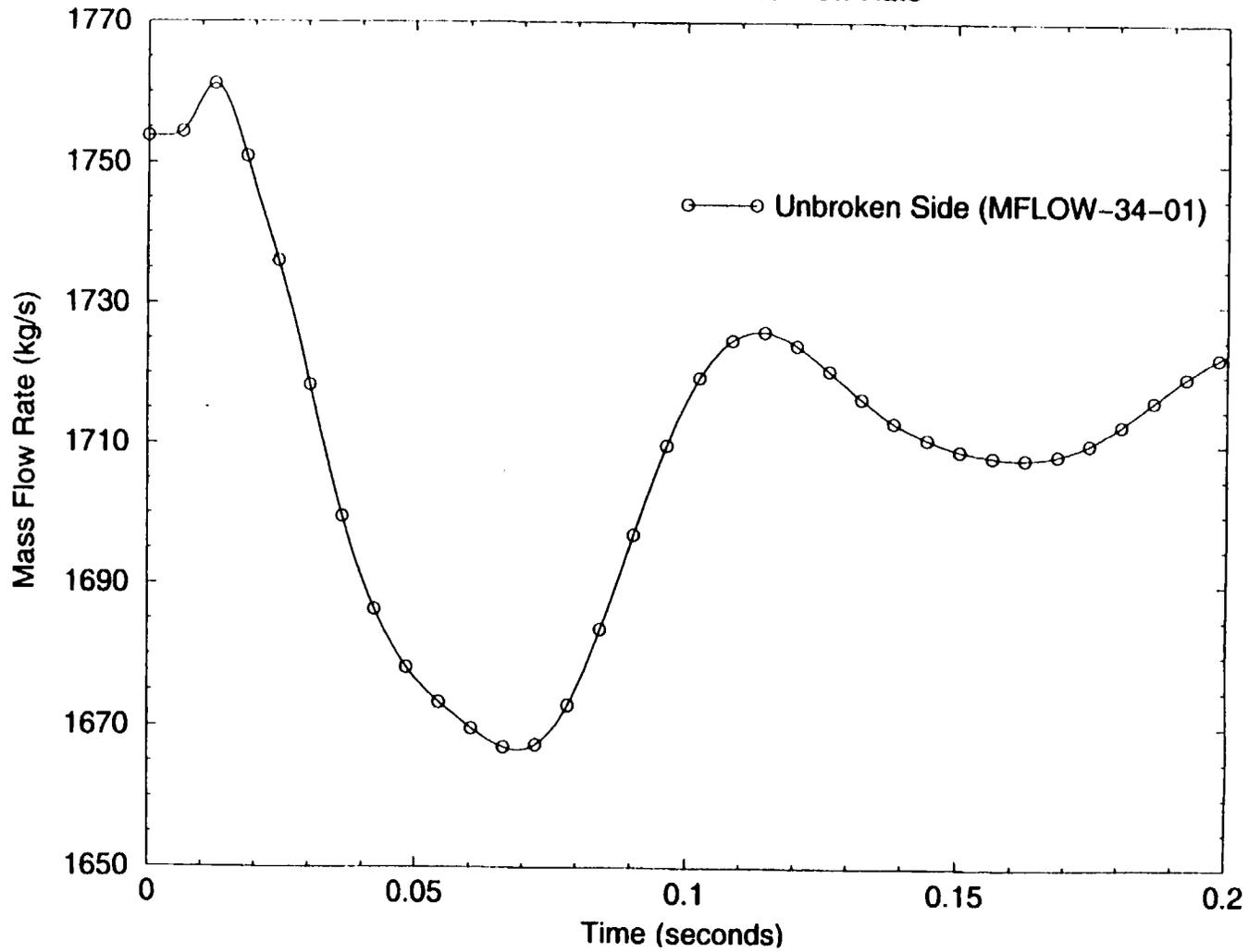
Figure 13: Mass Flow Rate in the Intact Side of the Recirculation Line (0-0.2 sec)
