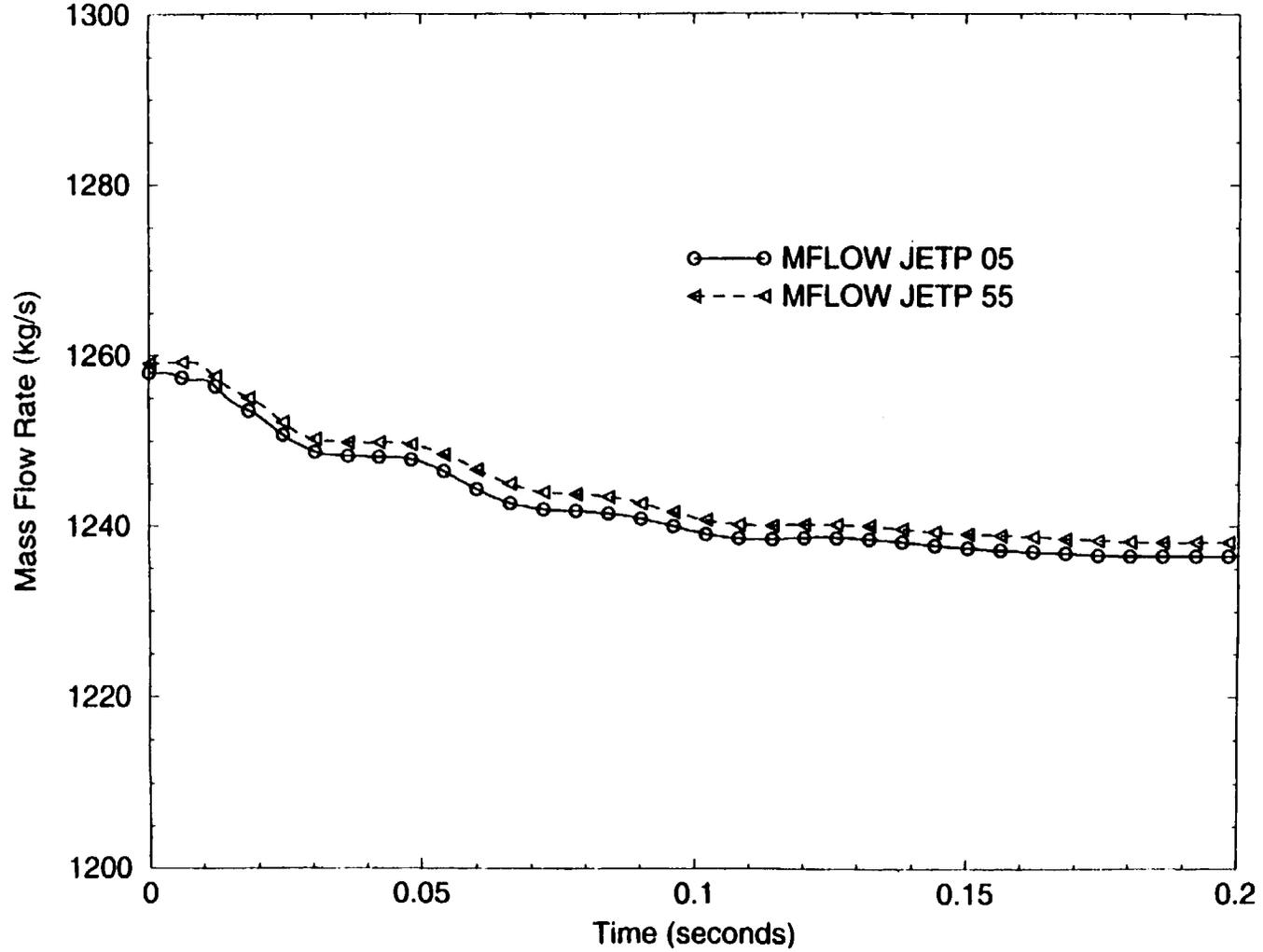
Figure 25: Mass Flow Rate in Jet Pump Components 5 and 55 (0-0.2 sec)
