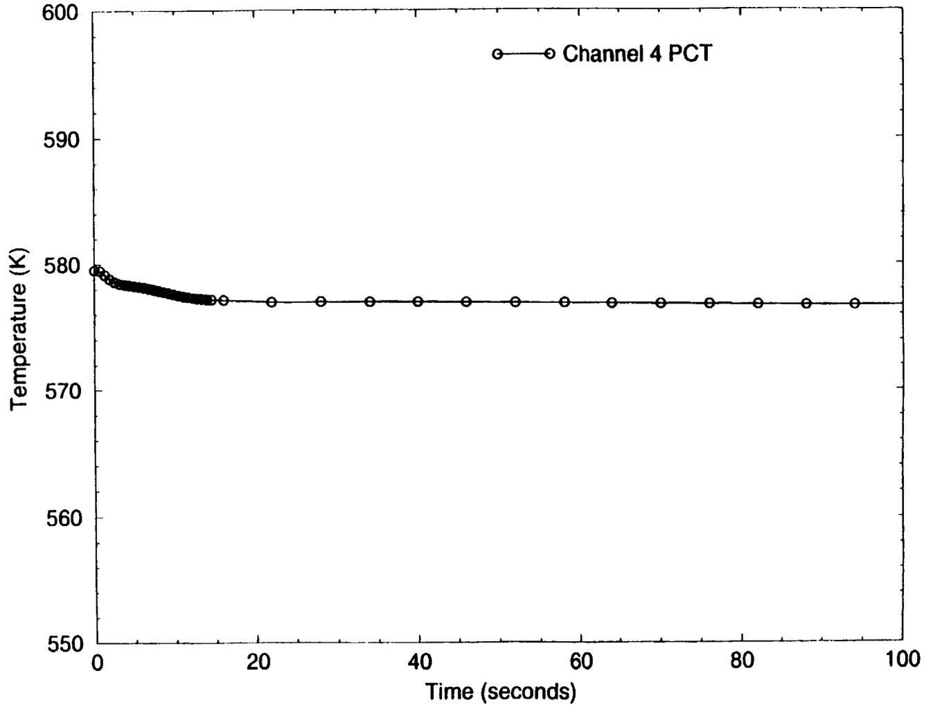
Figure 36: Peak Cladding Temperature for Hot Channel Component 4 (0-100 sec)
