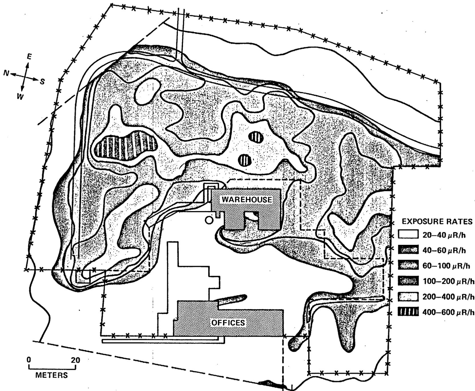
FIGURE 14. Exposure Rates ( $\mu\text{R}/\text{h}$ ) at 1 m Above the Surface on the W.R. Grace Property.
