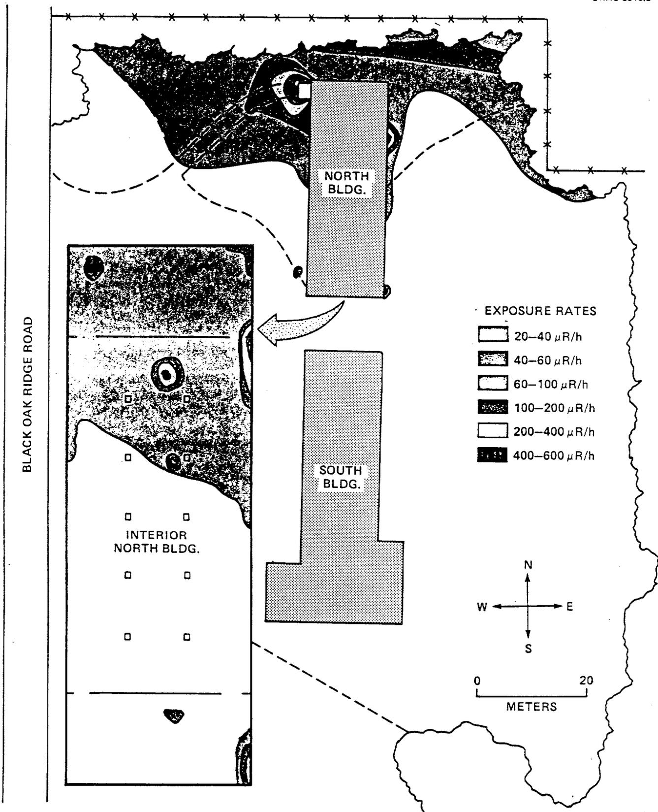
FIGURE 16: Surface Exposure Rates ( $\mu\text{R}/\text{h}$ ) on the School Bus Maintenance Yard.
