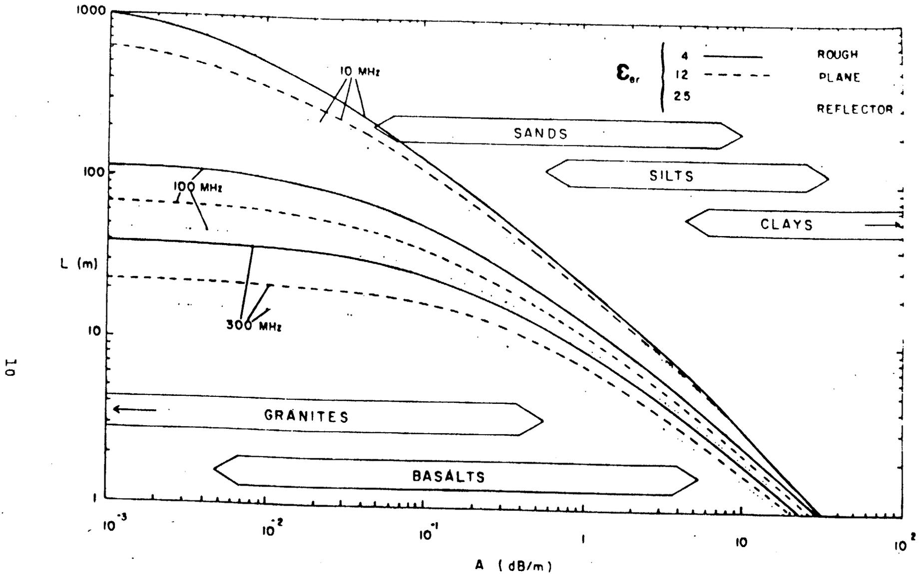
Figure 2: Variation of maximum depth of penetration ( $L$ ) as a function of attenuation ( $A$ ) for different frequencies and dielectric constants. Typical ranges of attenuation for different earth materials are also shown (after Horton et al, 1981).
