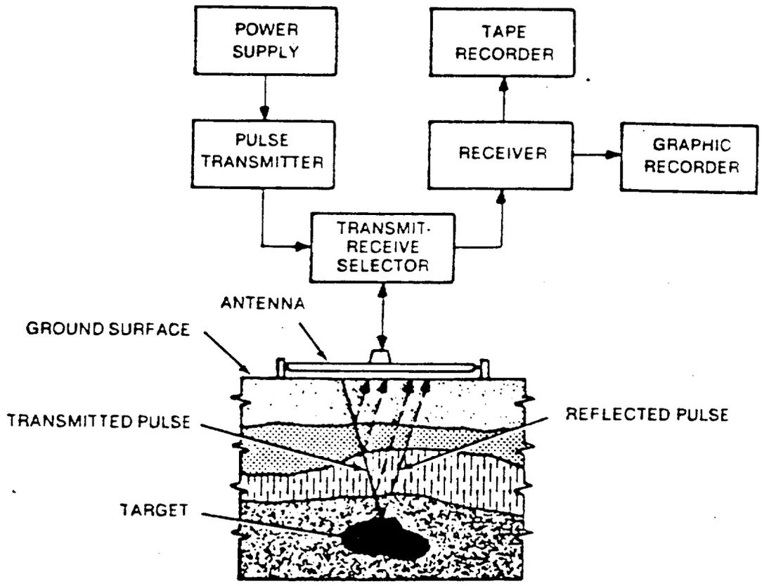
**Figure 3** Ground-Penetrating Radar (GPR) System, block diagram.
