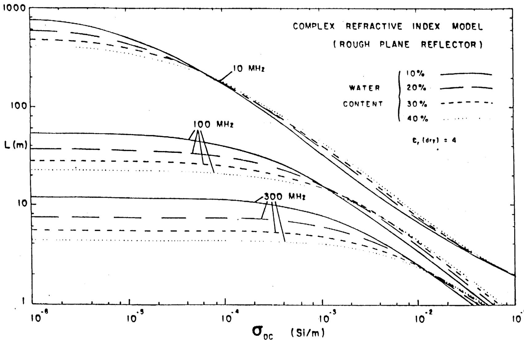
Figure 5: Radar range ( $L$ ) as a function of DC conductivity ( $\sigma_{\text{DC}}$ ) at different frequencies. Plots are based on a Complex Refractive Index Soil Model and reflection from a rough plane reflector. (after Horton et al, 1981).
