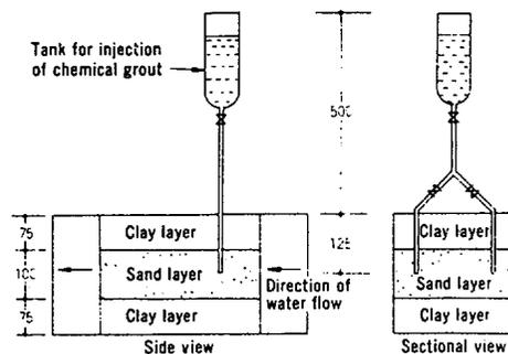
Solidification of various chemical grouts in water cut-off experiment.
