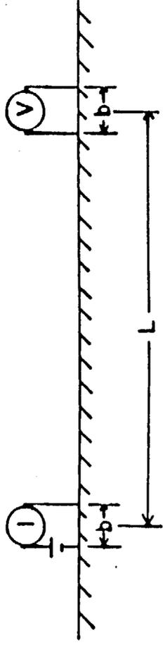
Figure 4: Common electrode configurations for resistivity arrays.
