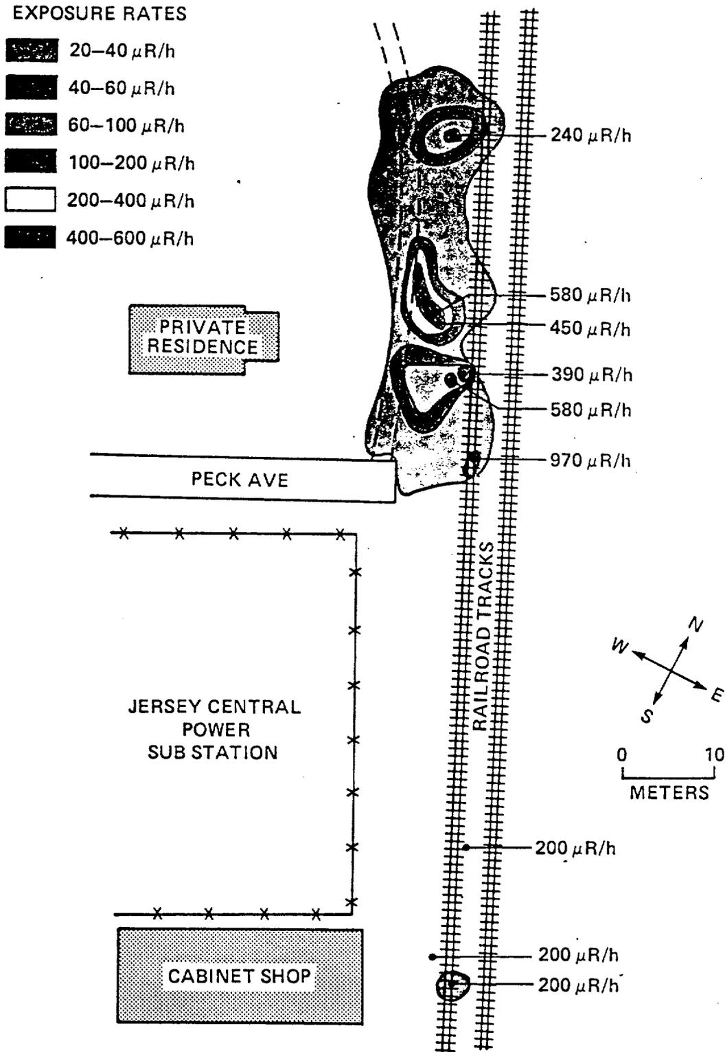
FIGURE 18. Surface Exposure Rates ( $\mu\text{R/h}$ ) Along the Erie Lackawanna Railroad in Pompton Plains.
