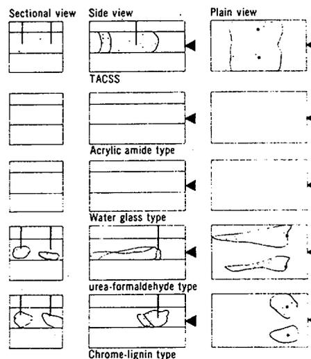
◀ Indicates the direction of water flow. A complete water cut-off wall was formed by TACSS only. Two kinds of other chemical grouts were entirely washed away.
