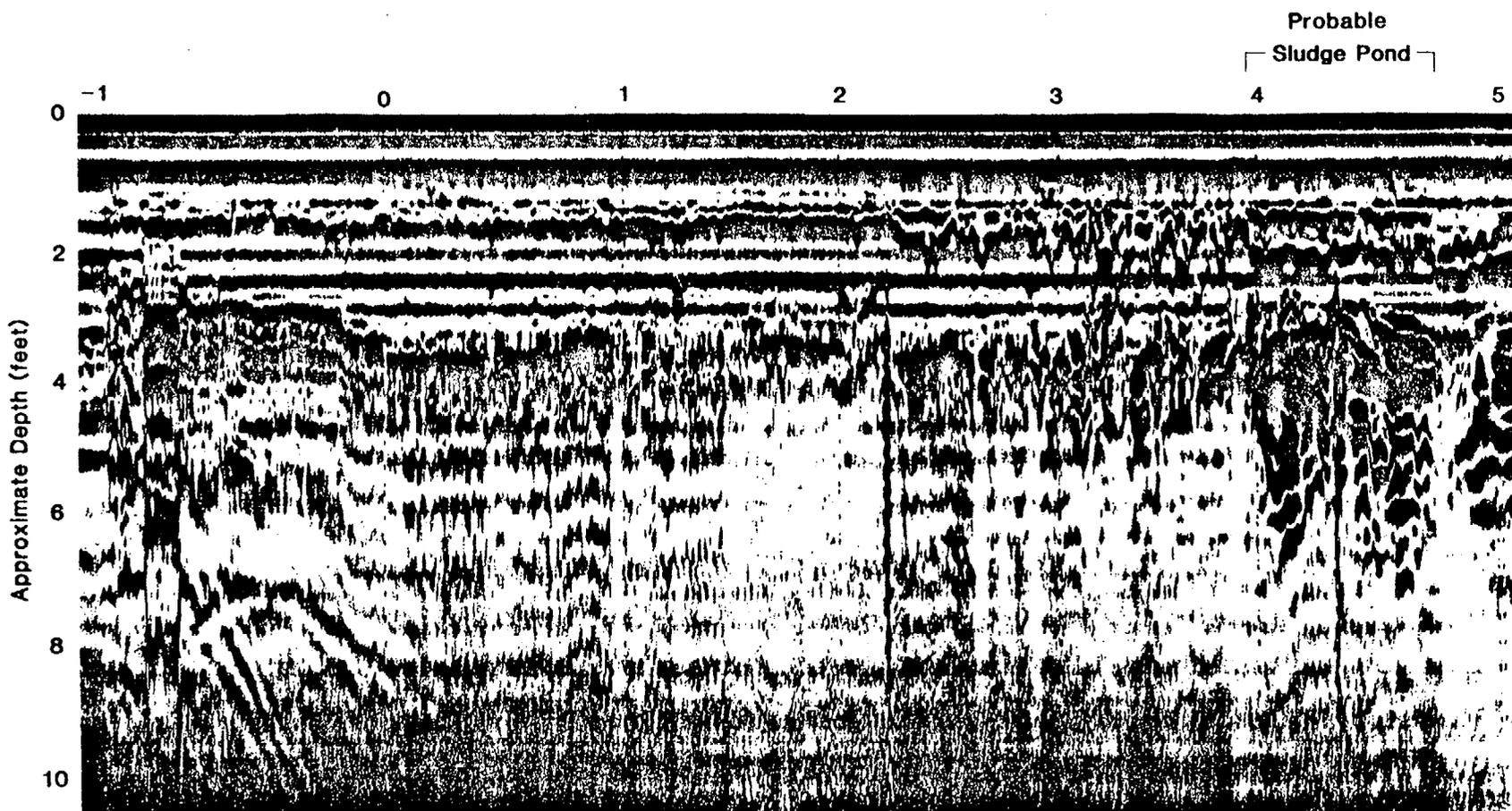
Figure 7: Radar profile along F+3 meters line.
