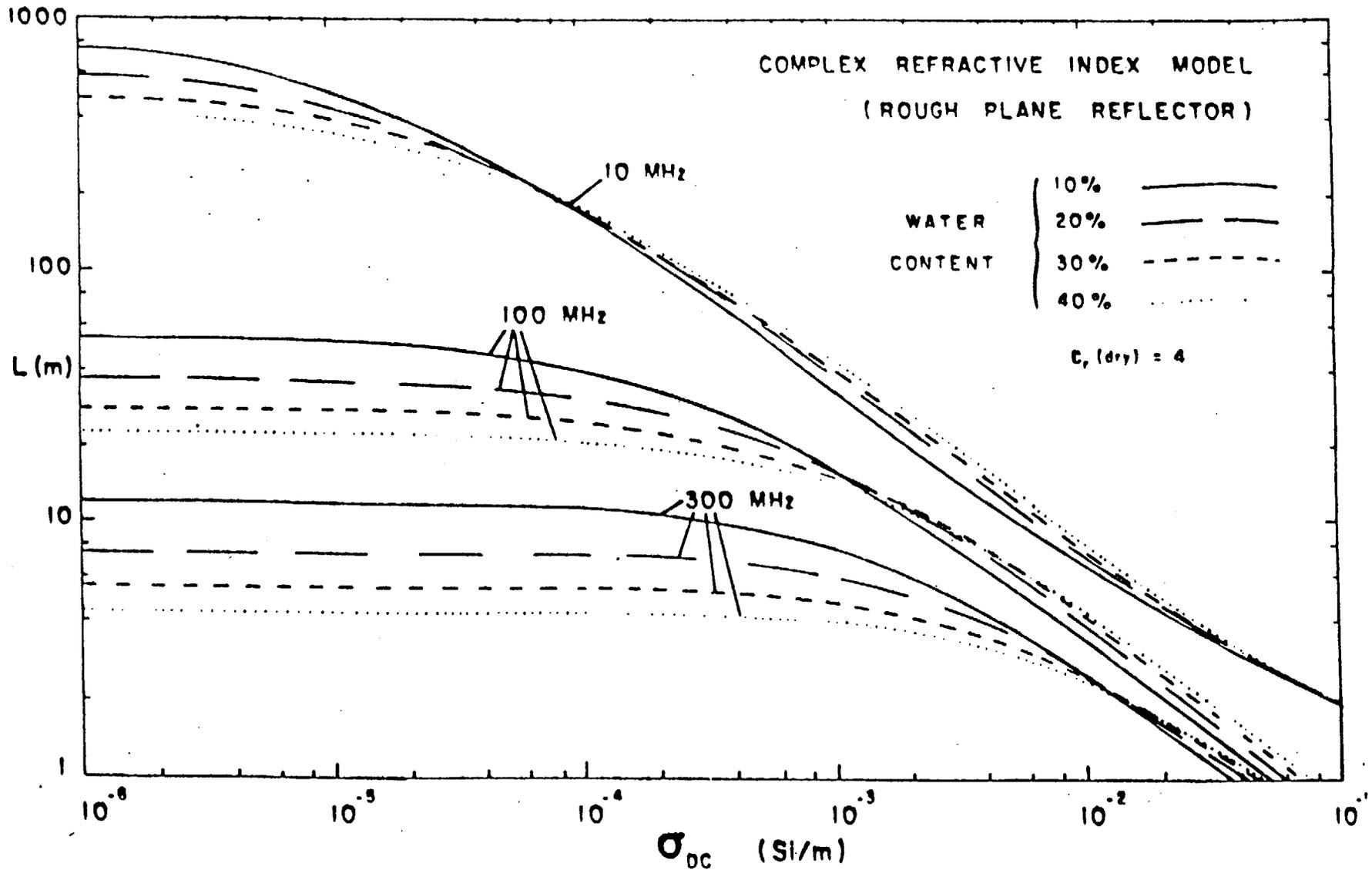
Figure 5: Radar range ( $L$ ) as a function of DC conductivity ( $\sigma_{DC}$ ) at different frequencies. Plots are based on a Complex Refractive Index Soil Model and reflection from a rough plane reflector. (after Horton et al, 1981).
