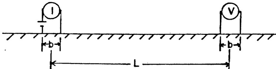
Figure 4: Common electrode configurations for resistivity arrays.
