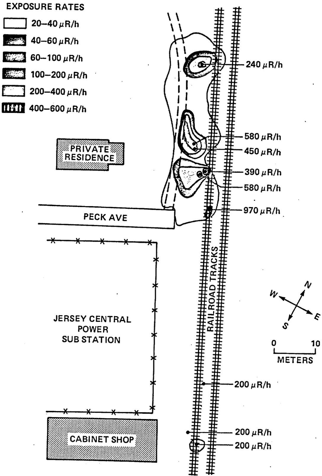
FIGURE 18. Surface Exposure Rates ( $\mu\text{R/h}$ ) Along the Erie Lackawanna Railroad in Pompton Plains.
