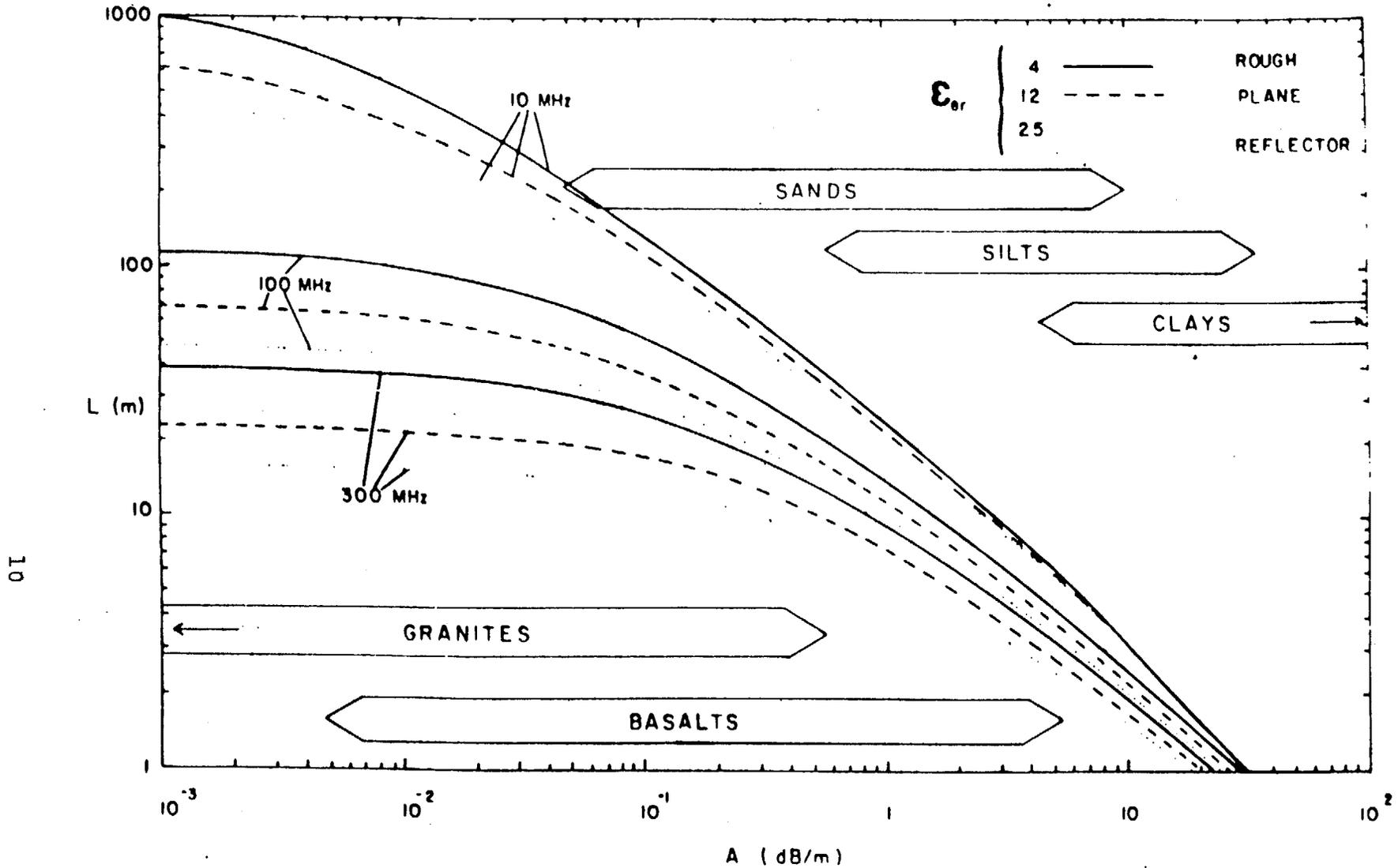
Figure 2: Variation of maximum depth of penetration (L) as a function of attenuation (A) for different frequencies and dielectric constants. Typical ranges of attenuation for different earth materials are also shown (after Horton et al, 1981).
