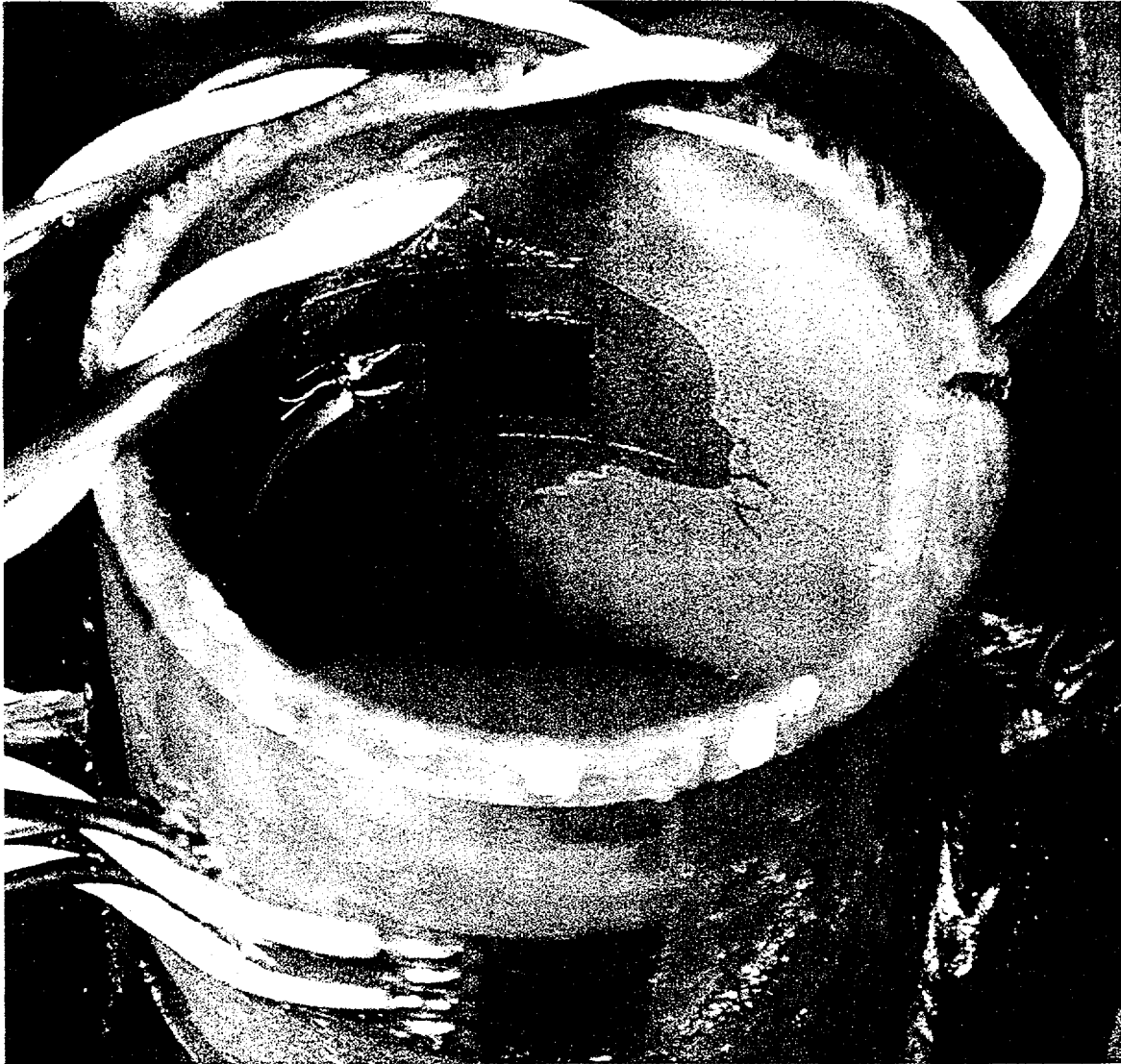
Strain Gage Attached to I.D. For Residual Stress Measurement Sample 00603-4
