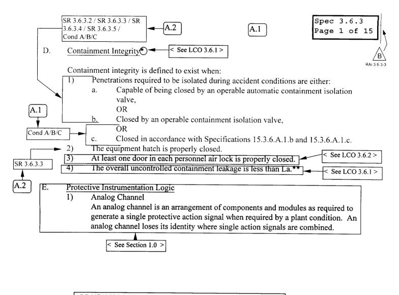
ADD NEW SRS 3.6.3.2 AND 3.6.3.3 TO PERIODICALLY VERIFY POSITION OF MANUAL CONTAINMENT ISOLATION VALVES AND BLANK FLANGES
