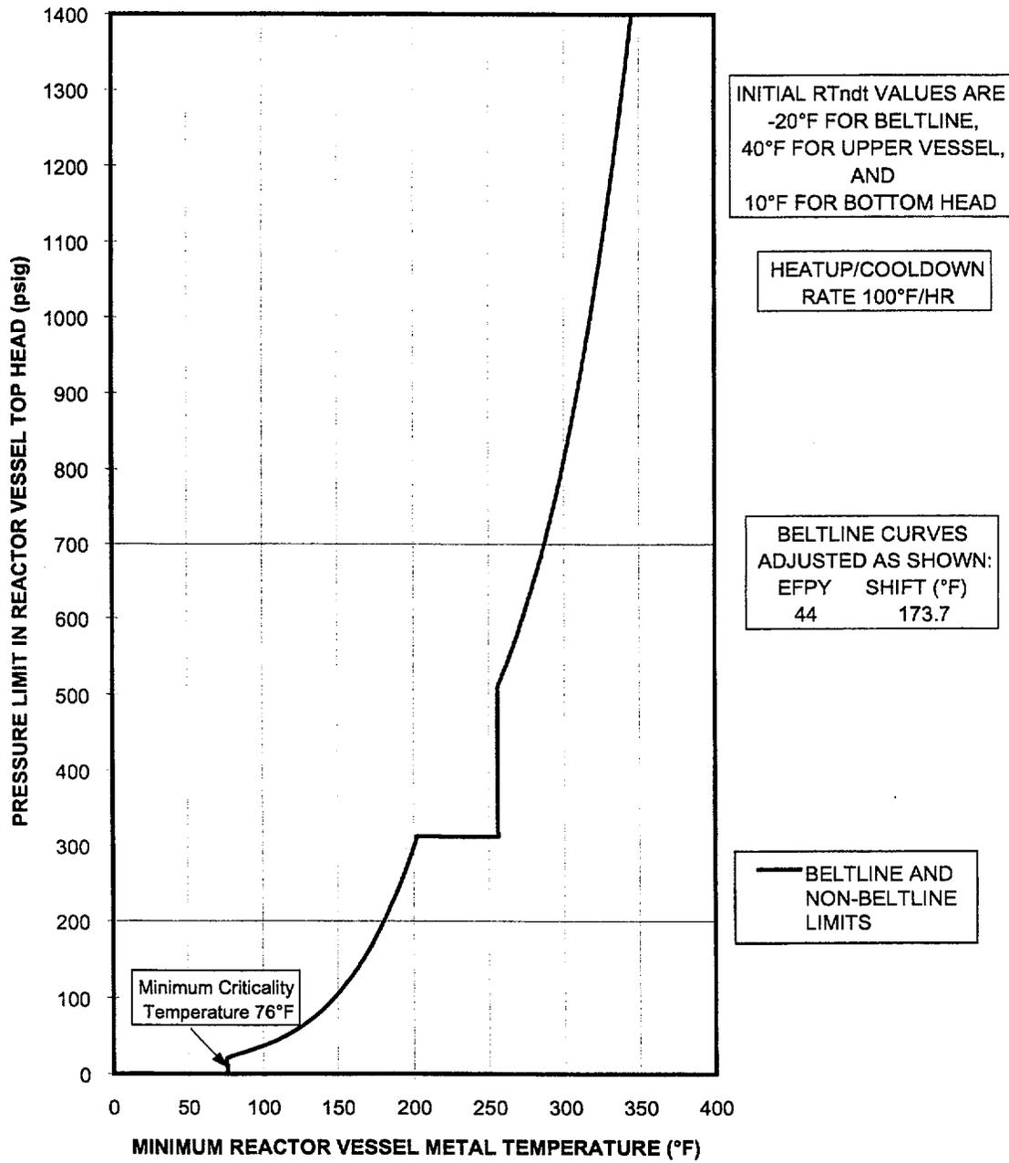
Figure C-3: P-T Curve for Unit 1 (Curve C)
