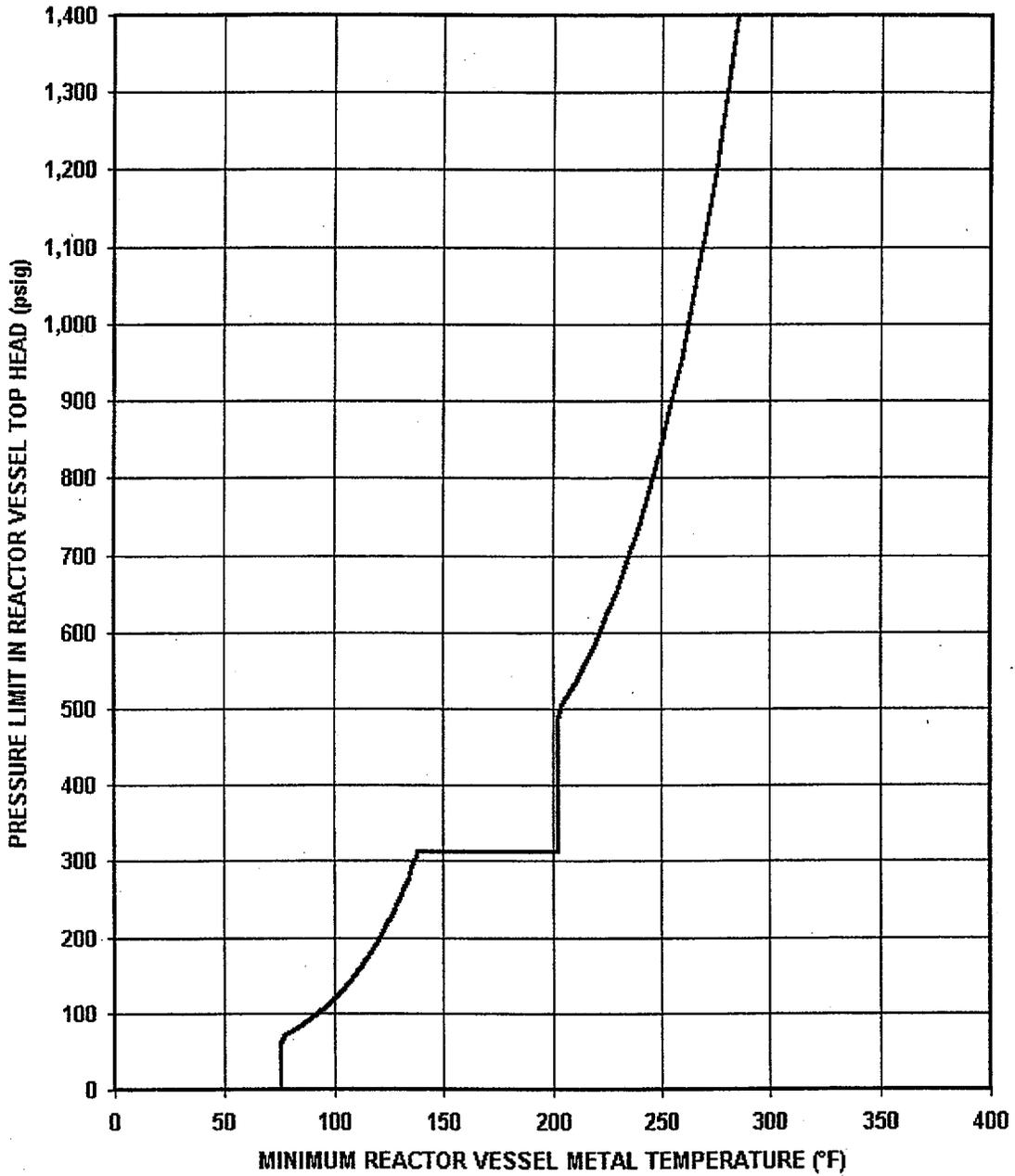
**Unit 1 Core Critical Curve (Curve C), 54 EFPY**
