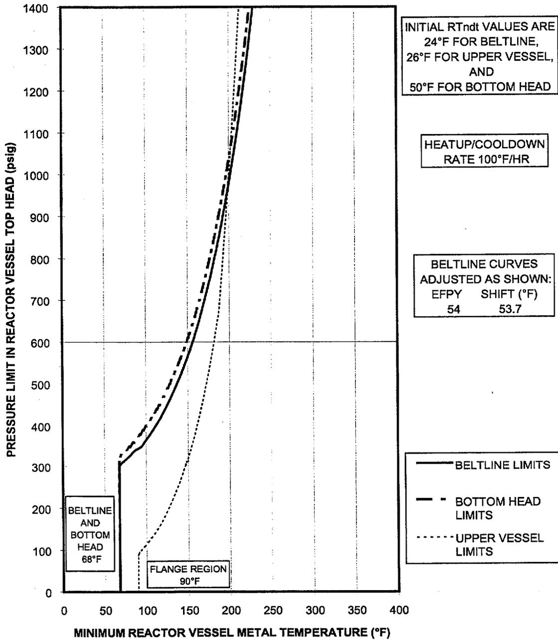
Figure 4-5: Non-Nuclear Heatup/Cooldown (Curve B) [Unit 2]
