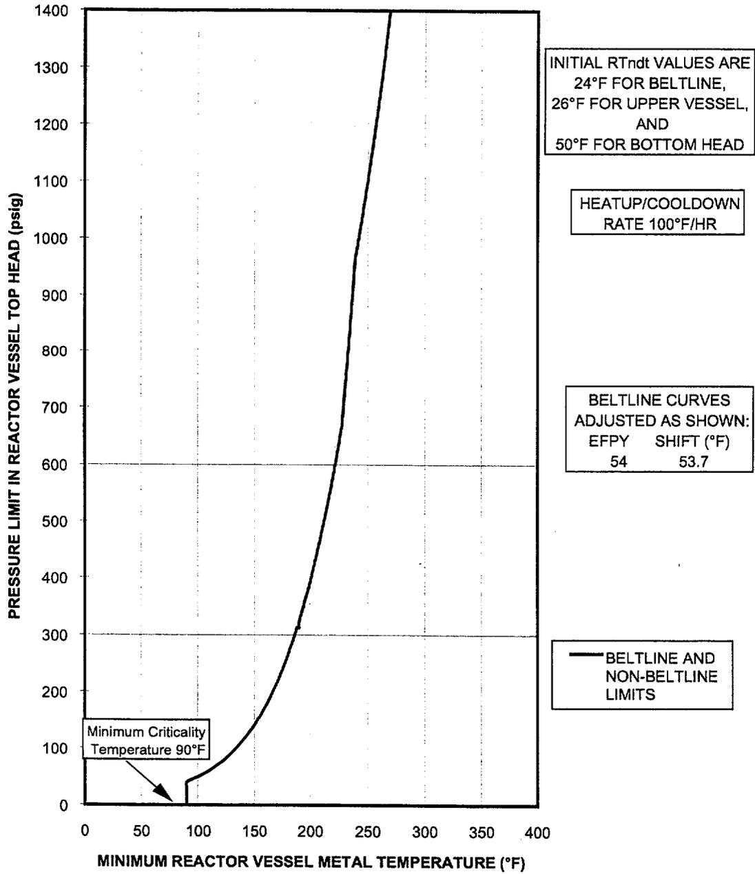
Figure 4-6: Core Critical Curve (Curve C) [Unit 2]
