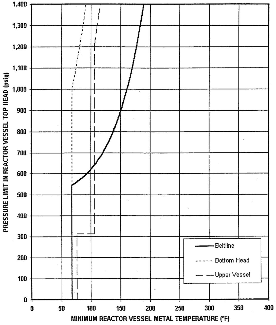
**Unit 1 Pressure Test Curve (Curve A), 32 EPFY**
