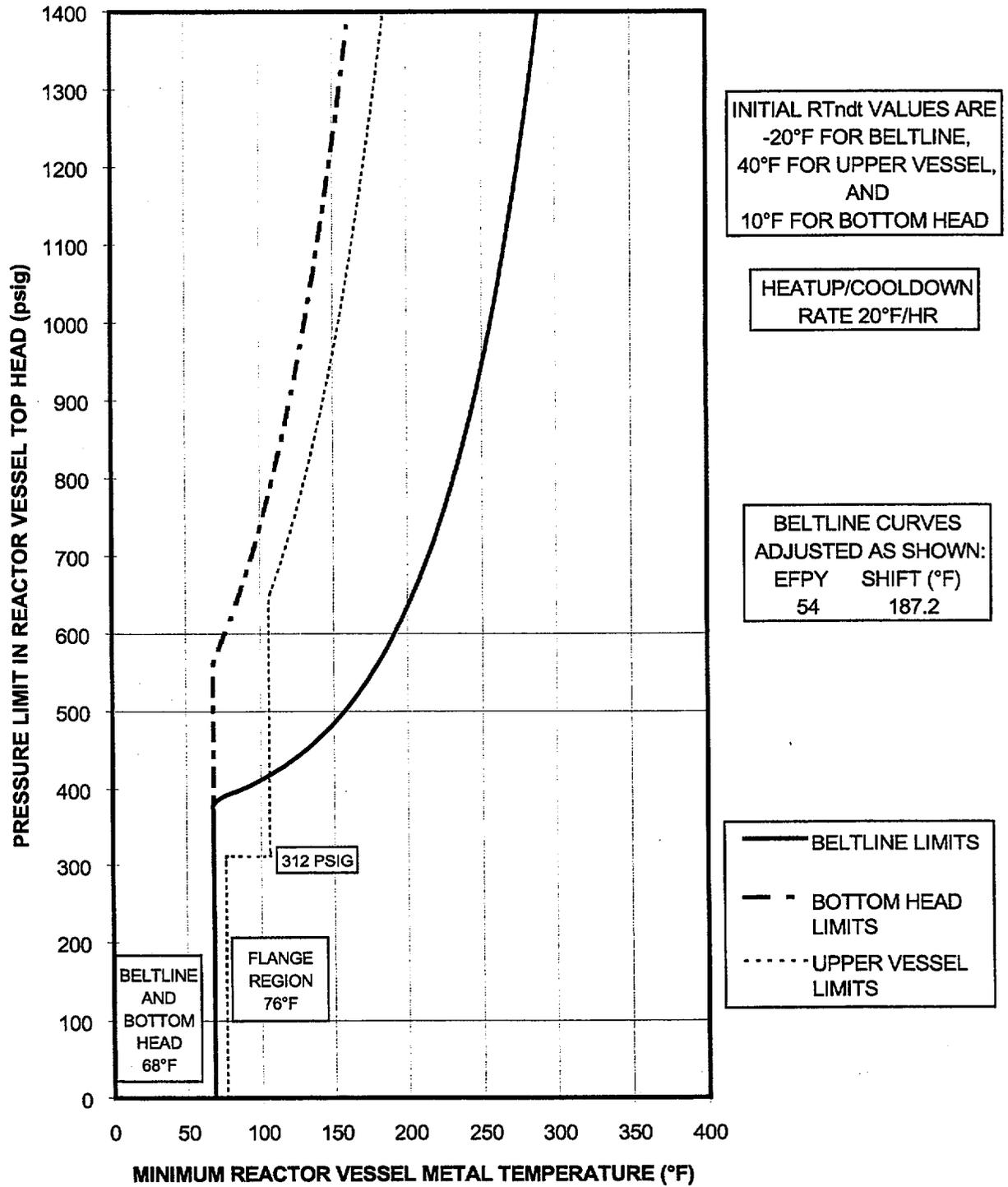
Figure 4-1: Pressure Test Curve (Curve A) [Unit 1]
