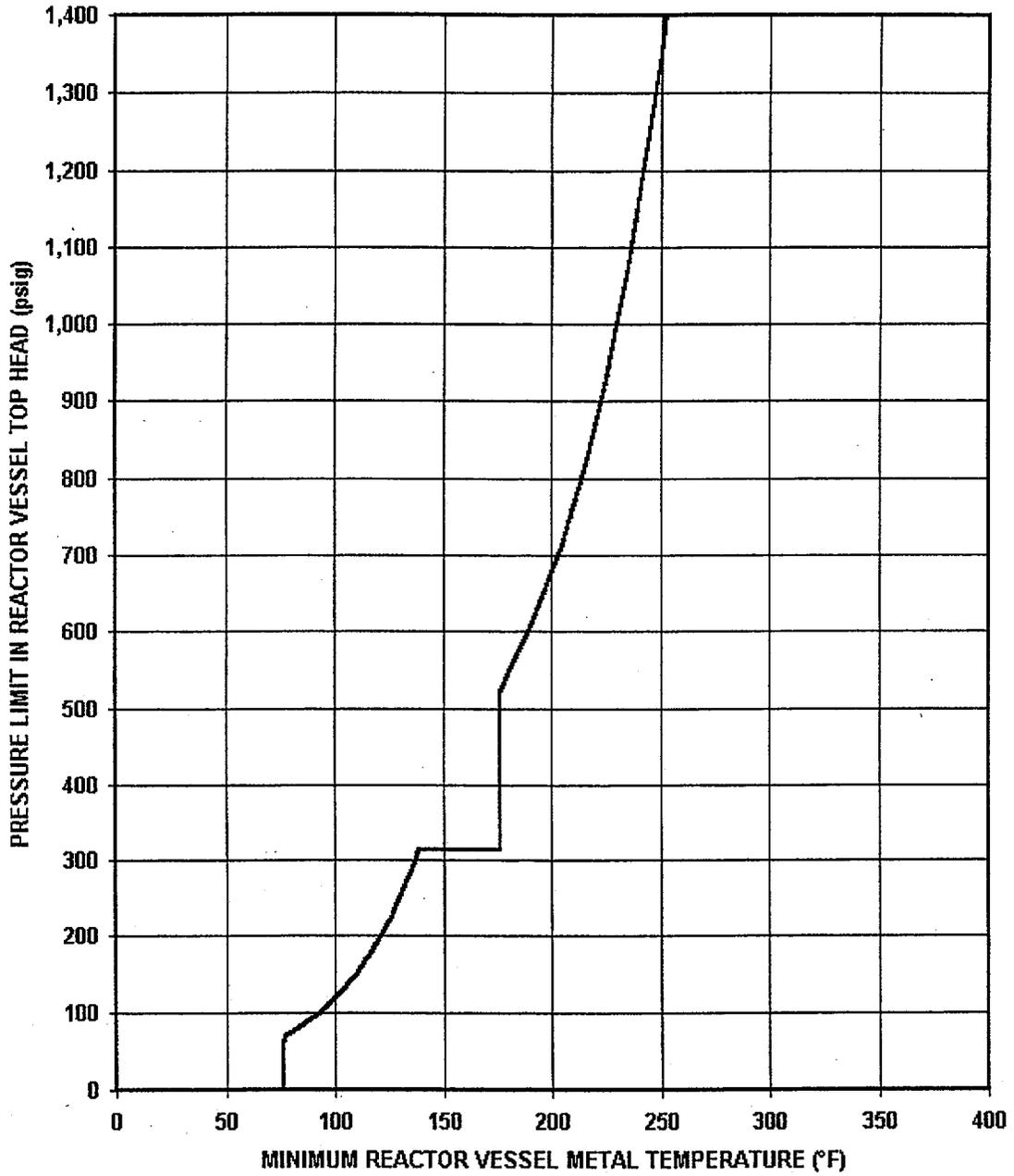
Unit 1 Core Critical Curve (Curve C), 32 EFPY
