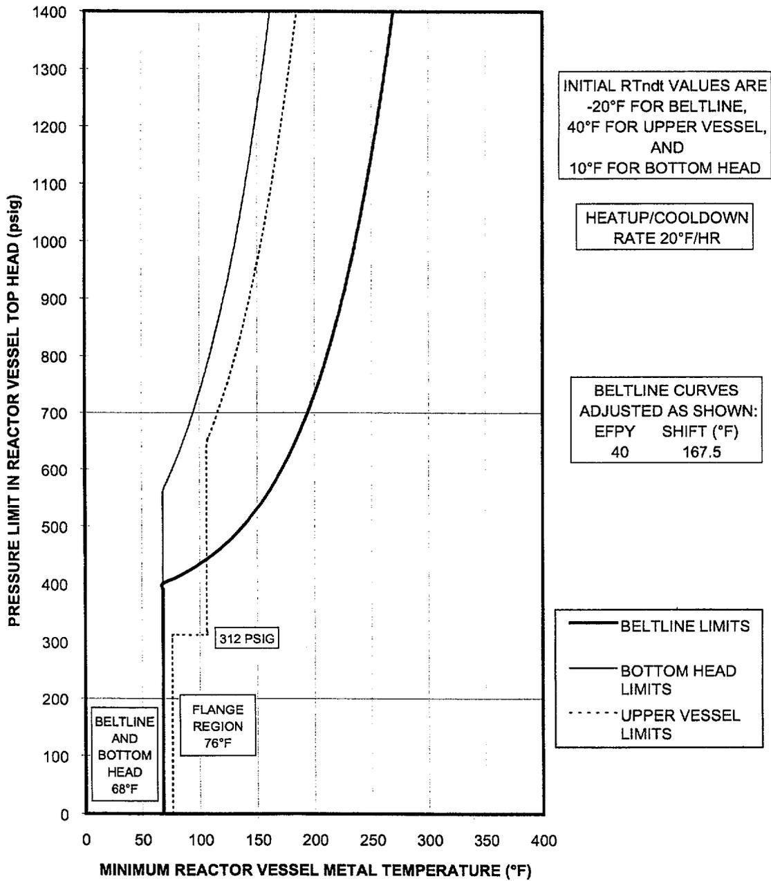
Figure B-1: P-T Curve for Unit 1 (Curve A)
