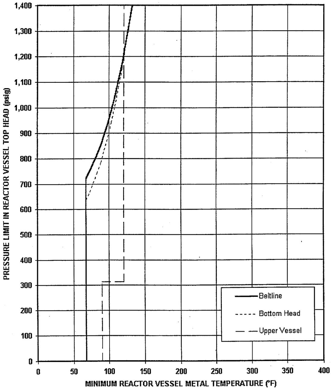
**Unit 2 Pressure Test Curve (Curve A), 54 EFPY**
