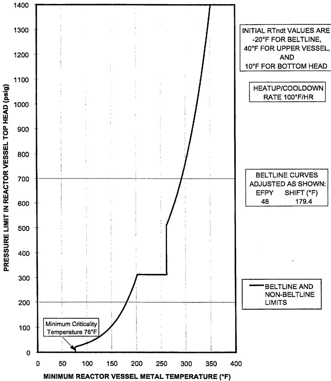
Figure D-3: P-T Curve for Unit 1 (Curve C)
