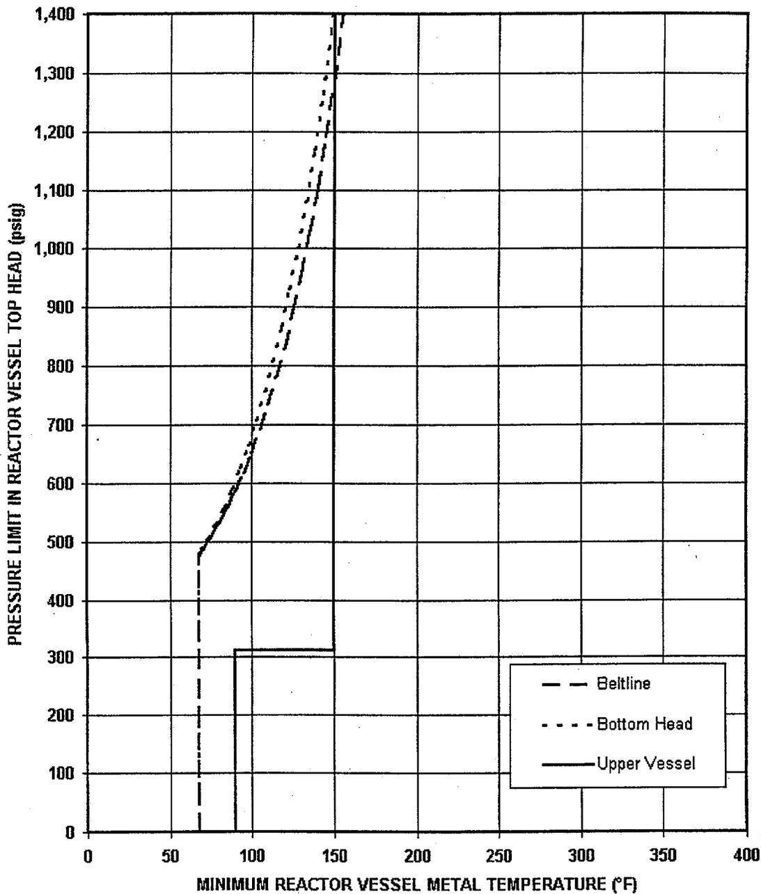
**Unit 2 Core Not Critical Curve (Curve B), 54 EFPY**
