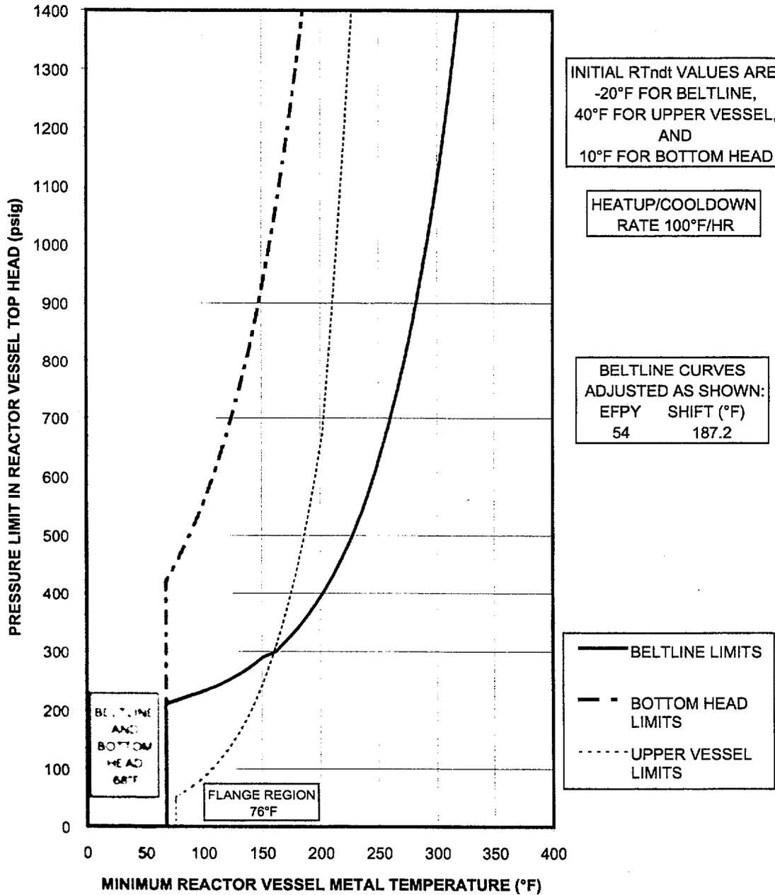
Figure 4-2: Non-Nuclear Heatup/Cooldown (Curve B) [Unit 1]
