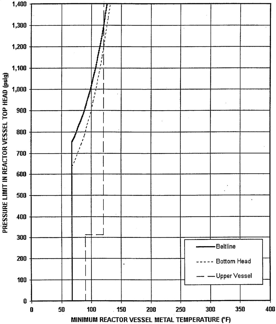
**Unit 2 Pressure Test Curve (Curve A), 32 EFPY**
