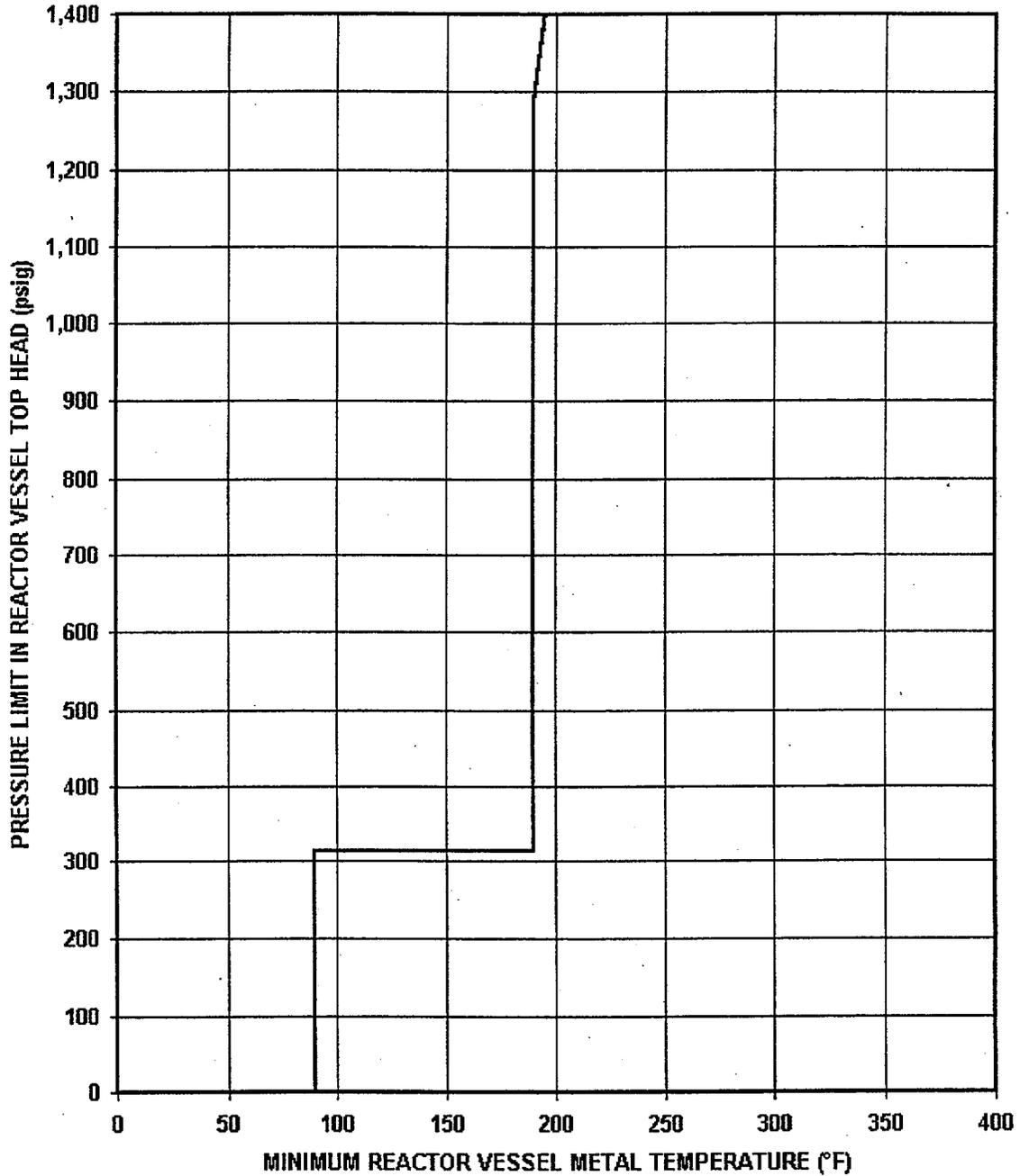
Unit 2 Core Critical Curve (Curve C), 54 EFPY
