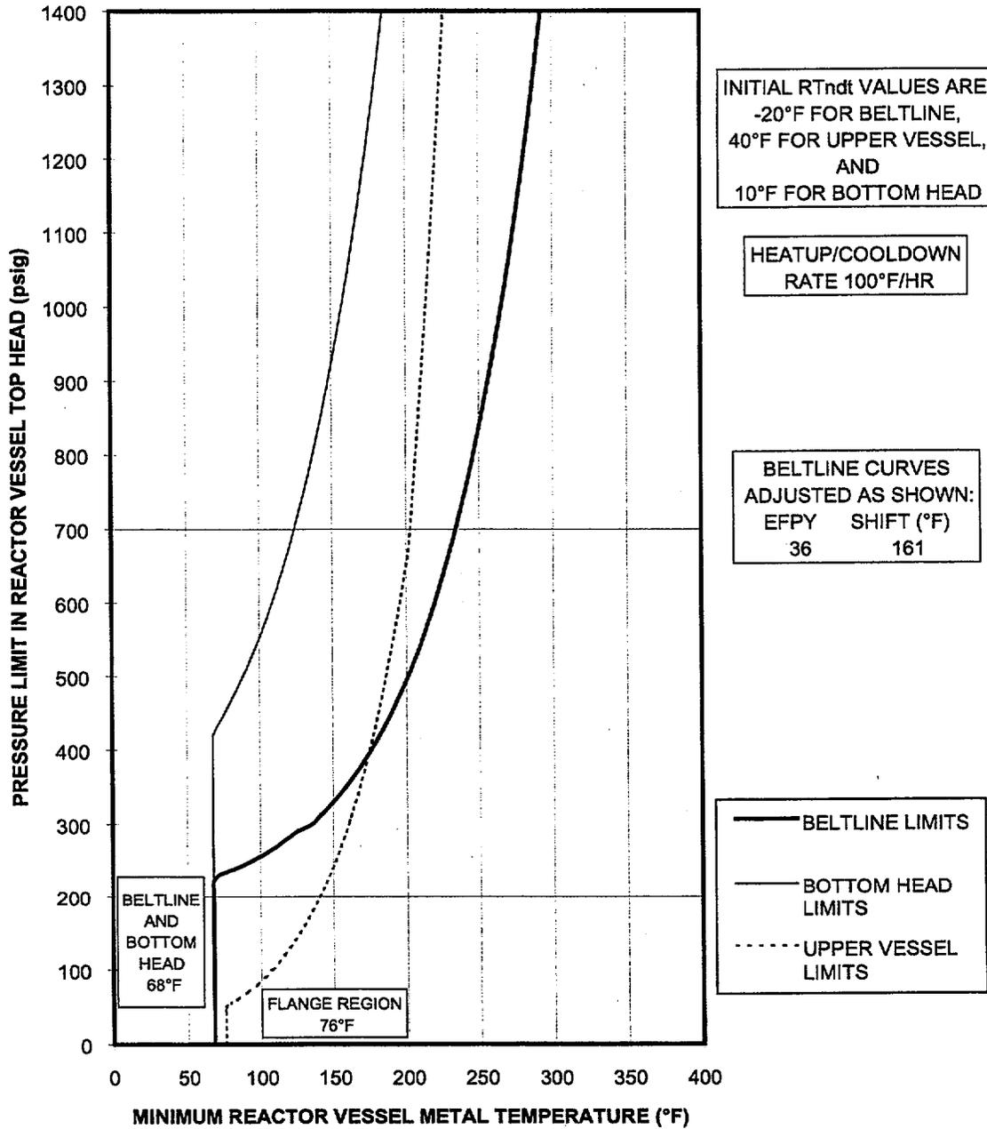
Figure A-2: P-T Curve for Unit 1 (Curve B)
