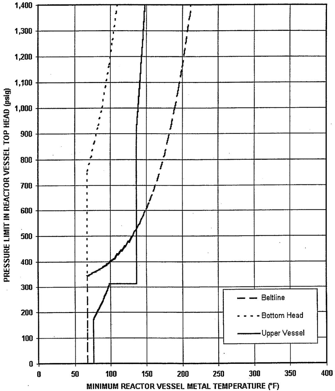
**Unit 1 Core Not Critical Curve (Curve B), 32 EFY**
