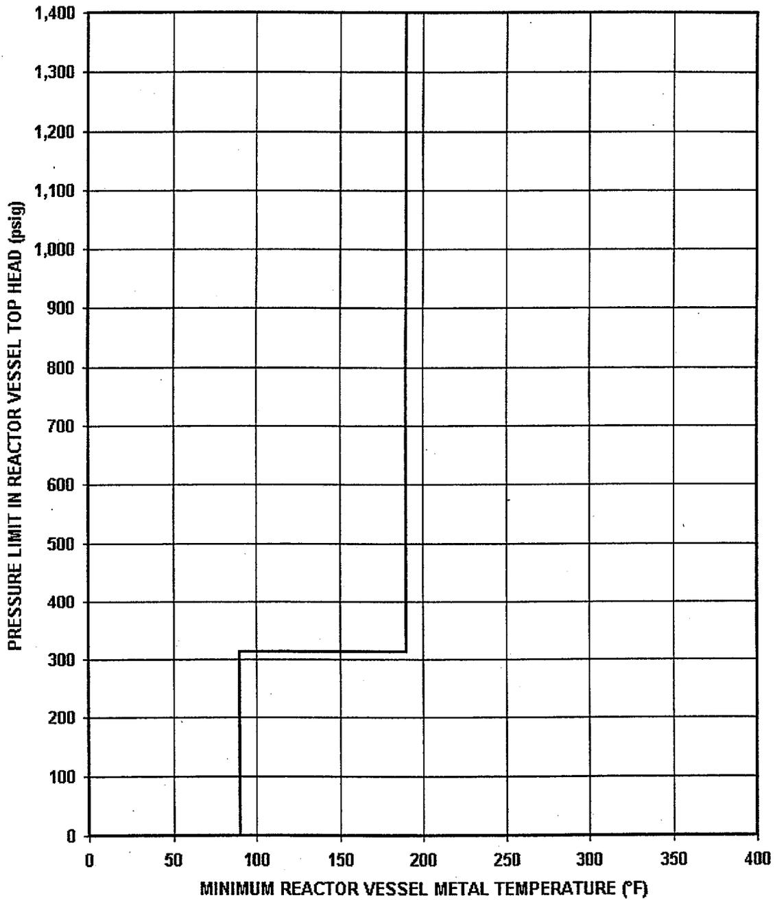
**Unit 2 Core Critical Curve (Curve C), 20 EFPY**
