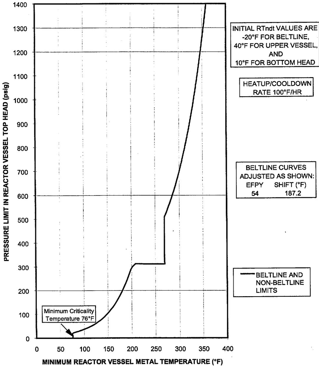
Figure 4-3: Core Critical Curve (Curve C) [Unit 1]
