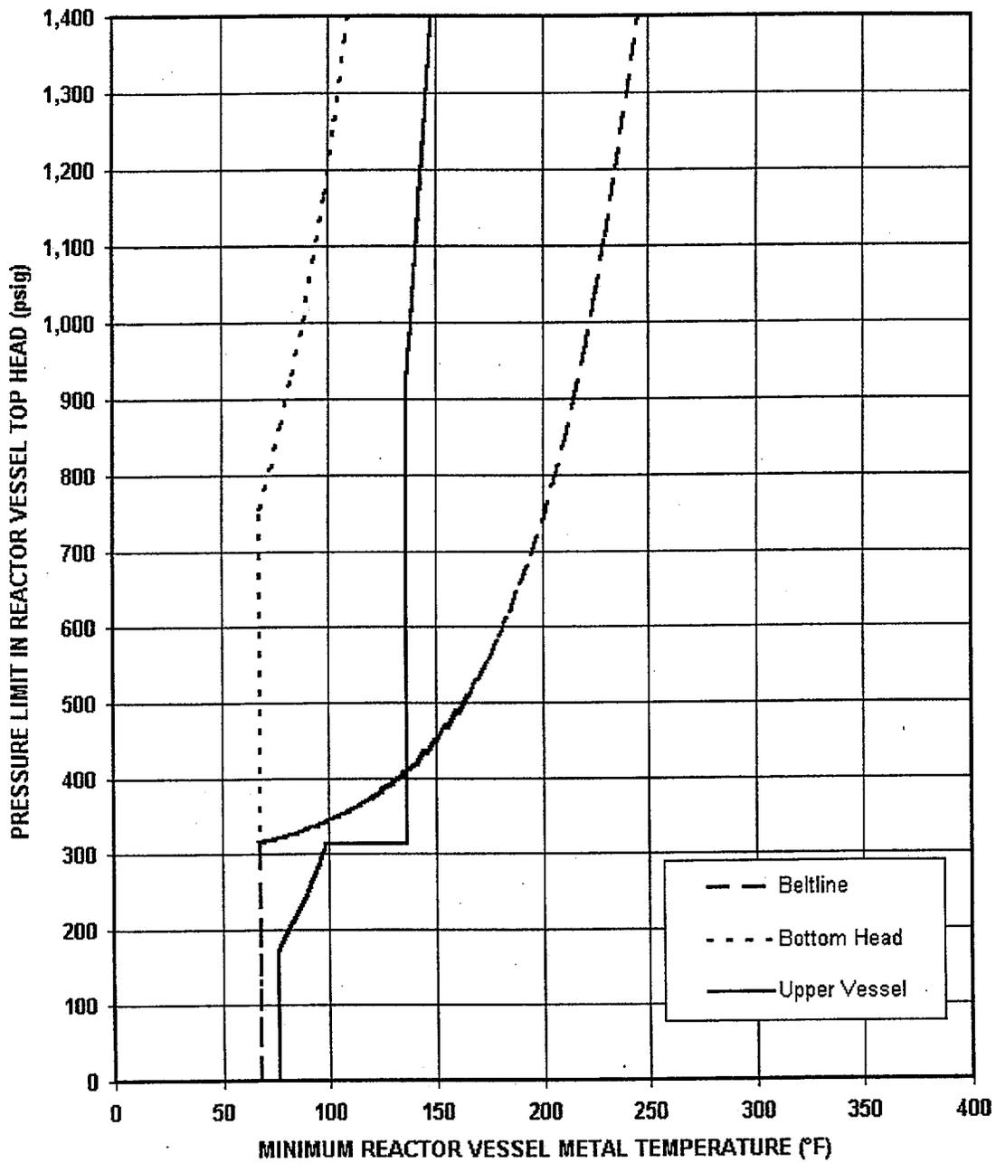
**Unit 1 Core Not Critical Curve (Curve B), 54 EFPY**
