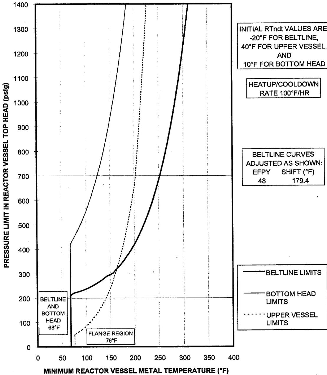
Figure D-2: P-T Curve for Unit 1 (Curve B)
