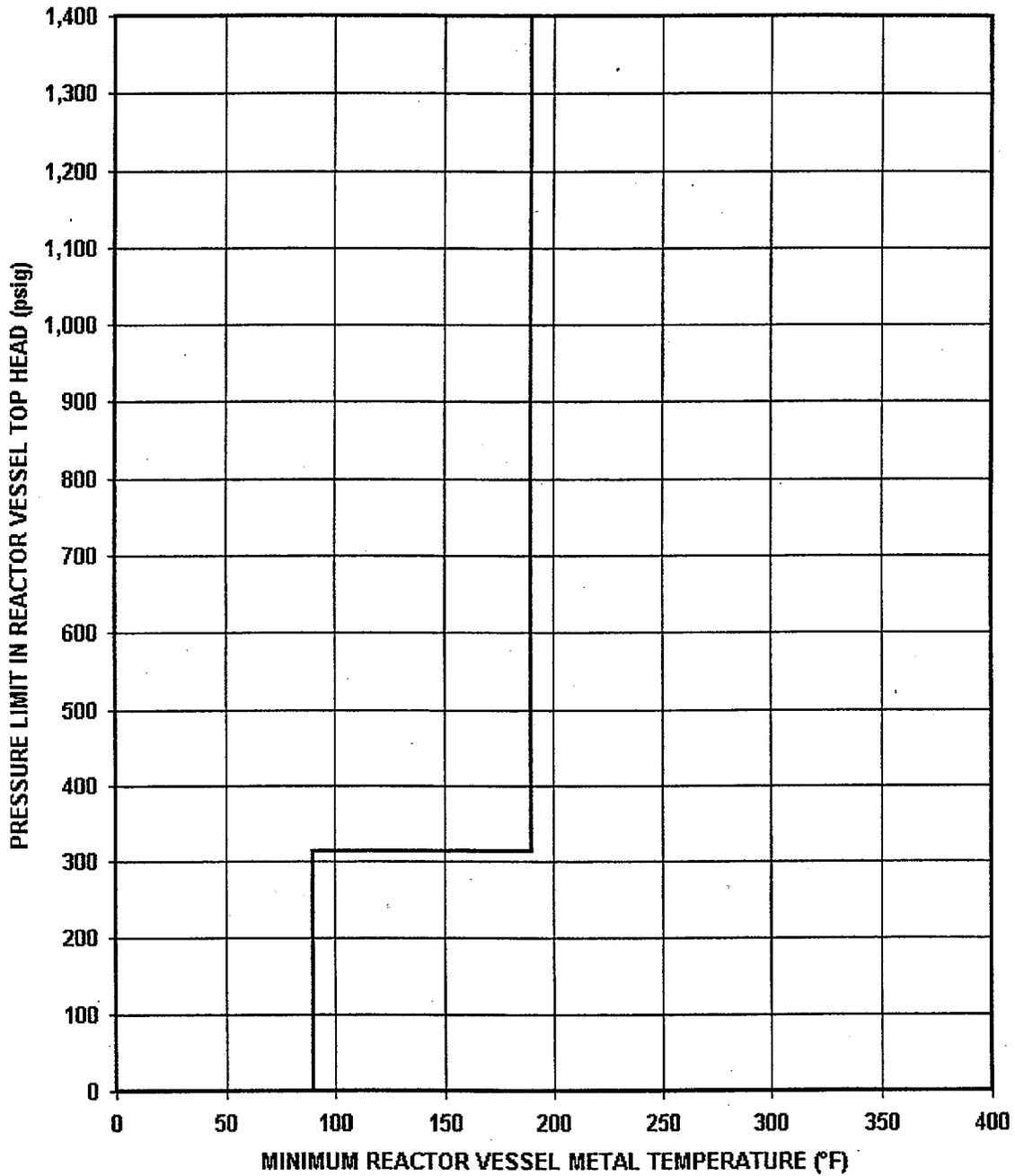
Unit 2 Core Critical Curve (Curve C), 32 EPY
