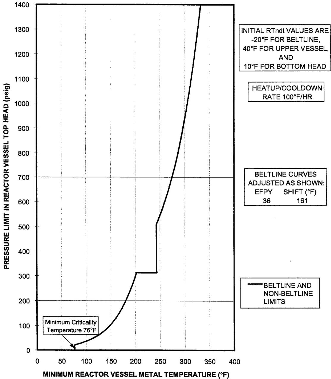
Figure A-3: P-T Curve for Unit 1 (Curve C)
