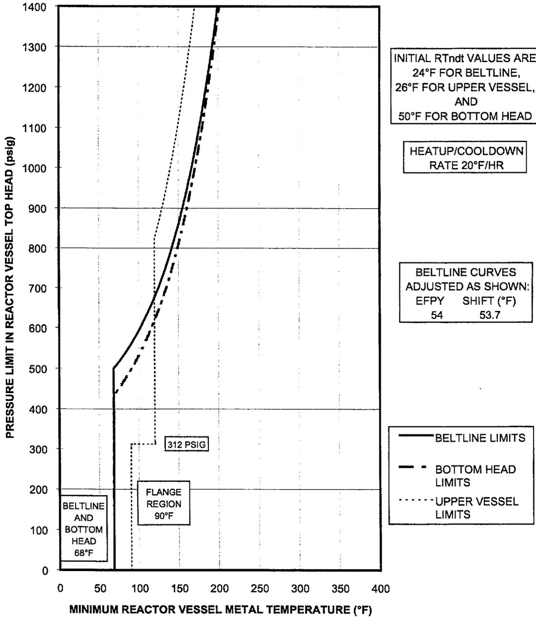
Figure 4-4: Pressure Test Curve (Curve A) [Unit 2]
