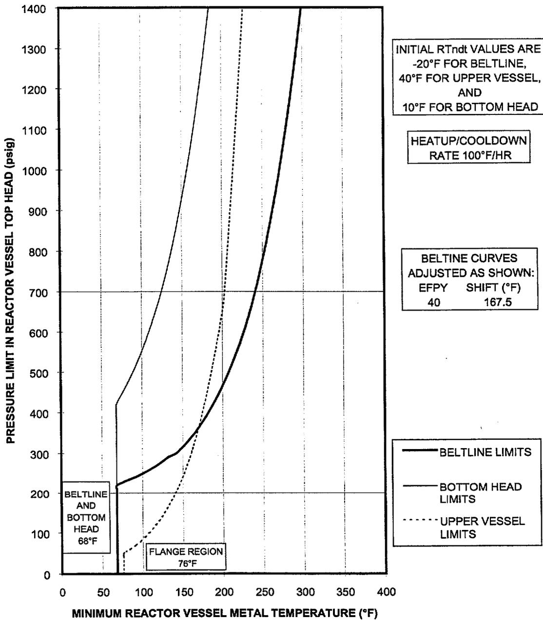
Figure B-2: P-T Curve for Unit 1 (Curve B)
