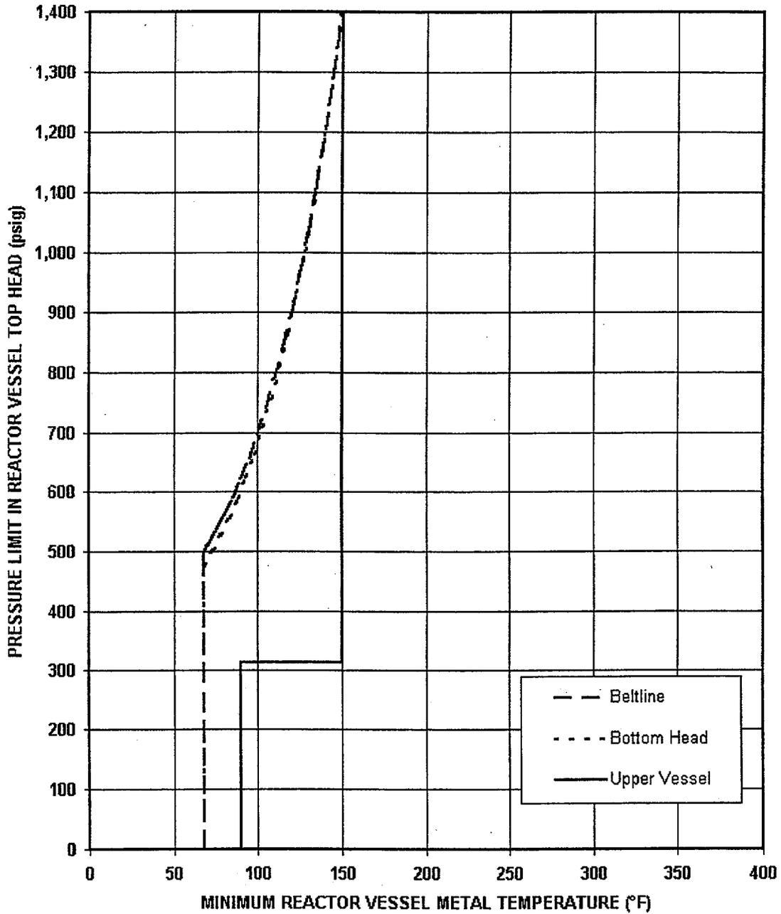
**Unit 2 Core Not Critical Curve (Curve B), 32 EFPY**
