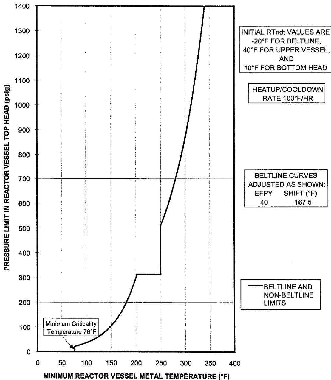
Figure B-3: P-T Curve for Unit 1 (Curve C)
