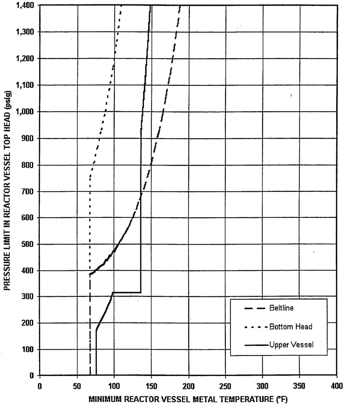
**Unit 1 Core Not Critical Curve (Curve B), 20 EFPY**
