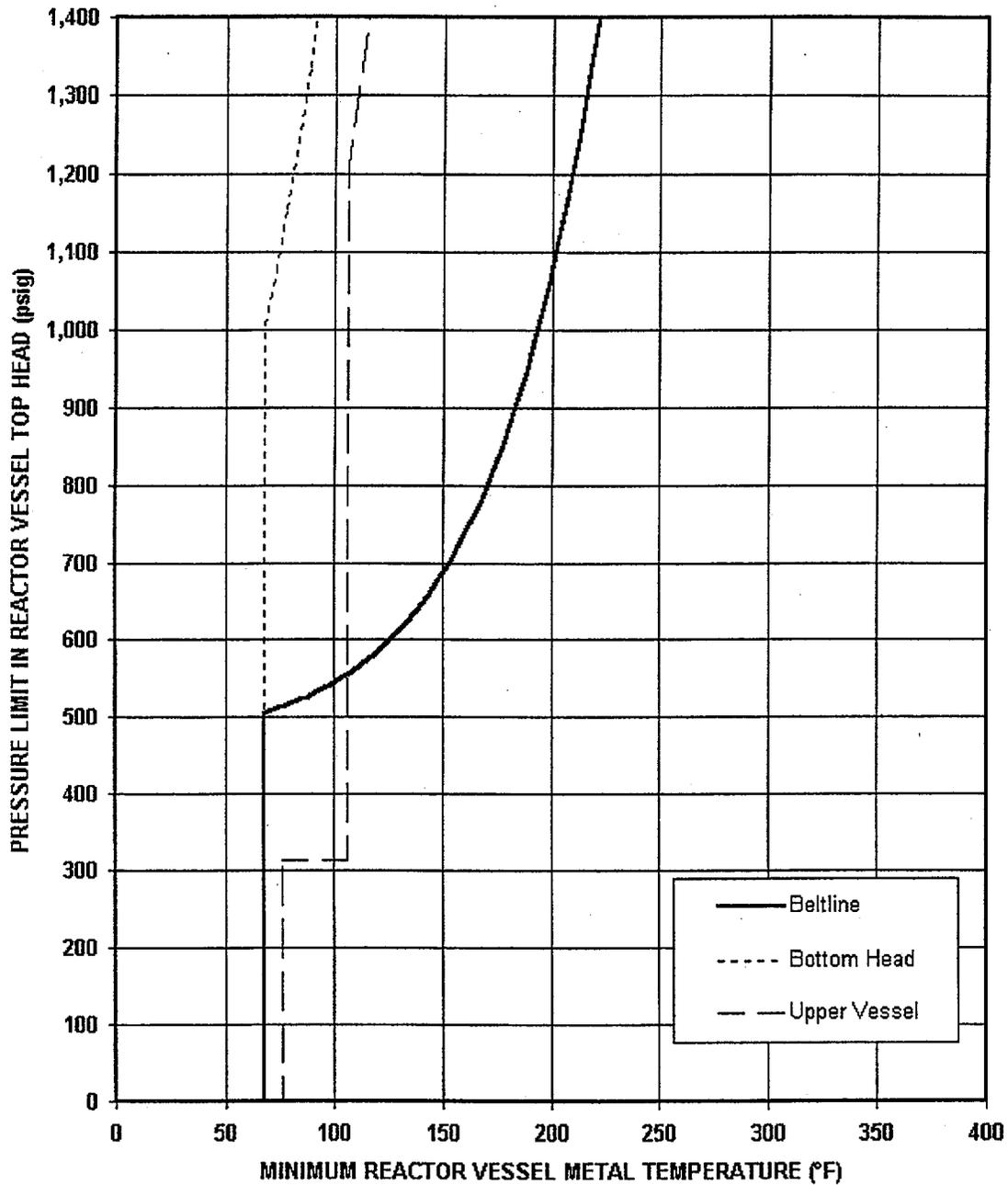
**Unit 1 Pressure Test Curve (Curve A), 54 EFPY**
