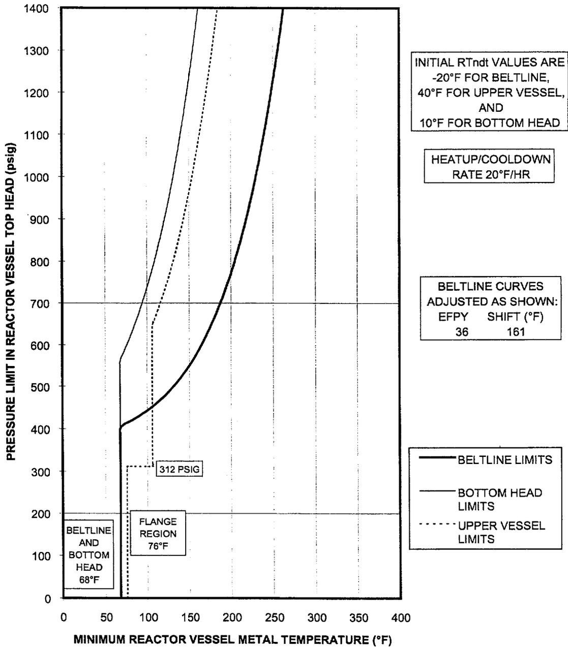
Figure A-1: P-T Curve for Unit 1 (Curve A)
