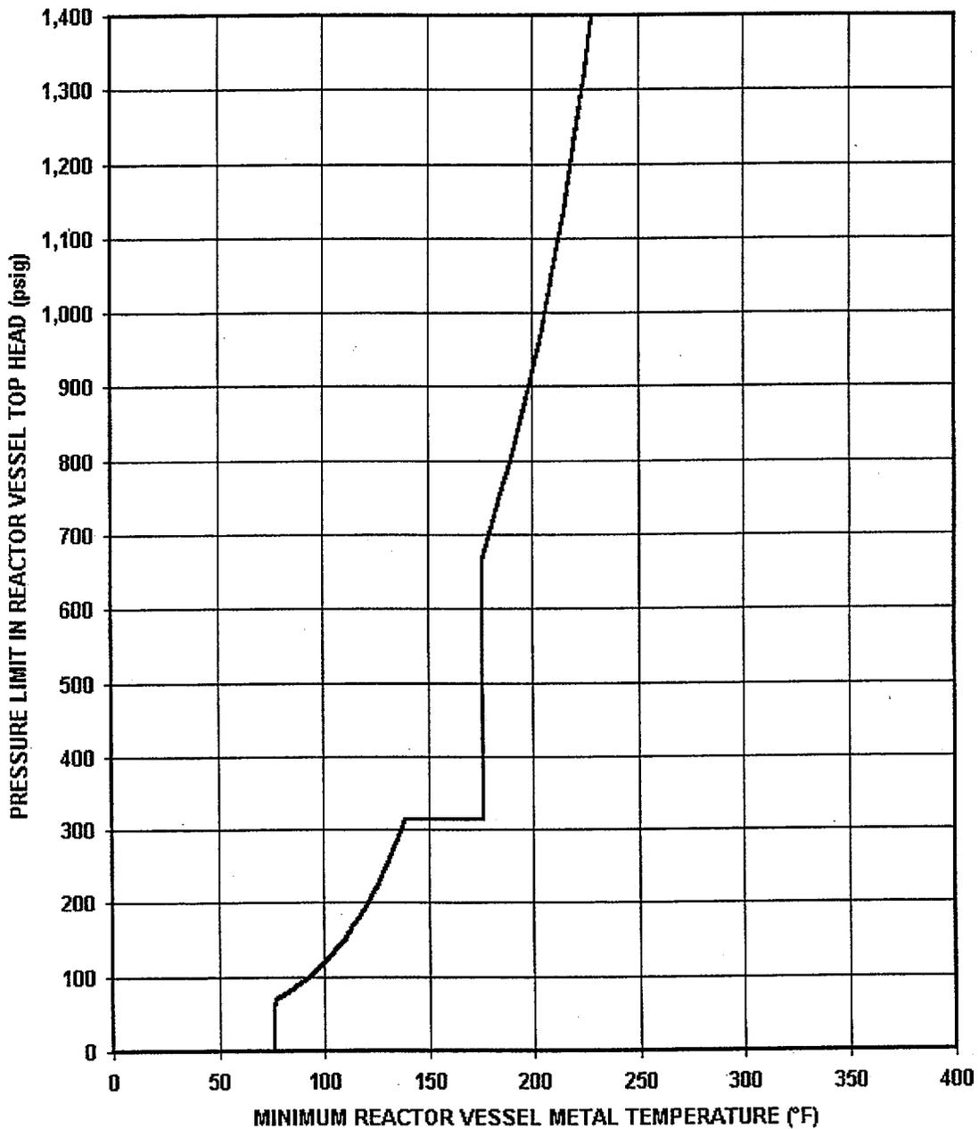
Unit 1 Core Critical Curve (Curve C), 20 EFPY
