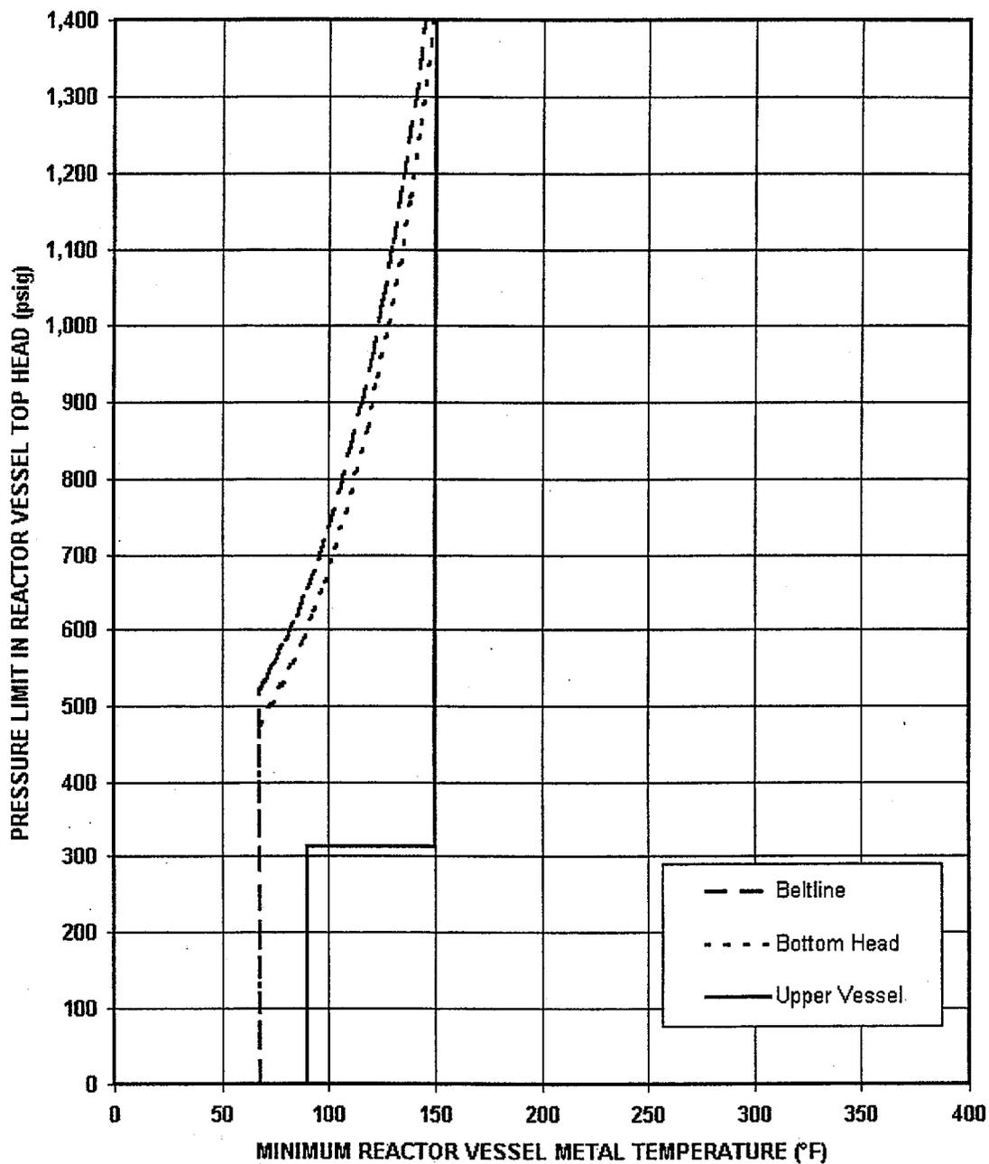
**Unit 2 Core Not Critical Curve (Curve B), 20 EFPY**
