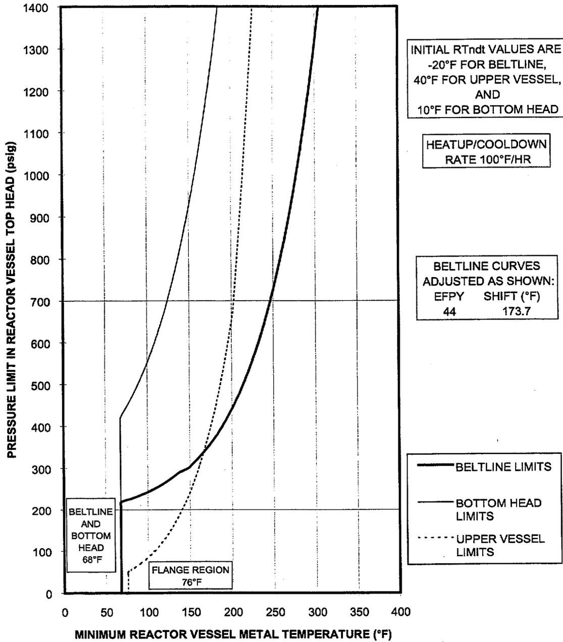
Figure C-2: P-T Curve for Unit 1 (Curve B)
