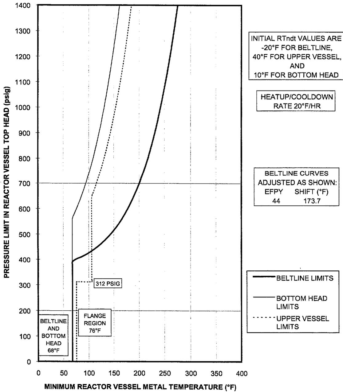
Figure C-1: P-T Curve for Unit 1 (Curve A)
