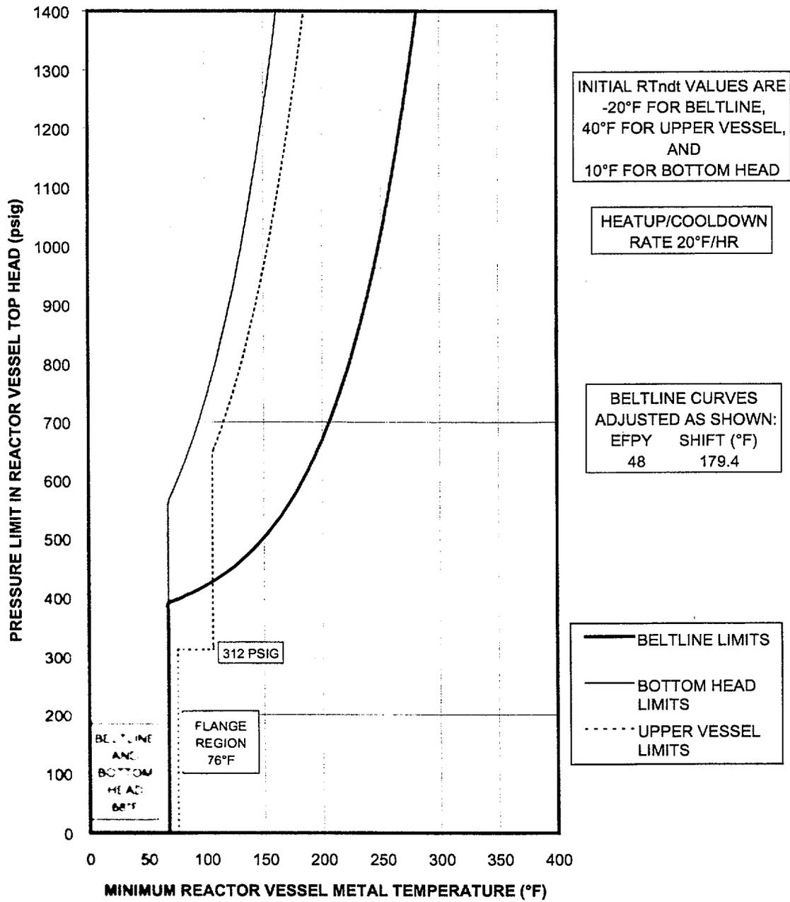
Figure D-1: P-T Curve for Unit 1 (Curve A)
