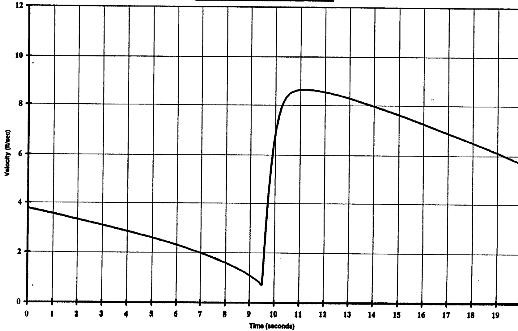
Figure A4-2 Case 4 : Pre P/P Startup - Velocity of Water in The Return Line - RBCU XAA-1B H.T. =85%, Fouling Factor =0.001
