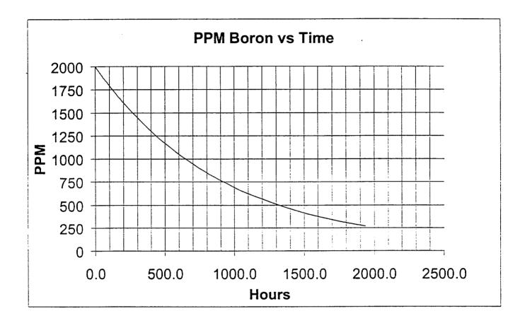
Figure 2: Boron Dilution with 5 gpm Non-Borated Water
