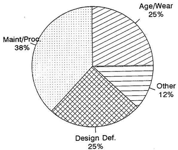
**BWR RCIC SYSTEM TDP FAILURE CAUSES
