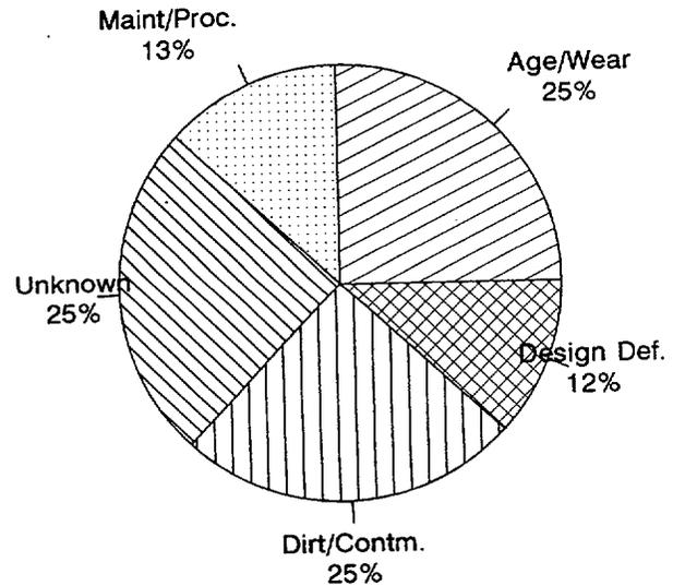
PWR AFW SYSTEM TDP FAILURE CAUSES
