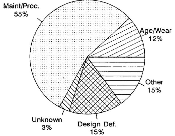
**BWR HPCI SYSTEM TDP FAILURE CAUSES
