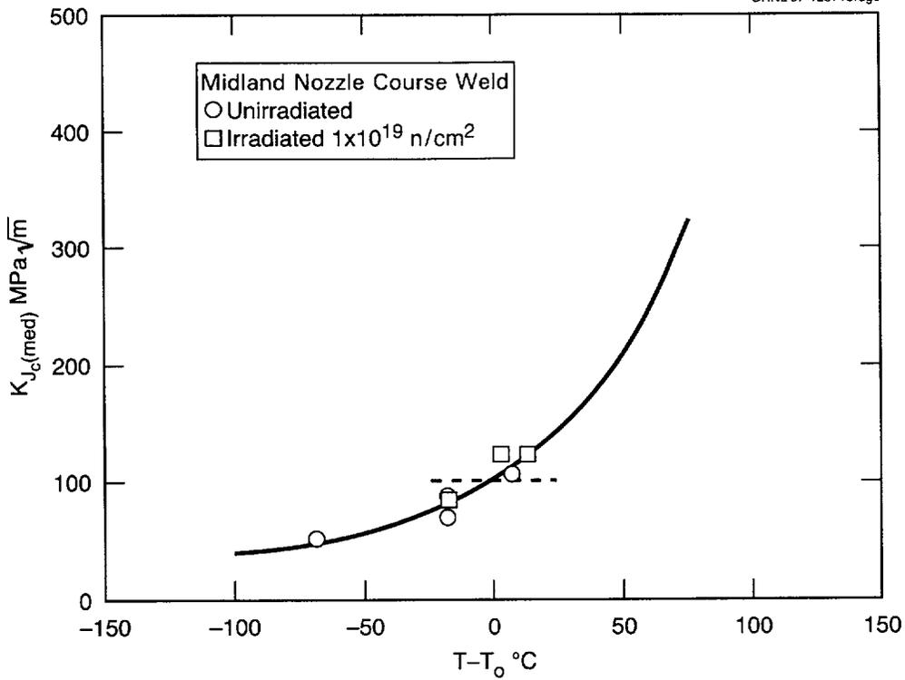
Figure 2.3. Median fracture toughness plotted against the master curve for WF-70 nozzle course weld metal.
