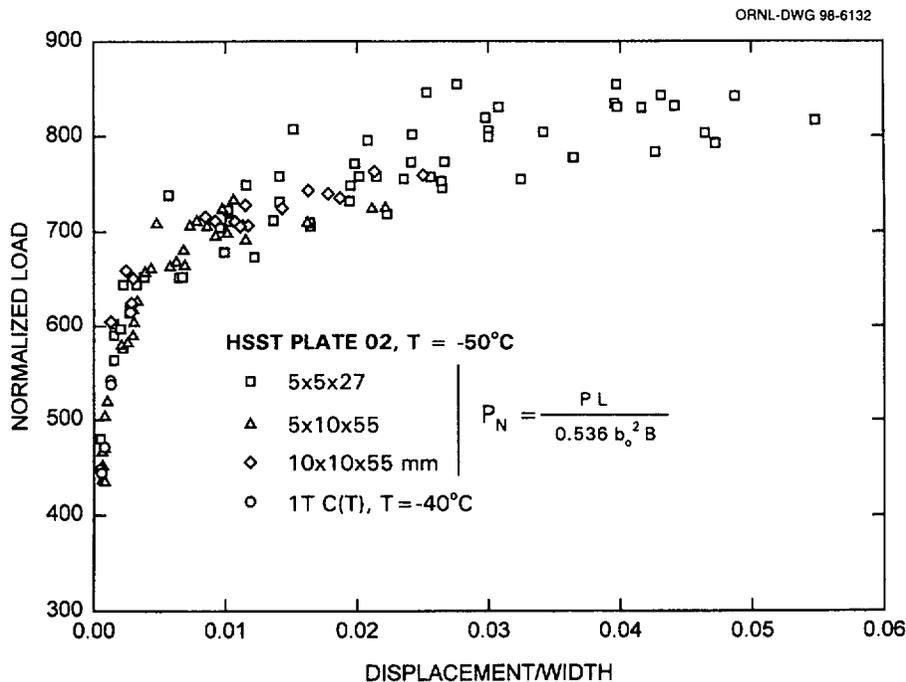
Figure 6.1. Key curves of different specimen types.
