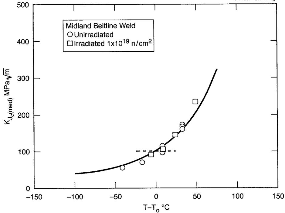
Figure 2.2. Median fracture toughness plotted against the master curve for WF-70 beltline weld metal.
