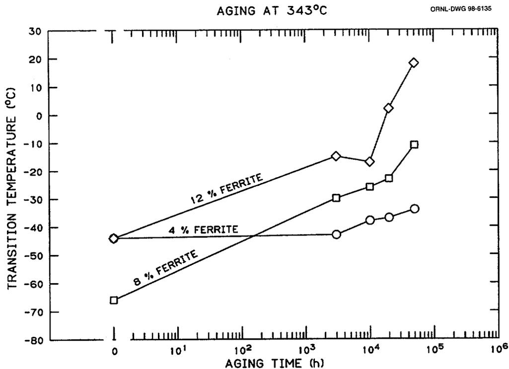
**Figure 7.2.** Effect of aging at 343°C on the ductile-to-brittle transition temperature for type 308 stainless steel welds. The transition temperature increases with increased aging time, and the effect is greater for welds with higher ferrite contents.
