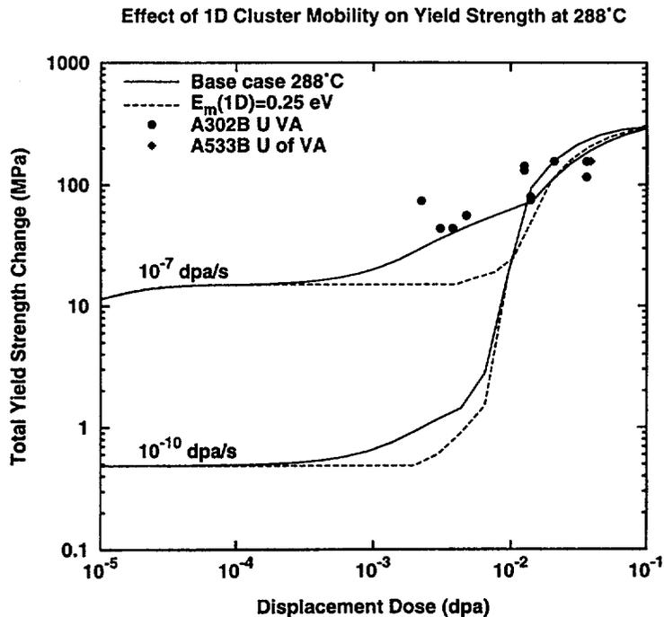
**Figure 4.3. Comparison of calculated yield-strength changes in experimental data for 288°C irradiation at indicated displacement rates; one-dimensional interstitial cluster migration energy is 0.25 eV.**
