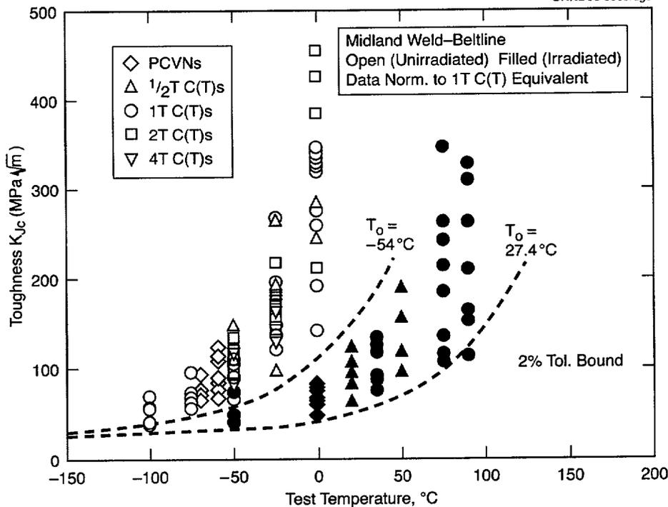
**Figure 2.5.** All nozzle course weld metal data as normalized to 1T specimens size equivalence; 2% tolerance bound curves.
