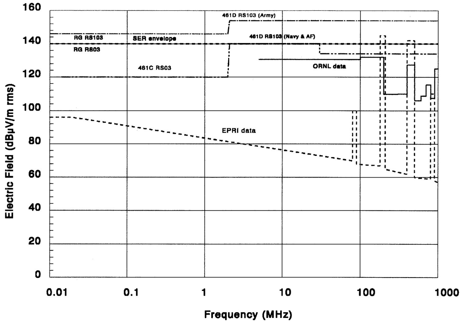
Figure A.4 Comparison of high-frequency radiated susceptibility envelopes
