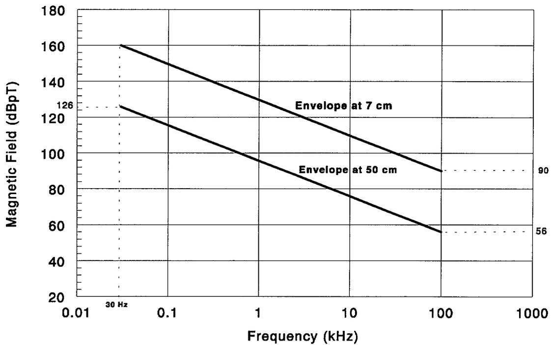
Figure 4.6 RE101 Magnetic Field Emissions Envelopes
