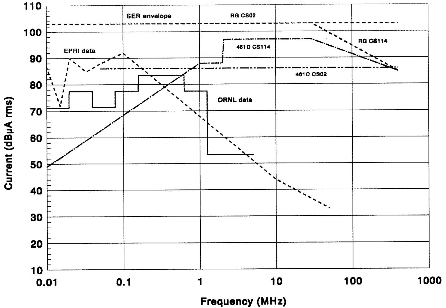
Figure A.2 Comparison of high-frequency conducted susceptibility envelopes
