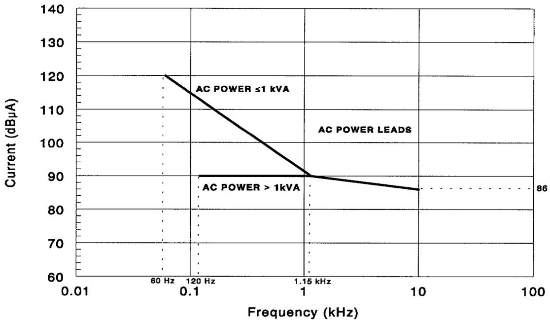
Figure 4.2 CE101 Emissions Envelopes for ac Power Leads
