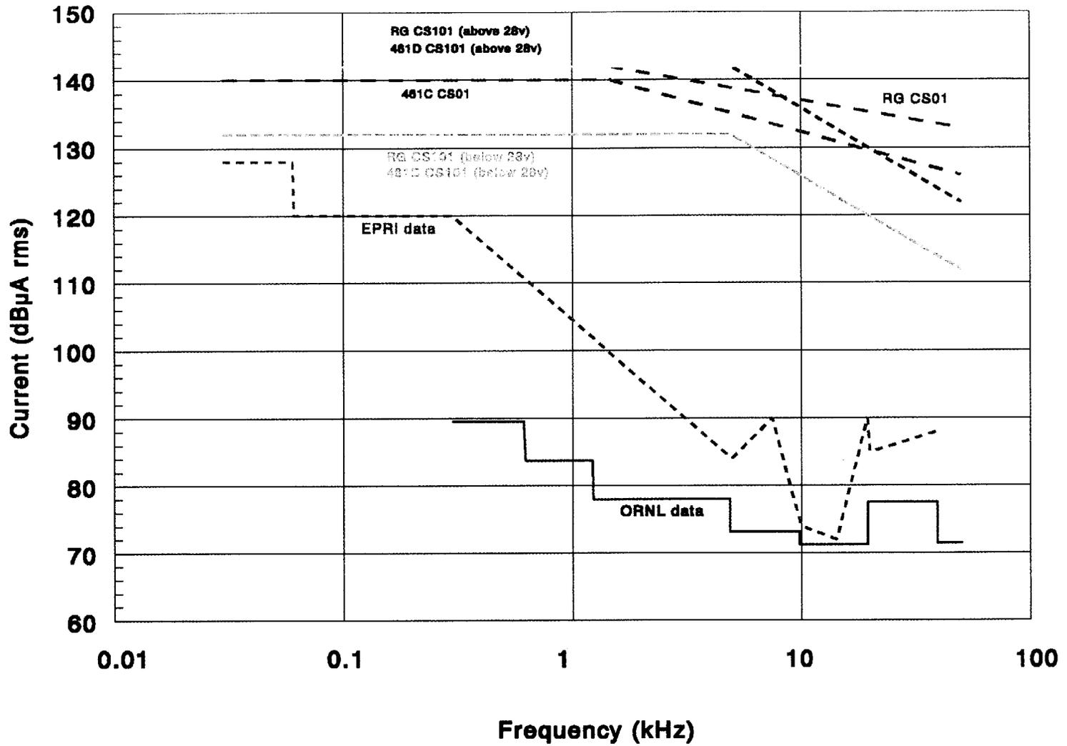
Figure A.1 Comparison of low-frequency conducted susceptibility envelopes
