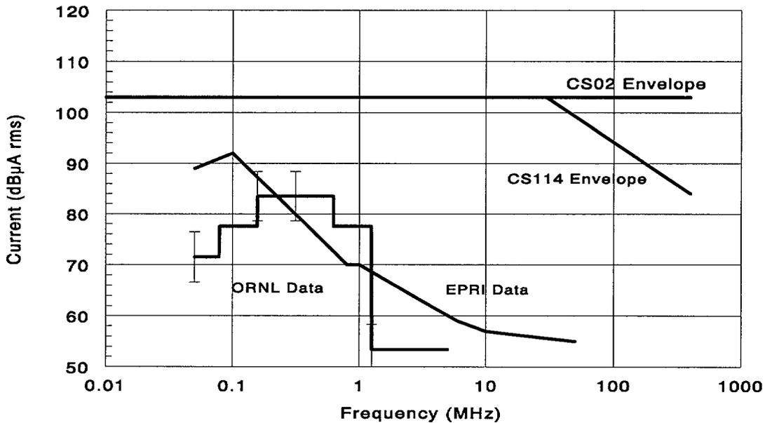
Figure 6.4 Data vs Operating Envelopes, Conducted Interference - 10 kHz to 400 MHz
