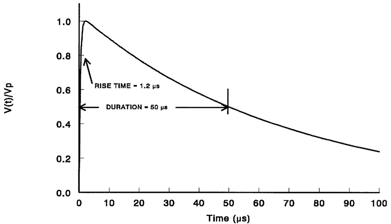
Figure 5.2 Combination Wave, Open-circuit Voltage
