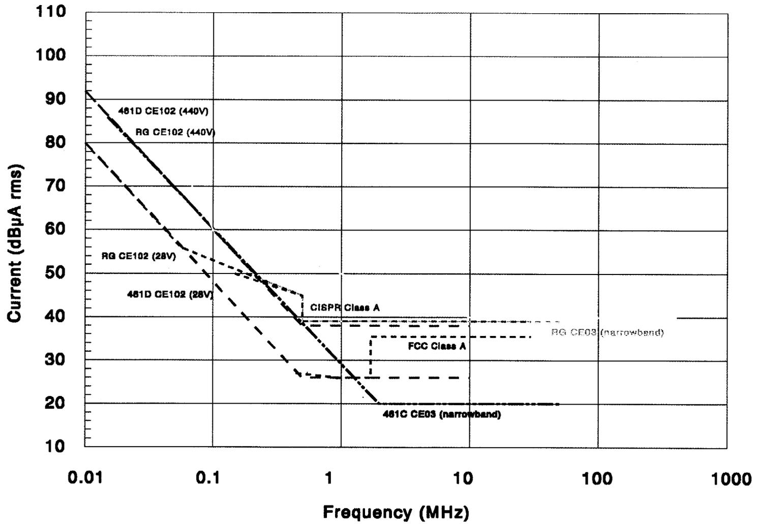
Figure A.6 Comparison of high-frequency conducted emissions envelopes
