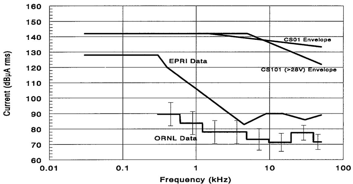
Figure 6.3 Data vs Operating Envelopes, Conducted Interference - 30 Hz to 50 kHz
