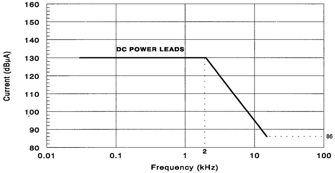
Figure 4.9 CE01 Emissions Envelope for dc Power Leads
