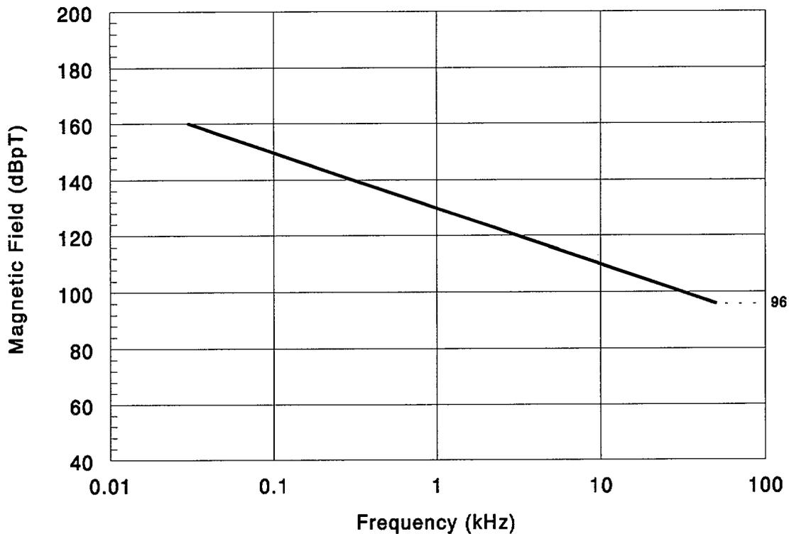
**Figure 4.13 RE01 Magnetic Field Emissions Envelope**
