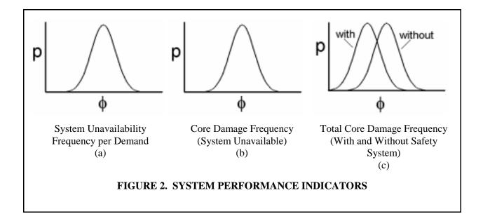
Figure 2c is a key result in the quantification of the defense-in-depth of safety system protection. It is the total core damage frequency with and without the specific safety system being analyzed. It is important to note that Figure 2c is a different CDF than the one on which Figure 2b is based. The Figure 2b CDFs are those of Column 6. The Figure 2c CDF is the probabilistic sum of the Column 6 CDFs.
