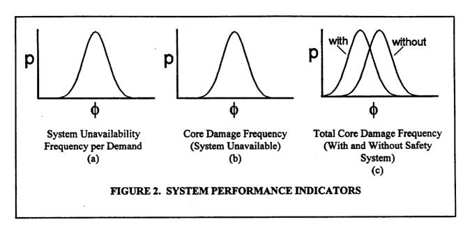
Figure 2c is a key result in the quantification of the defense-in-depth of safety system protection. It is the total core damage frequency with and without the specific safety system being analyzed. It is important to note that Figure 2c is a different CDF than the one on which Figure 2b is based. The Figure 2b CDFs are those of Column 6. The Figure 2c CDF is the probabilistic sum of the Column 6 CDFs.
