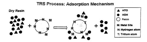
The metal sites saturate relative to the HTO in the feed. The adsorption material is regenerated by heating in hot air driving off all waters of hydration.
