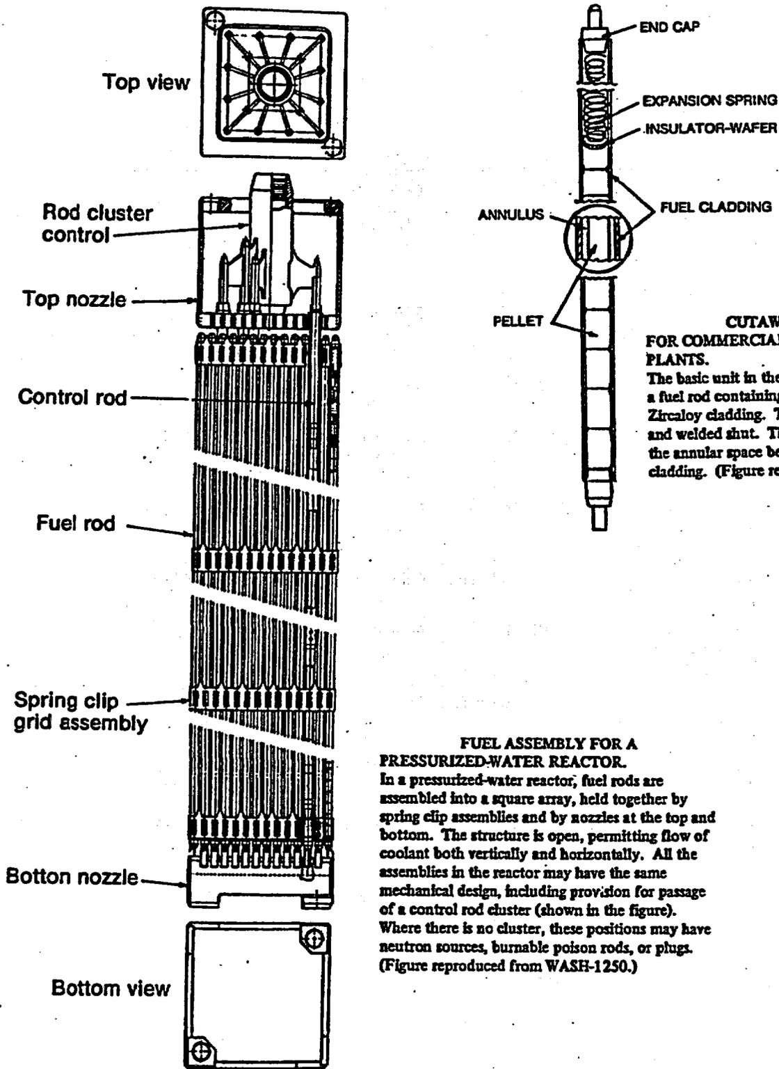
**FUEL ASSEMBLY FOR A PRESSURIZED-WATER REACTOR.**
